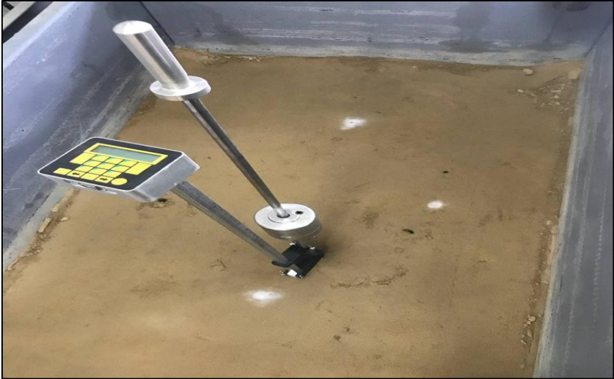
Figure (3.13) DCP in laboratory test setup
