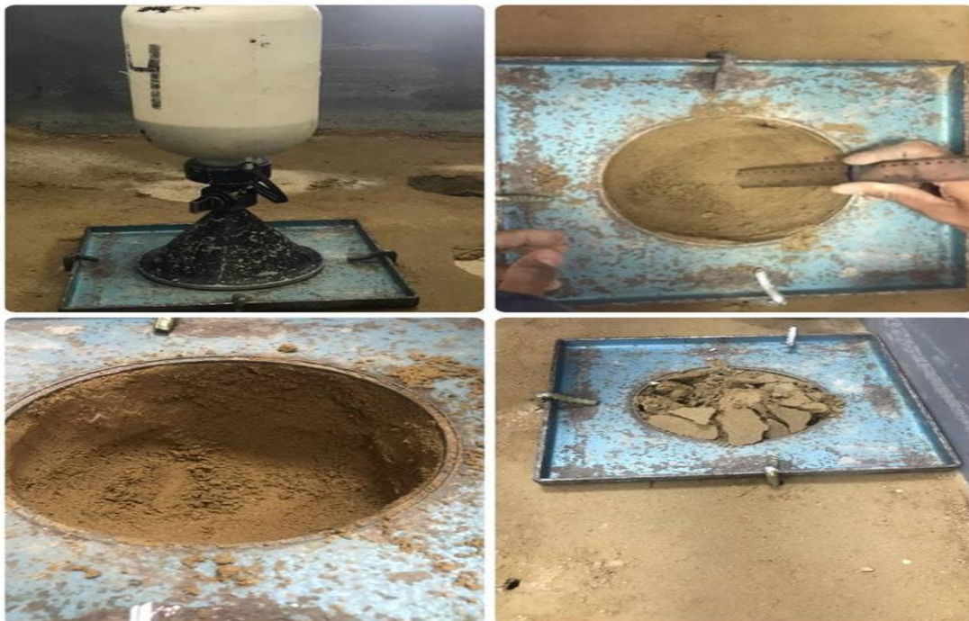
Figure (3.15) Sand replacement method test
