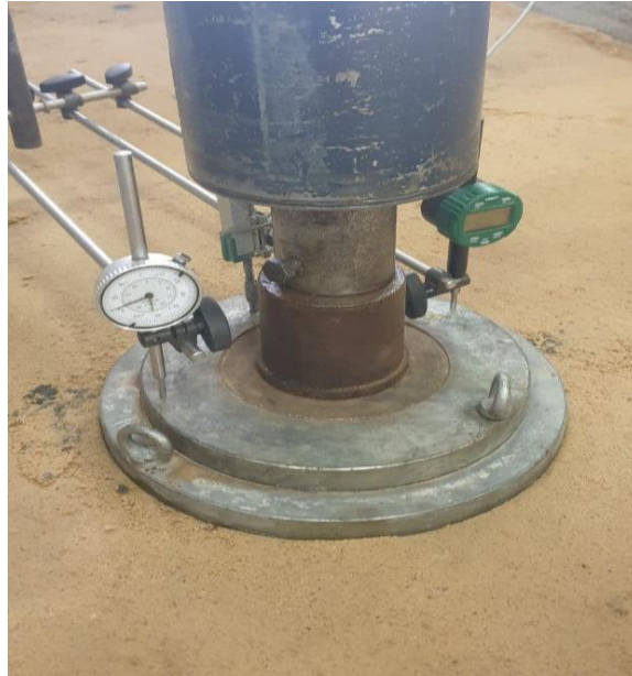
Figure (3.10) Plate load test
