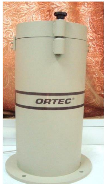
Figure (3-4): Photograph of the shielding chamber in NaI(Tl) detector [72].
