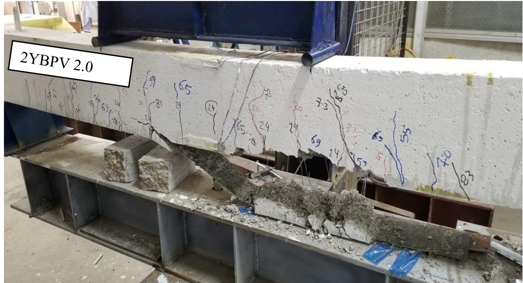
a) The failure of the beam by cover delamination
