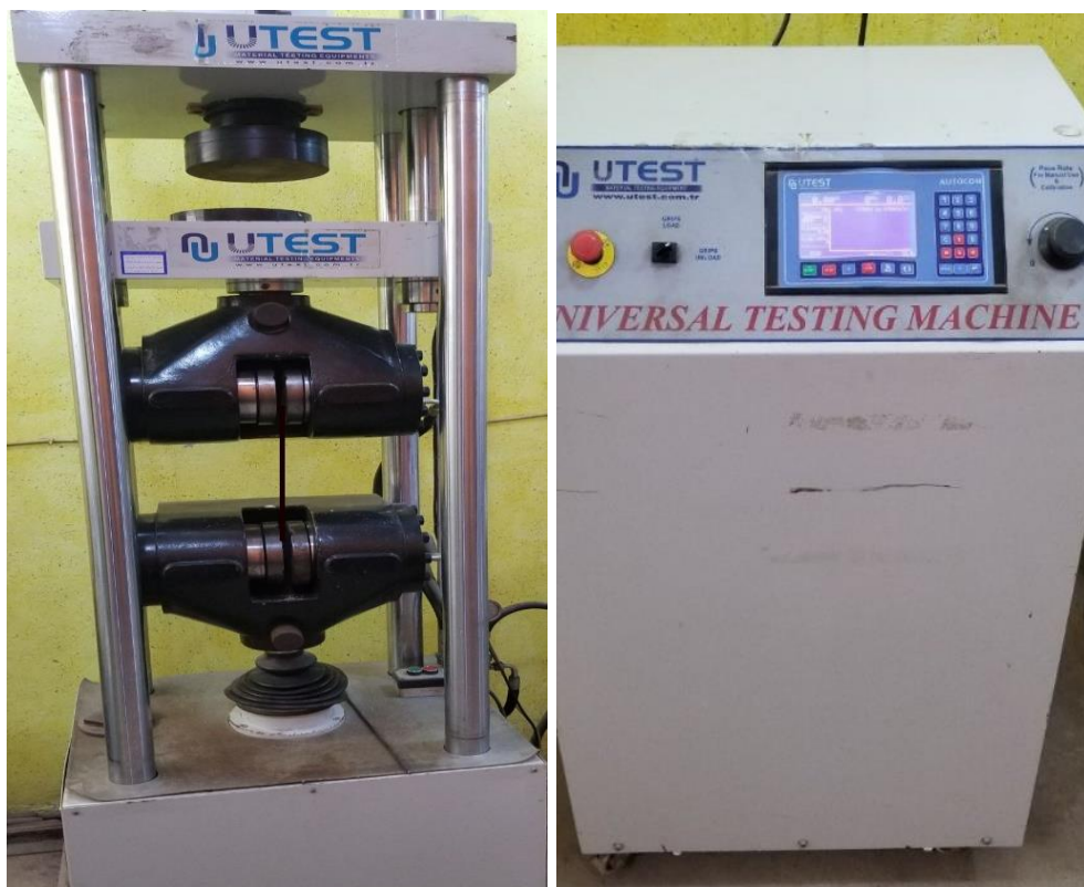
Figure 3-7: Steel reinforcement testing machine
