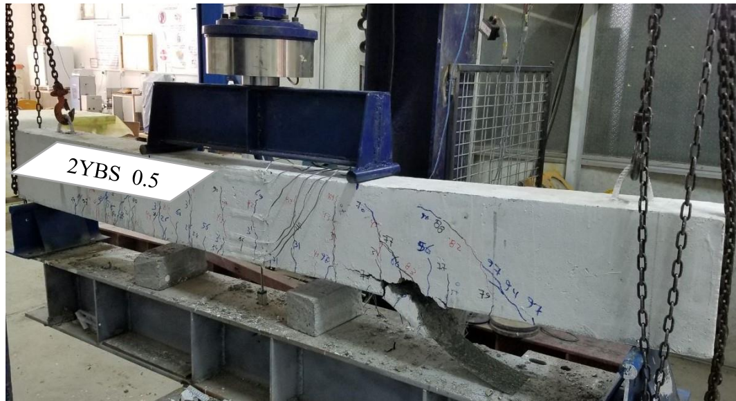
a) Failure of the beam 2YBS 0.5 by delamination problem
