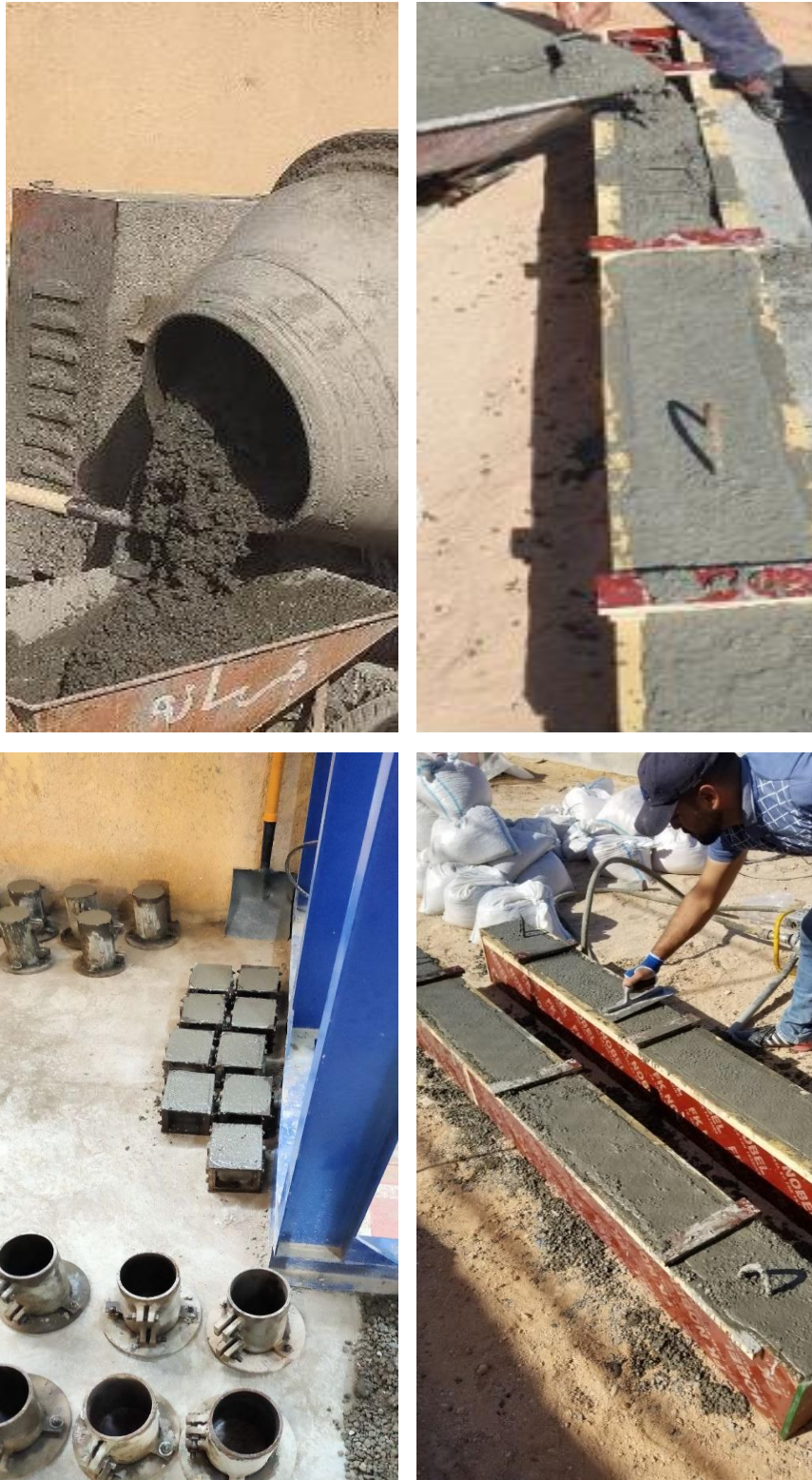
Figure 3-12: The first group where the model is casted in one batch from the mixer B.R.C.
