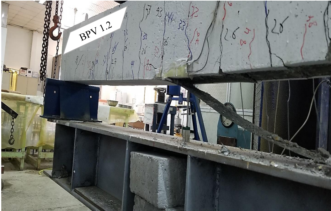
a) The failure of the beam BPV 1.2 by debonding problem
