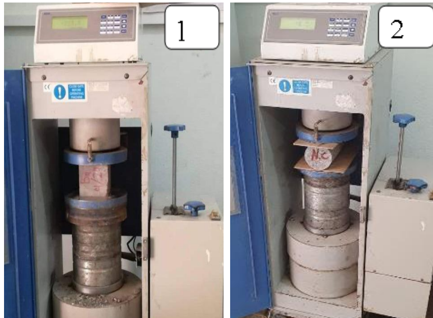
Figure 3-17: Compressive and Splitting Tensile Strengths: 1) Compressive Strength; 2) Splitting Tensile Strength.
