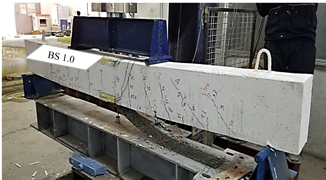
b) Failure of the beam BS 1.0 by debonding problem
