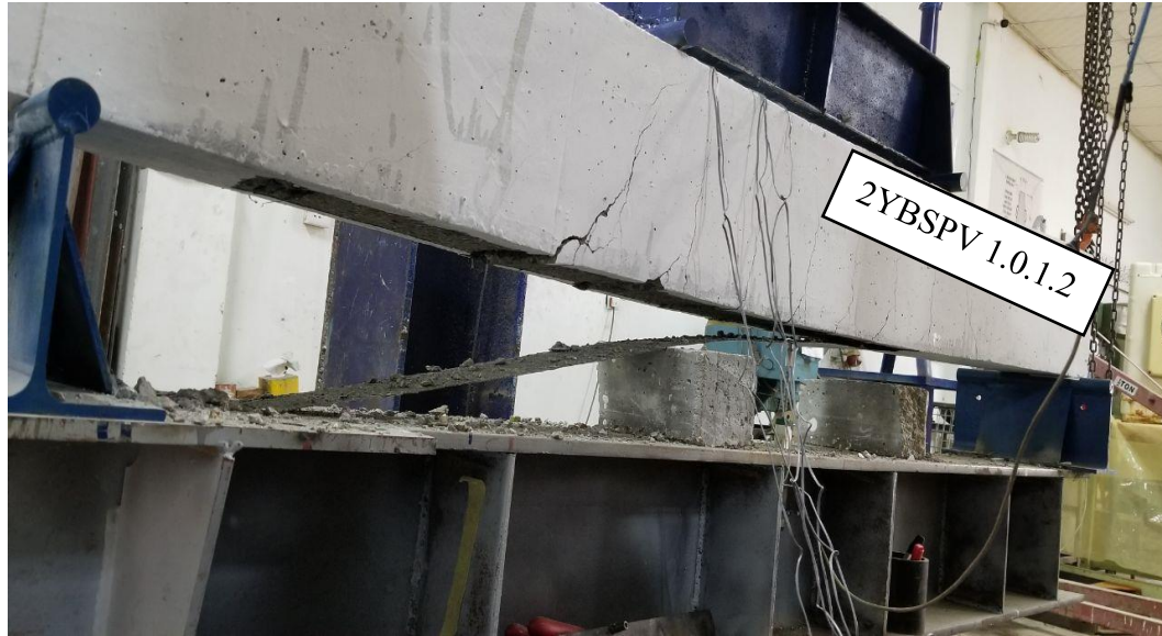
c) Failure of the beam 2YBSPV 1.0.1.2 by debonding problem
