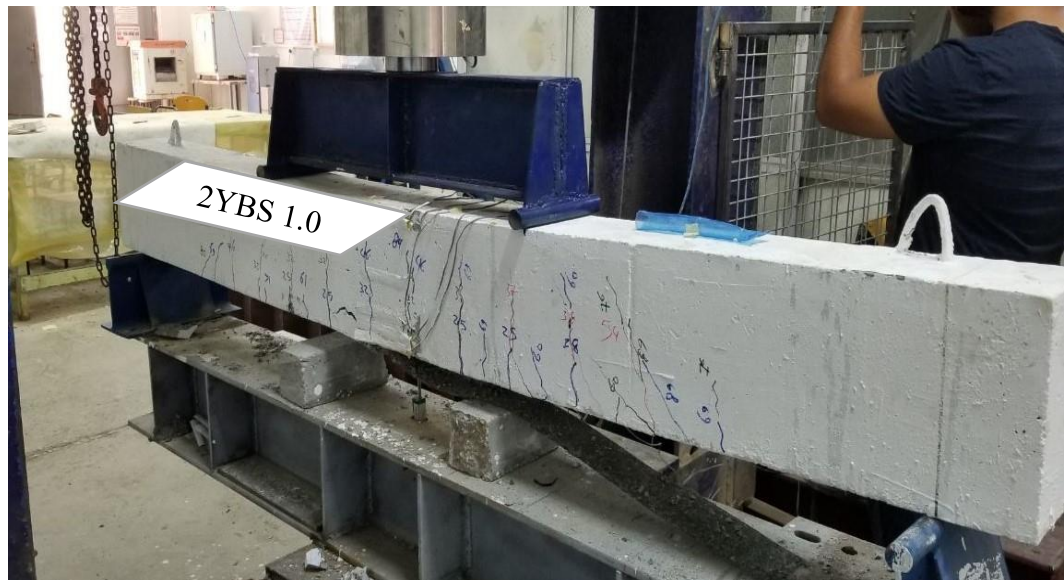
b) Failure of the beam 2YBS 1.0 by debonding problem
