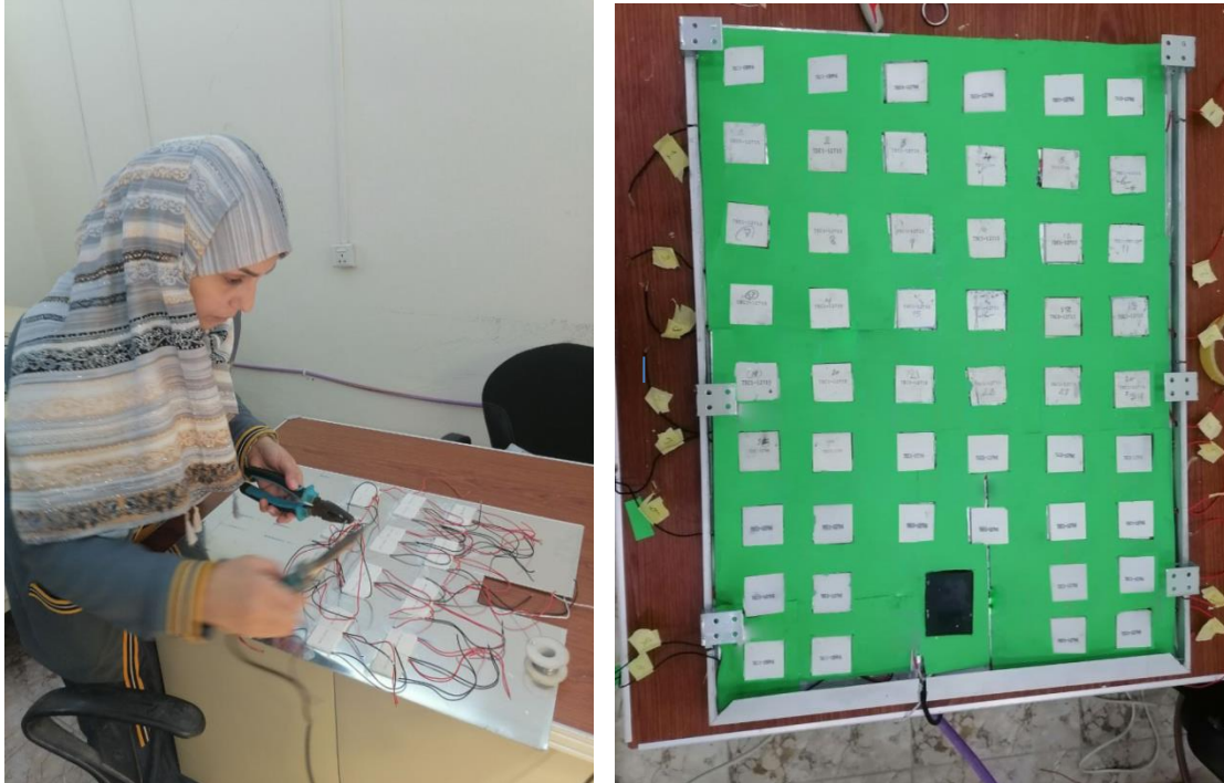
(b) Detail pictures of TEG modules arrangement and tying
