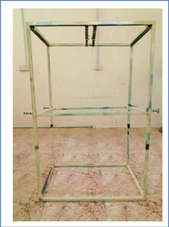
Figure 4-8: Iron structure with slider part
