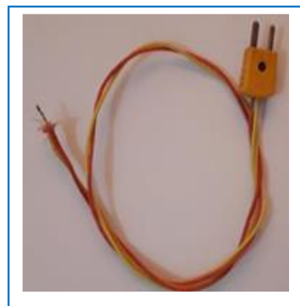
Figure 4-14: Thermocouple Type (k)
