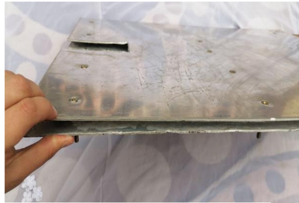
(g) Putting and linking other aluminum plate above the heat
