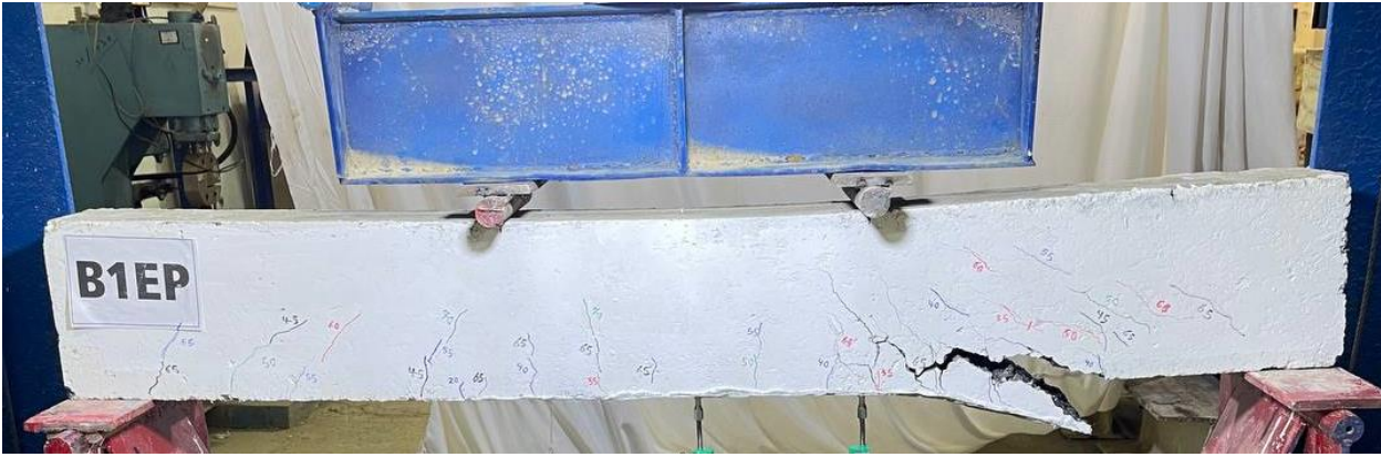
Plate 4.11: Cracks Pattern of Specimen B1EP.
