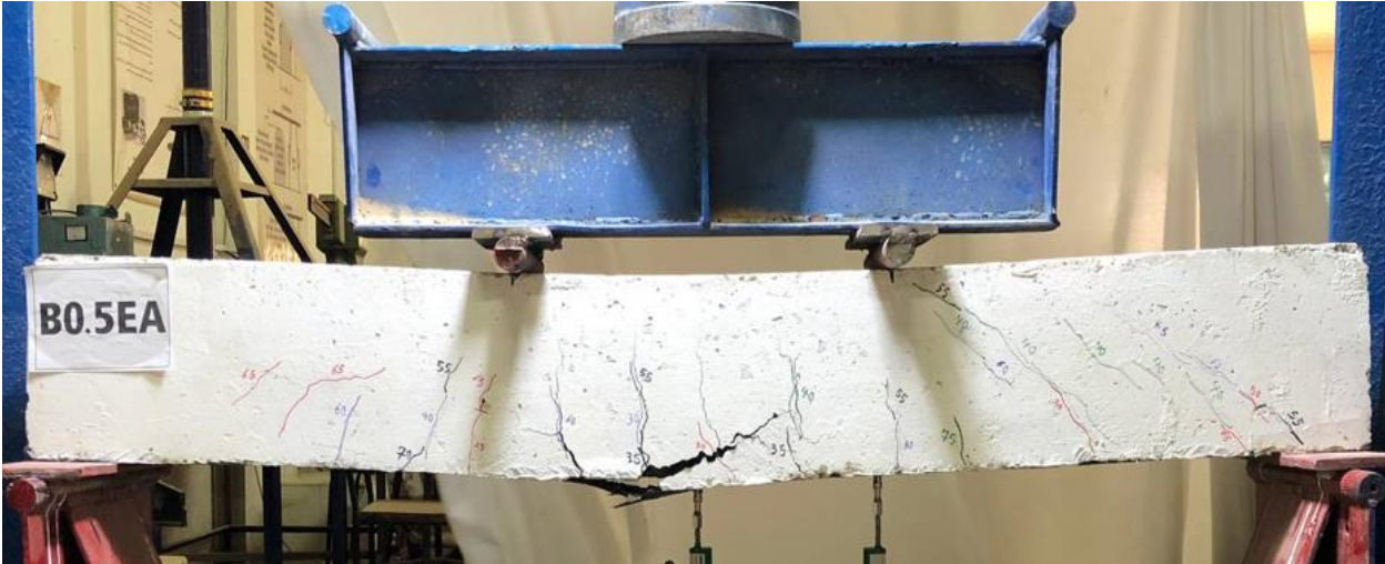
Plate 4.6: Cracks Pattern of Specimen B0.5EA.
