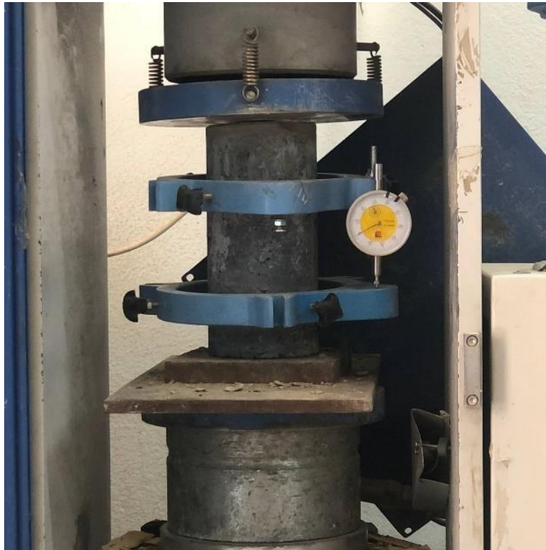
Plate 3-9: Modulus of elasticity test
