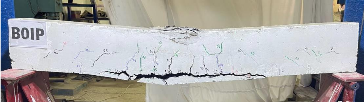
Plate 4.5: Cracks Pattern of Specimen B0IP.
