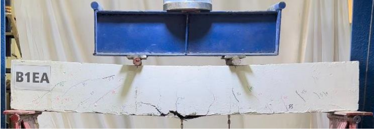
Plate 4.10: Cracks Pattern of Specimen B1EA.
