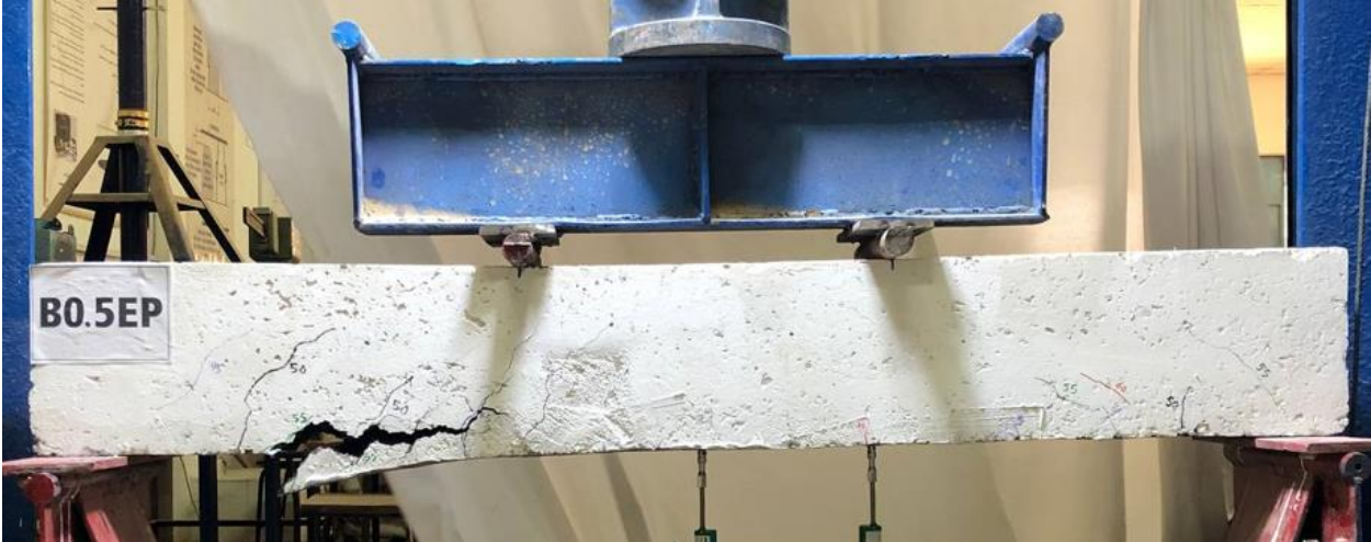
Plate 4.7: Cracks Pattern of Specimen B0.5EP.
