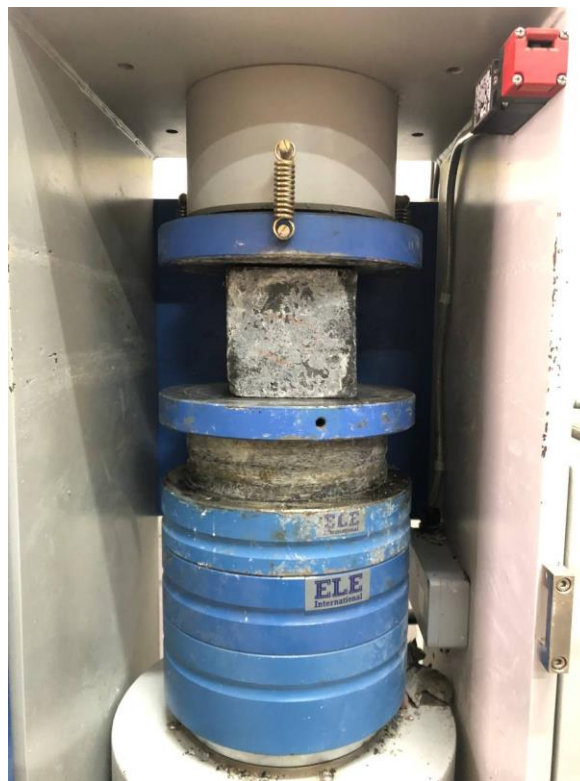
Plate 3-7: Compressive test machine.
