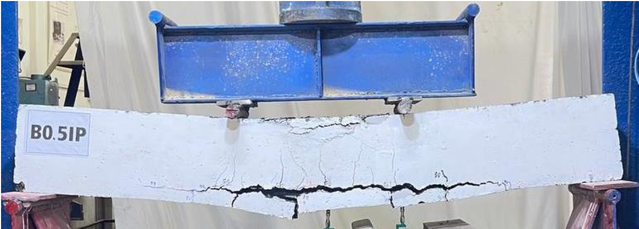
Plate 4.9: Cracks Pattern of Specimen B0.5IP.
