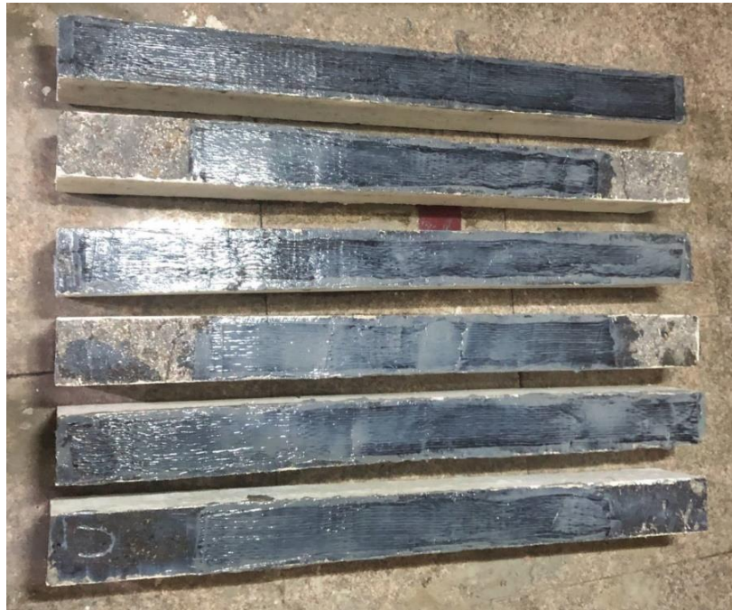
Plate 3.2: External all-strength and part-strength CFRP sheet.
