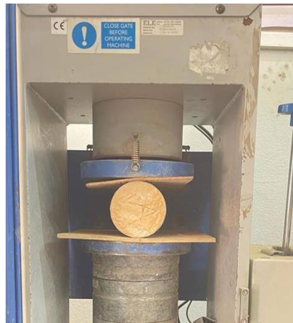
Plate 3-8: Splitting tensile strength test.
