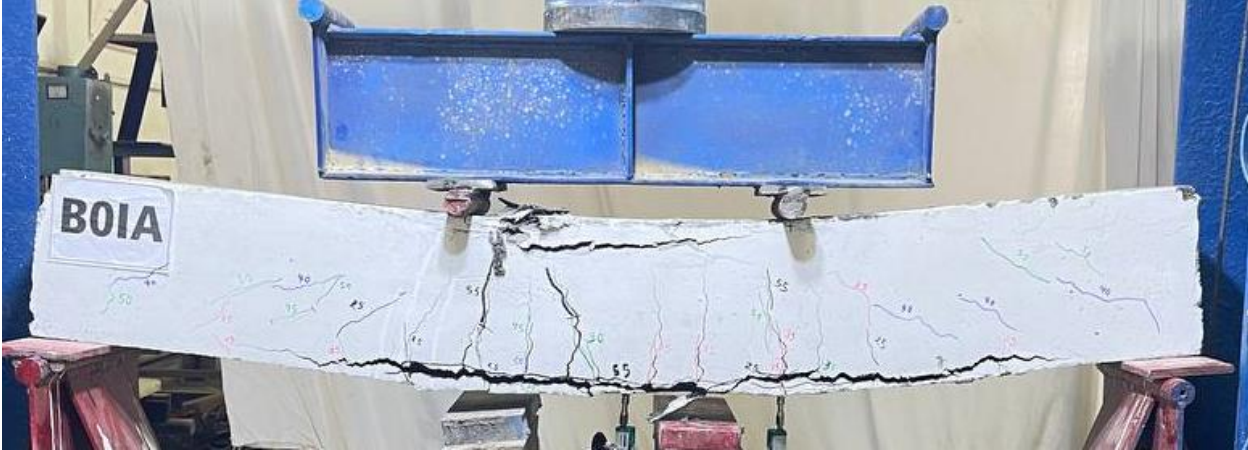
Plate 4.4: Cracks Pattern of Specimen B0IA.
