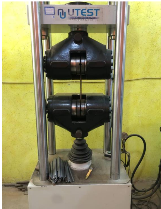
Plate 3-4: Steel bar tensile test.
