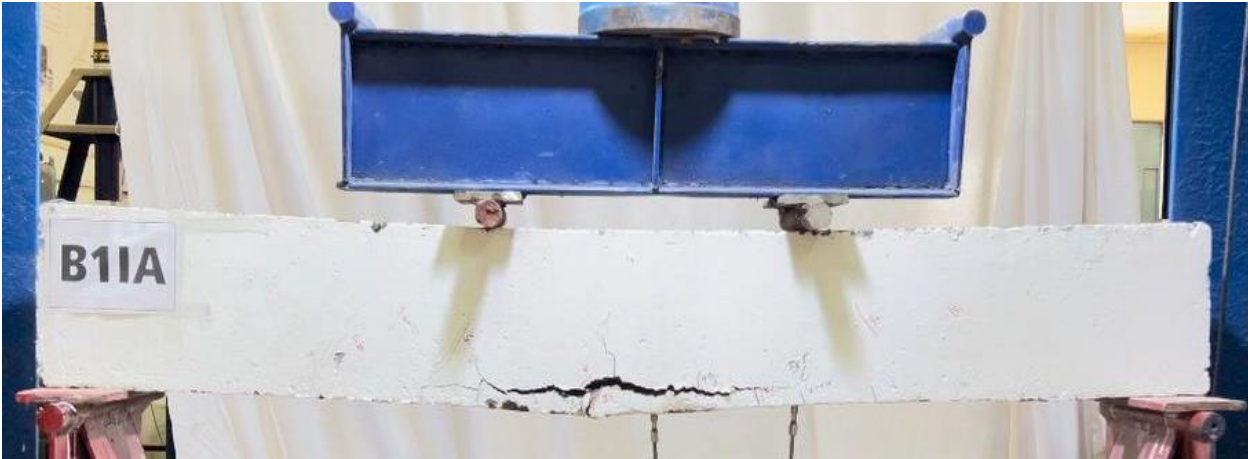
Plate 4.12: Cracks Pattern of Specimen B1IA.
