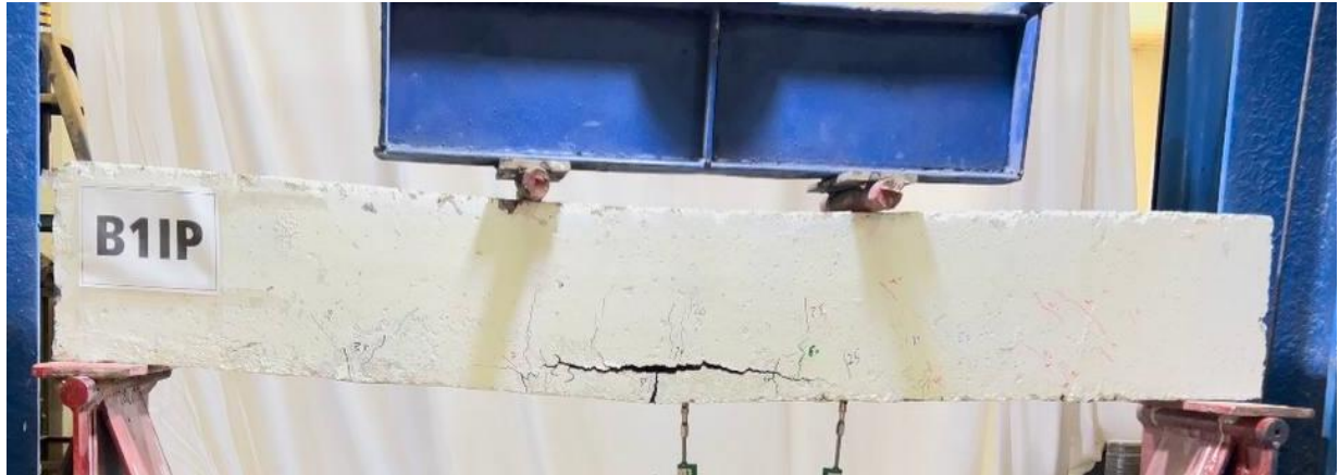
Plate 4.13: Cracks Pattern of Specimen B1IP.
