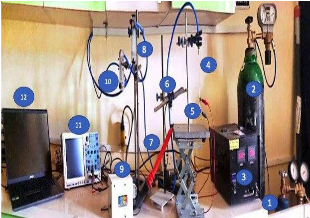
Figure 3-1 Photograph of APPJ plasma jet system (1. Oxygen gas tube, 2. Argon gas, 3. Power supply, 4. Pyrex tube, 5. Electrodes, 6. OES sensor, 7. High voltage prob, 8. Argon flow meter, 9. OES device, 10. Oxygen flow meter, 11. Oscilloscope, 12. laptop).
