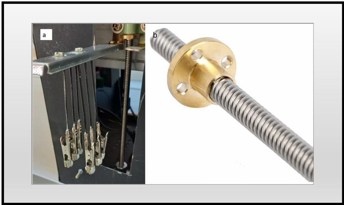
Figure 3-2. a) The developed sample holder, b) copper nut and T8 guide lead screw 300 mm.
