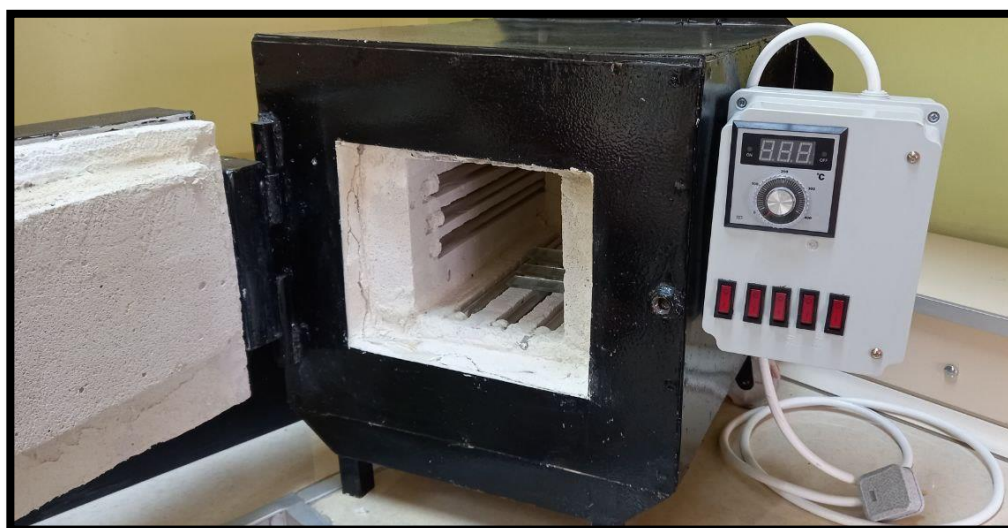
Figure 3-3. Manufacturing muffle furnace.
