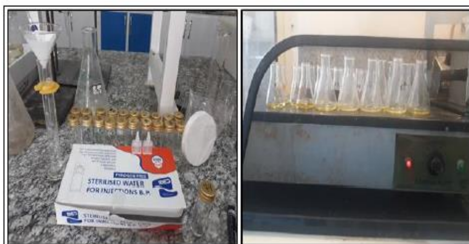
Figure 3.9. Filtering the samples using filter paper and adding deionized water.
