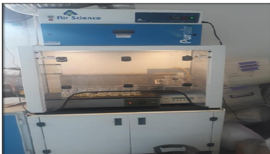
Figure 3.8. Image of the hood for discharging the fumes when preparing the samples.
