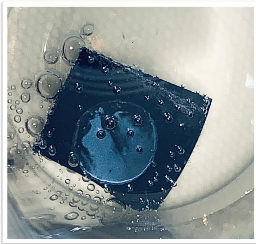
Figure (2-4), Real image when Porous layer was removing in KOH.
