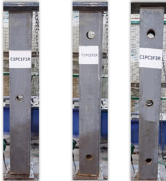
Figure 4-14: Columns with openings on opposite sides
