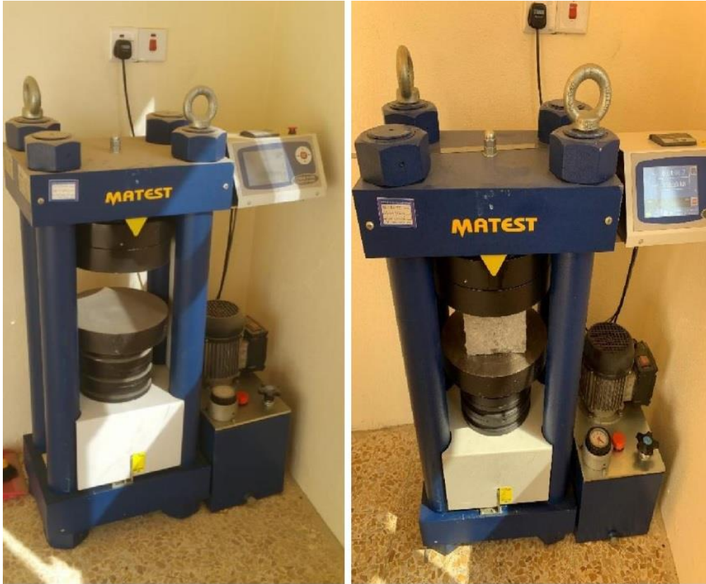
Figure 3-10: Concrete Tests Through Digital Testing Machine
