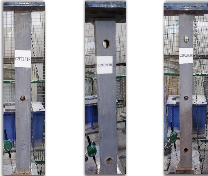
Figure 4-38: Columns with openings on opposite sides
