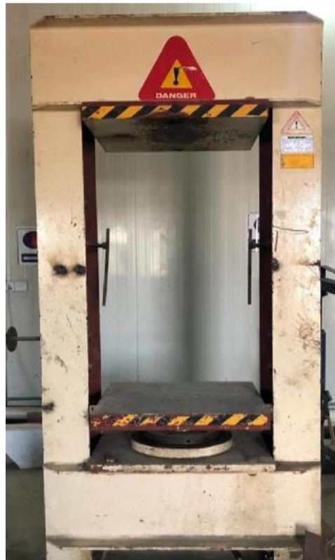
Figure 3-10: CFDST columns checking machine
