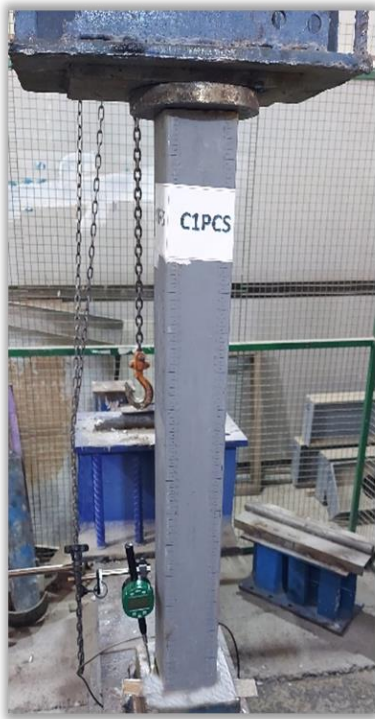
Figure 4-1: C1PCS column test
