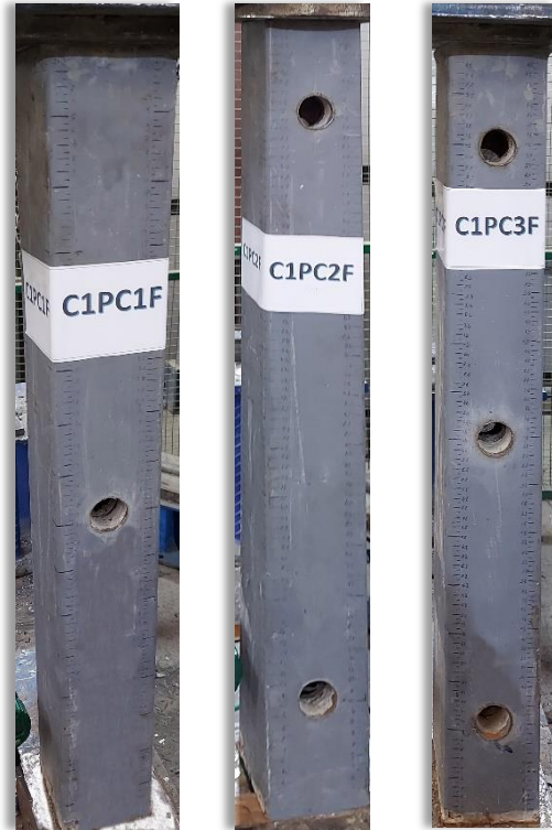
Figure 4-4: Columns with openings on one side
