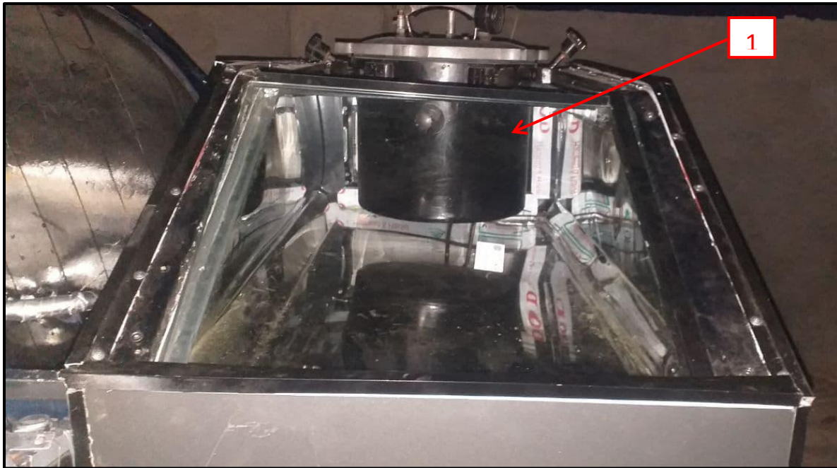
figure (4.3): Steam Sterilization Chamber: (1) Aluminum cylinder (Autoclave)
