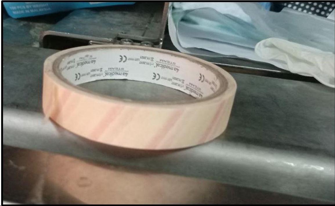
Figure (5.22): 3M™ Autoclave Steam Indicator Tape, which is Used to Check the Success of the Sterilization Process
