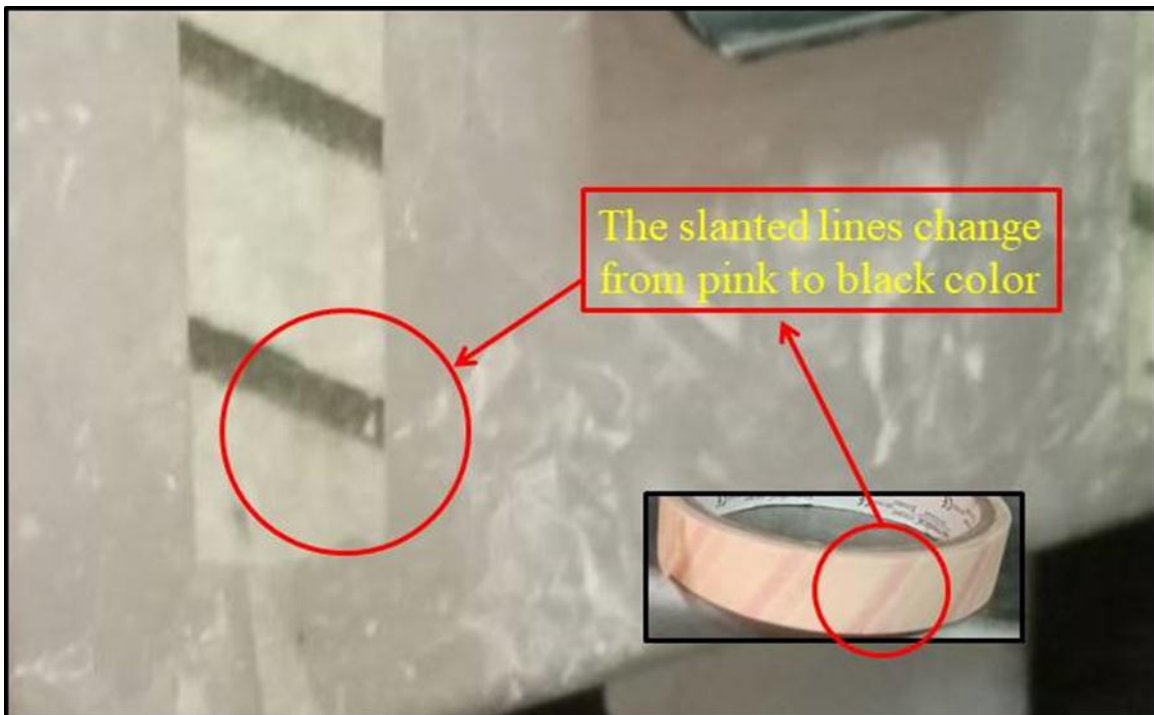
Figure (5.23): The change of the color of the slashes of the 3M™ autoclave indicator tape indicates the success of the sterilization process.
