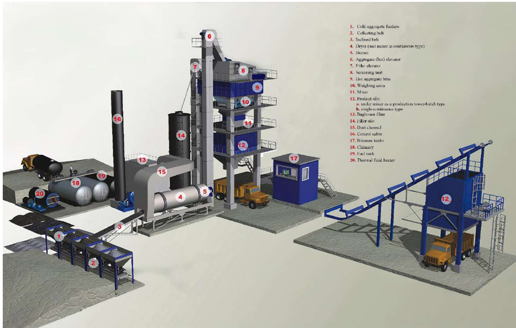
Figure 4-1: Schematic shows major components of a typical asphalt concrete unit plant (modified after (Brock & Richmond, 2007)).
