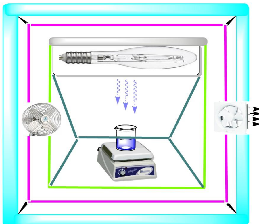
Figure (2-4). Diagrammatic representation of a Homemade Photocatalytic Reactor Unit.
