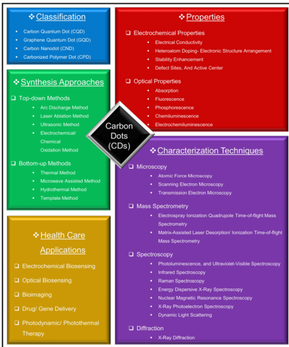
Figure1.3: The classification of CDs, their properties, synthesis approaches, characterization techniques, and applications in health care [40]
