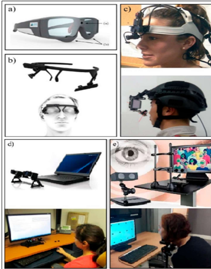
Figure 2.1 Types of eye tracking devices: (a)eye tracking glasses, (b)headband,(c)helmetmounted,(d)remote or table,(e)tower-mounted [10]
