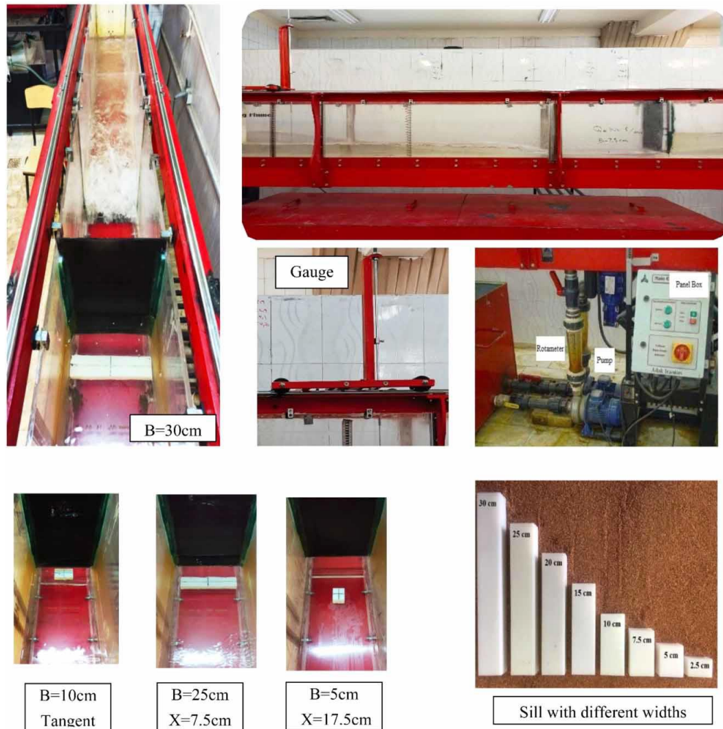
Figure 2.8 : Photographs of the experimental flume with the equipment installed on it and some of the models
