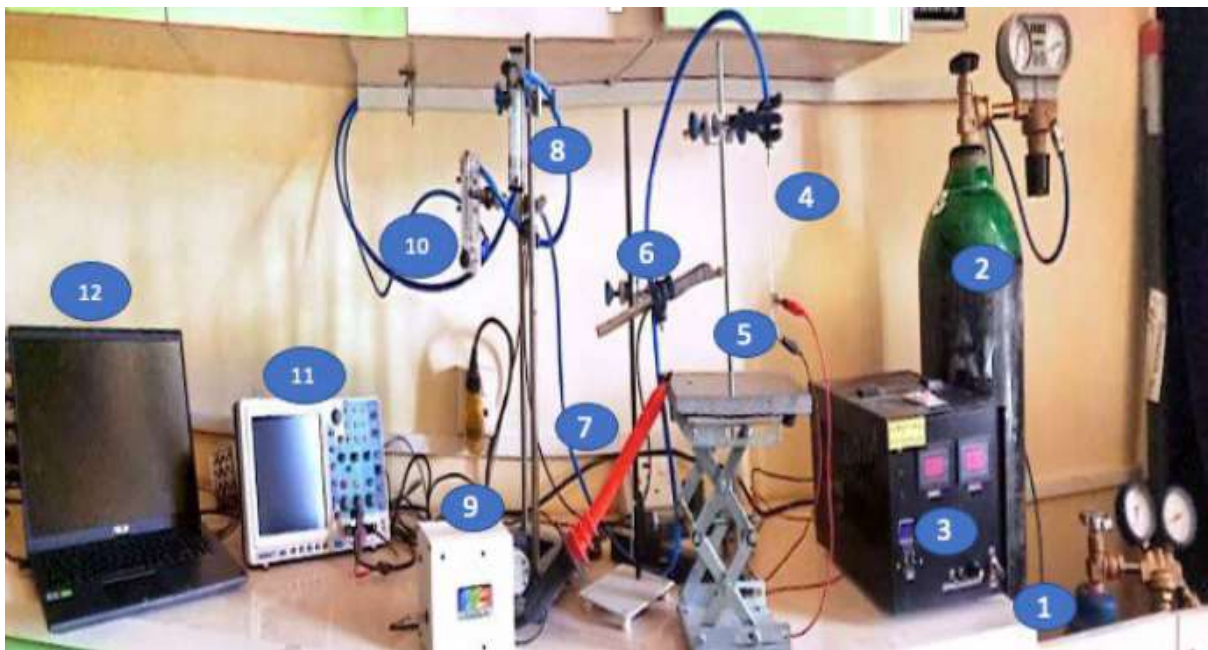
Figure (3-1): Photograph of APPJ plasma jet system:
