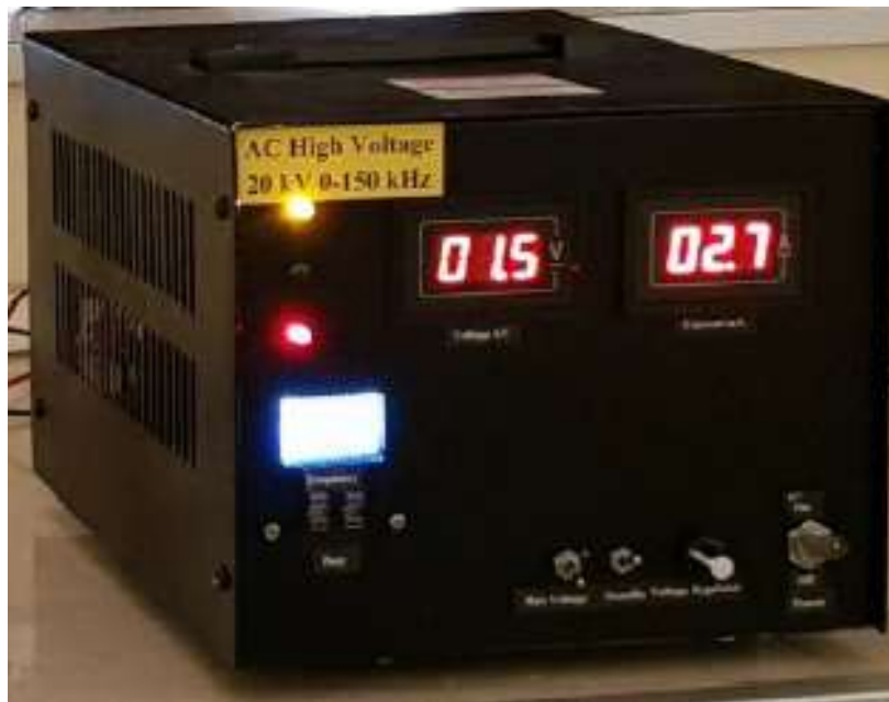
Figure (3.2): a homemade AC power source with high voltage.
