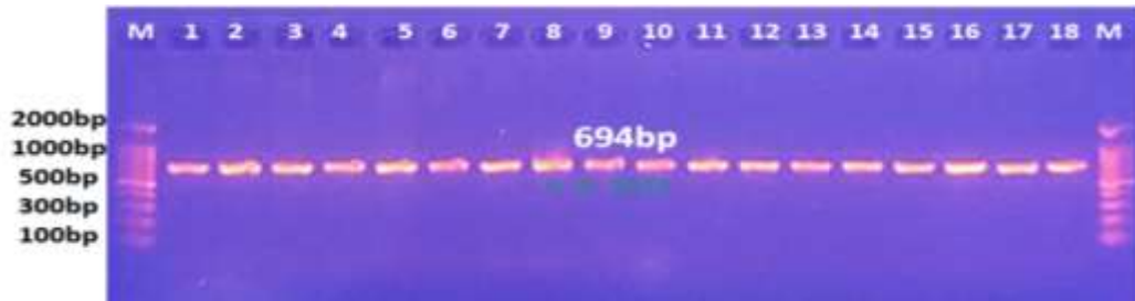
Figure(4-8):Gel electrophoresis IL17A F, IL17A R 69 of chr6 as target DNA region of IL17A(COVID-19 patient without fungal infection group)amplification region with flanking primers, number of patient PCR products 694bp,M= molecular marker 100bp for each step
