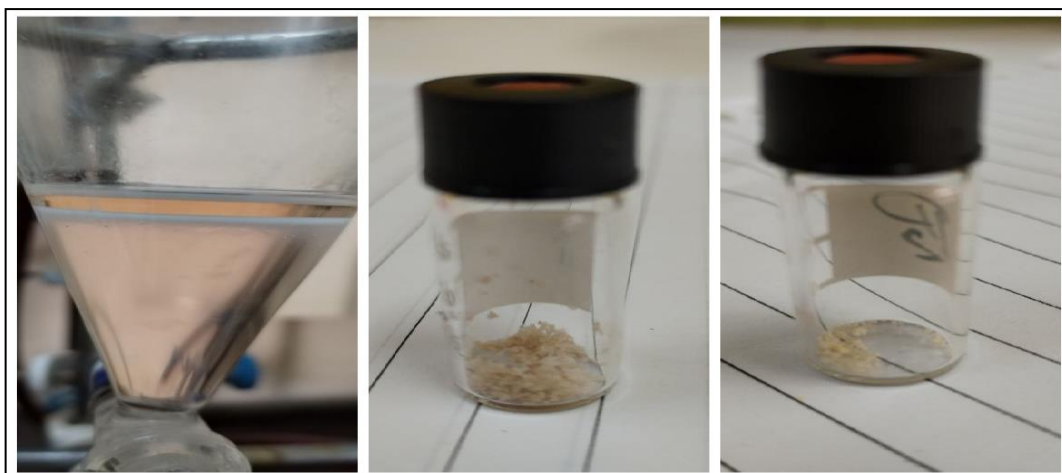
Figure (2-11): A figure showing the separation of the two layers in the separation funnel, where the ethanolic layer (at the top) and the etheric layer (at the bottom), and the products of the primary and side reaction, respectively.
