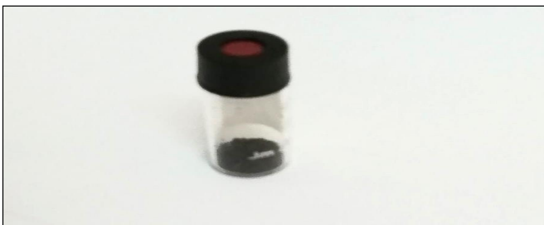
Figure (2-7): The black by product (ethyl fatty ester) which was isolated and dried.
