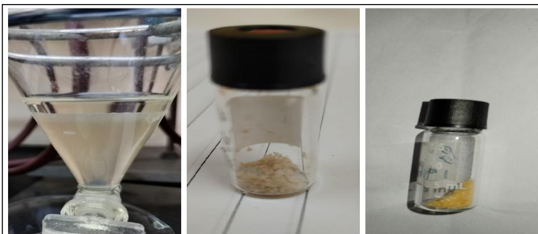
Figure (2-10): The separation funnel during the separation of the two layers, as well as the products of the etheric and ethanolic layers, respectively.
