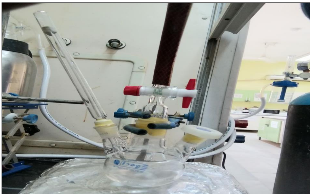
Figure (2-8): The reactor of the enzymatic hydrolysis of PC in presence of PLD.
