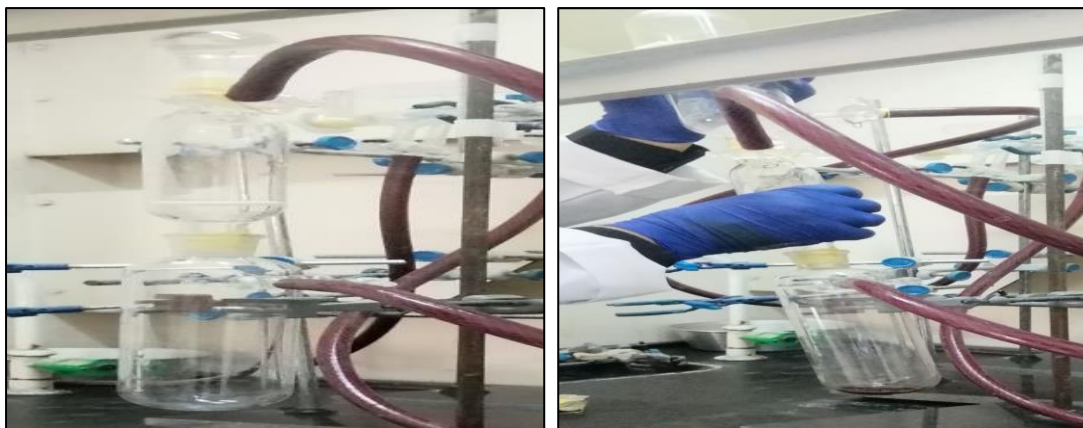
Figure (2-2): The filtration technique which was used to separate the reaction products from the side products, where the black substance on the filter surface is the byproduct. While the oil solution contains the product of the reaction with the solvent.
