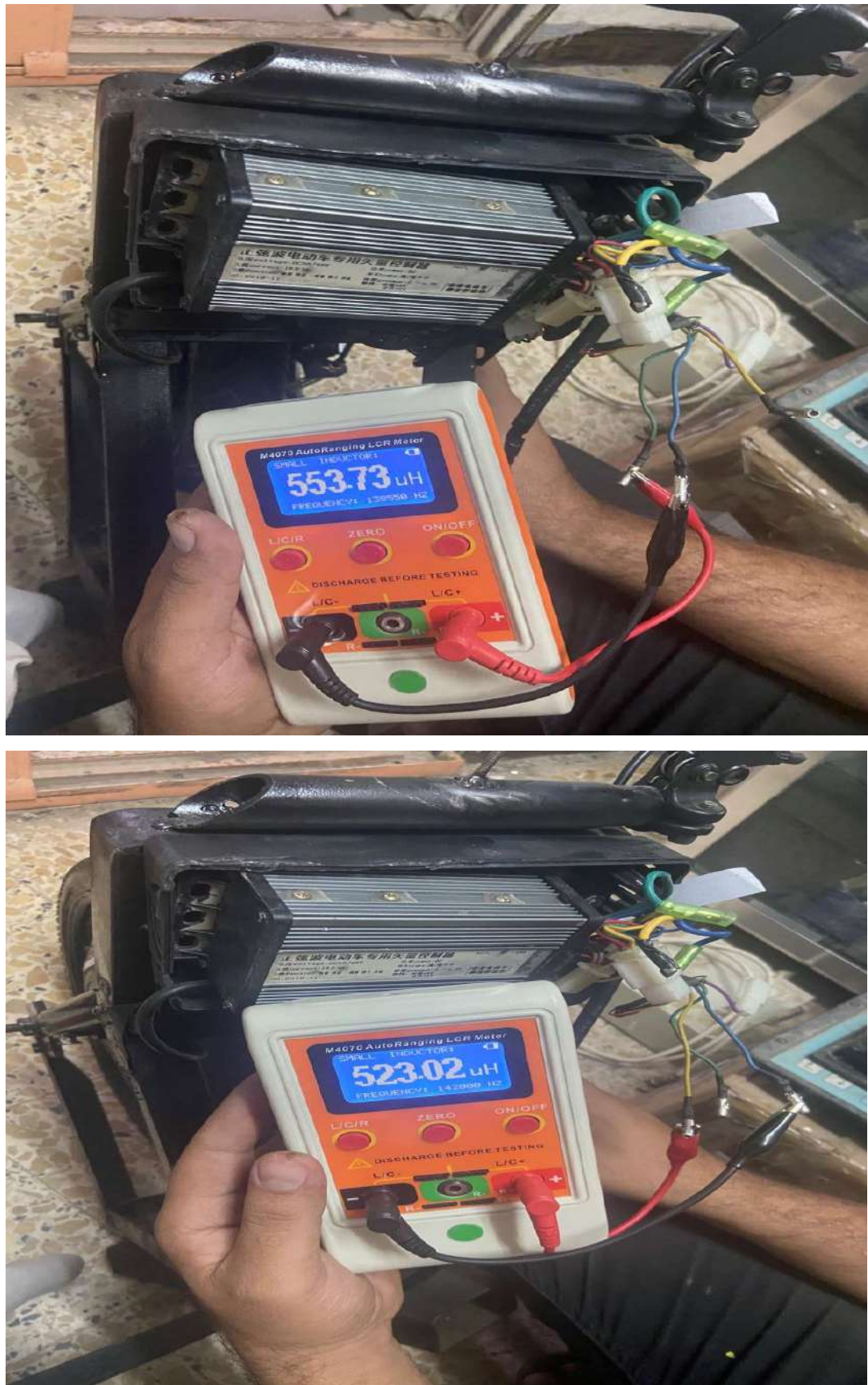
Fig A.2.4 Measuring BLDCM Inductance
