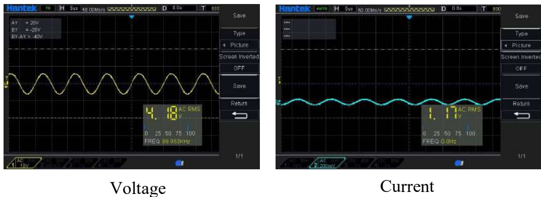
Fig. 4.10. The waveforms of the voltage and current in Rx side 5 cm.
