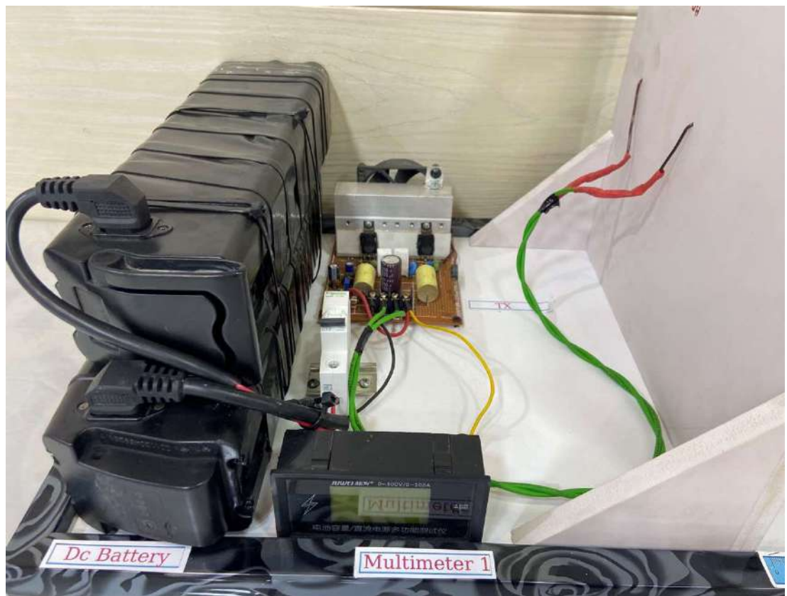
Fig A.2.2 Battery and TX Circuit Large Scale Prototype
