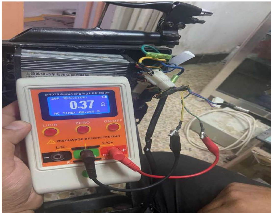
Fig A.2.3 Measuring BLDCM Resistance
