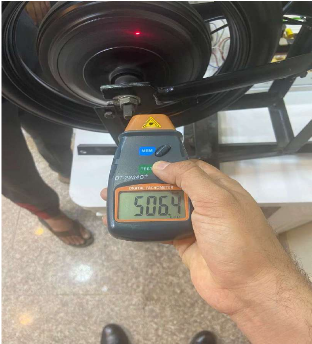
Fig A.2.5 Measuring BLDCM RPM
