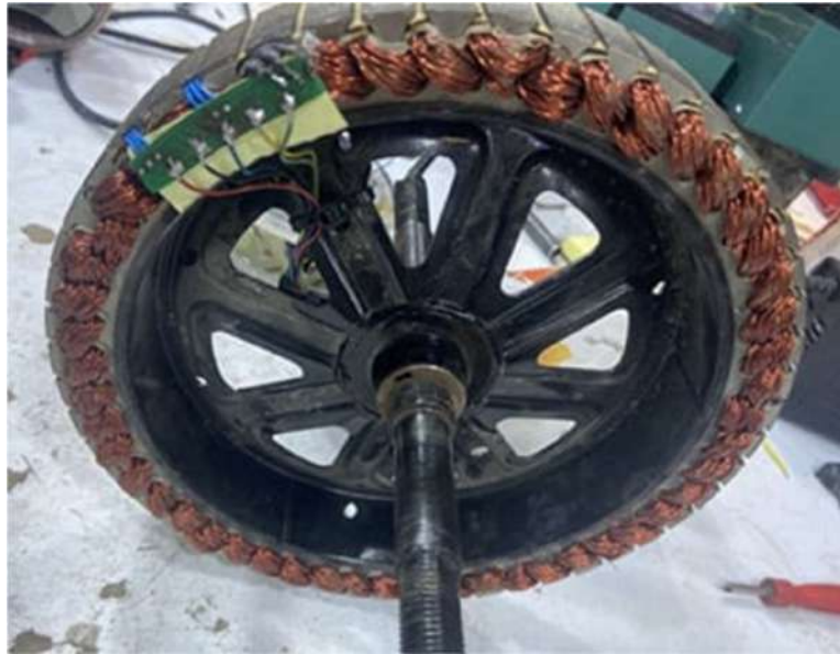
Fig. 3.6. The practical BLDCM with its drive circuit
