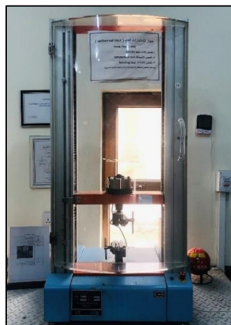
Figure 4.44:The universal testing machine (Max Load 5 KN).
