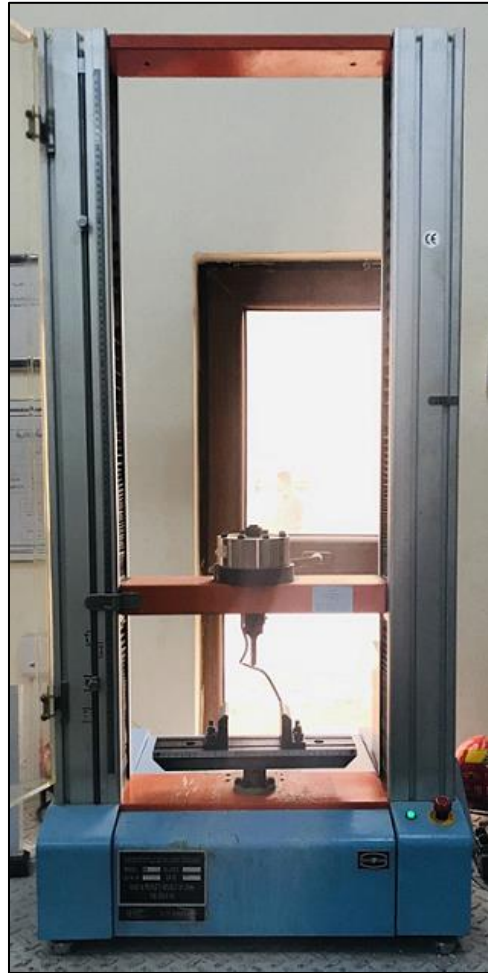
Figure 4.36: The universal test machine (Max Load 5 KN)
