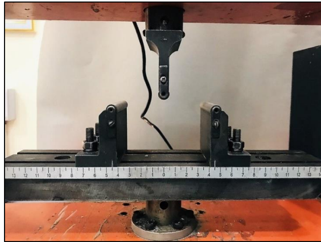
Figure 4.37: The roller used with a universal test machine.
