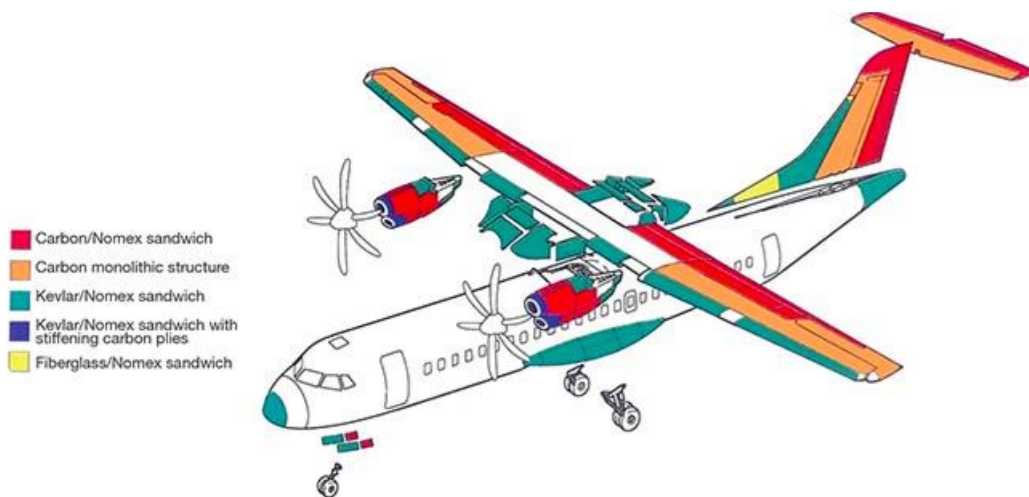
Figure 1.1: Composite Sandwich Structures in ATR 72 Airframe [4]
