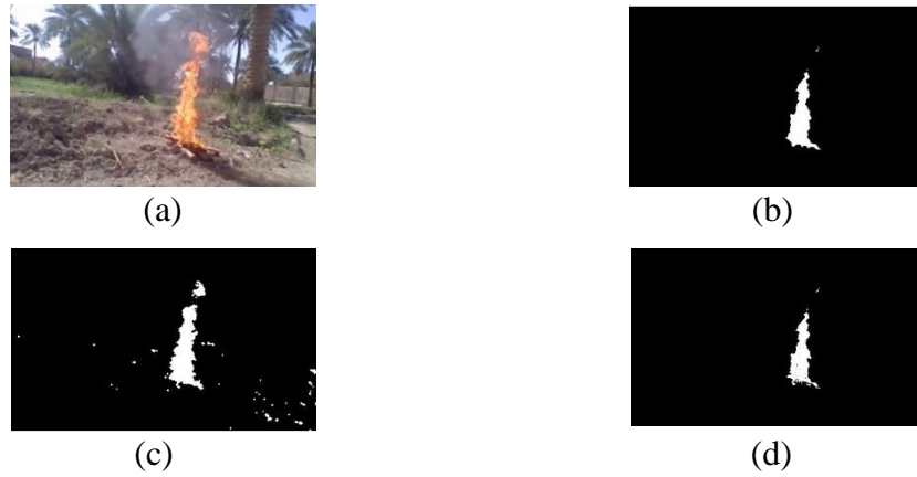
Figure 3.36 The combination of two colors of flame. (a.) Outdoor place in RGB_N -Frames 1 . (b. and c.) based HSV for POS-Otsu and YCbCr (d.) The combination between b and c.
