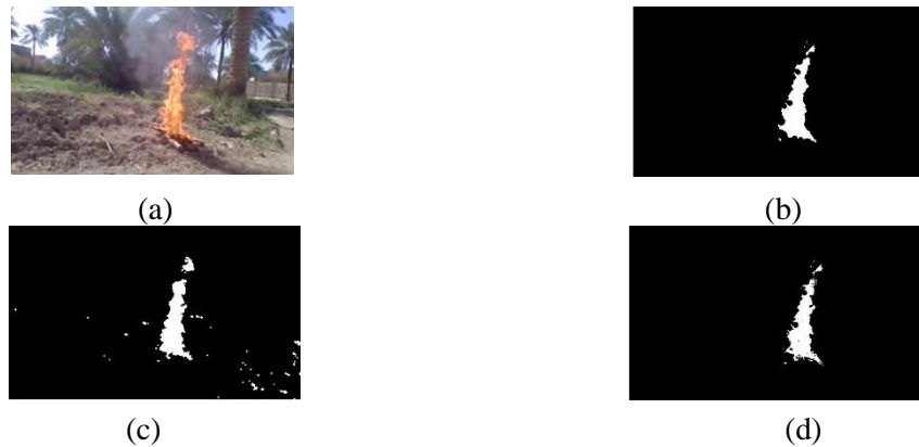
Figure 3.38 The combination of two colors of flame. (a.) Outdoor place in RGB_N Frames 1 . (b. and c.) based HSV for FOA-Otsu and YCbCr (d.) The combination between b and c.
