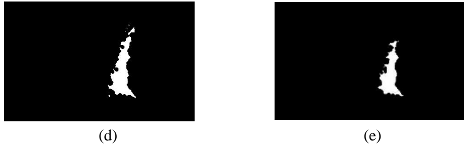
Figure 3.31 The morphological process of the adaptive flame detection for outdoor (a.) Original RGB_N frame (b.) based on POS-Otsu (c.) based on POS-Kapur (d.) based on FOA-Otsu (e.) based on FOA-Kapur.
