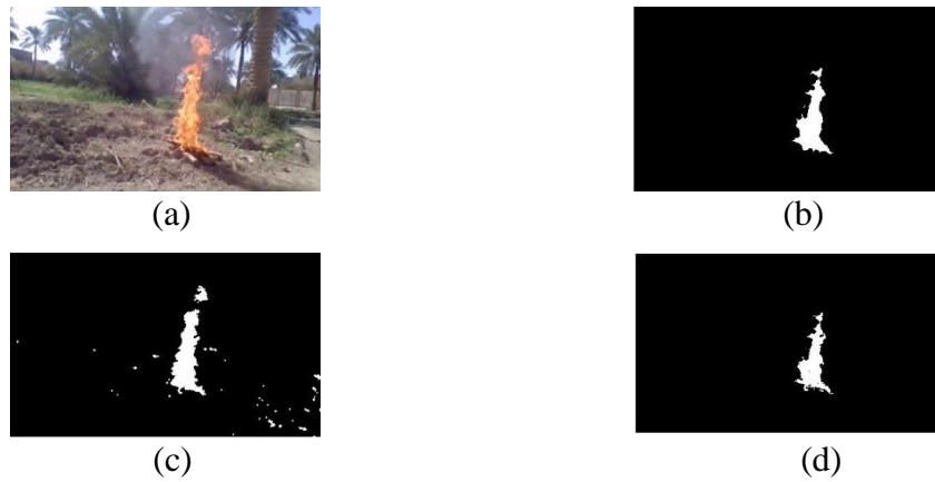
Figure 3.37 The combination of two colors of flame. (a.) Outdoor place in RGB_N -Frames 1 . (b. and c.) based HSV for POS-Kapur and YCbCr (d.) The combination between b and c.
