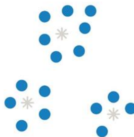
Figure 2.11 K-means clustering represents groups by their centroid - each member's average (Cluster Analysis and Clustering Algorithms - MATLAB & Simulink 2022).
