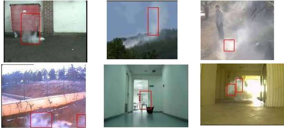
Figure 4.3 The proposed smoke detection using KMU Fire & Smoke Database and VisiFire dataset.
