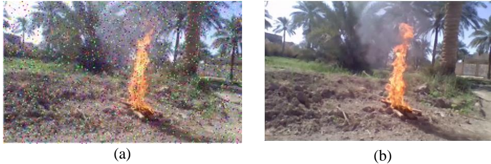
Figure 2.3 Image filtering (a.) image with salt and pepper noise (b.) The noise elimination by median filter.
