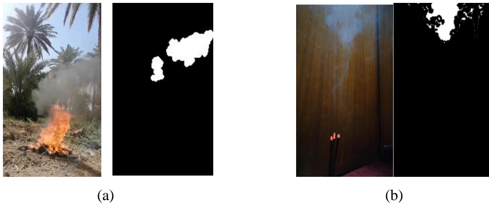
Figure 3.30 The morphological process for smoke color detection-based CIE L^*a^*b by static thresholds for (a.) outdoor place (b.) indoor place.
