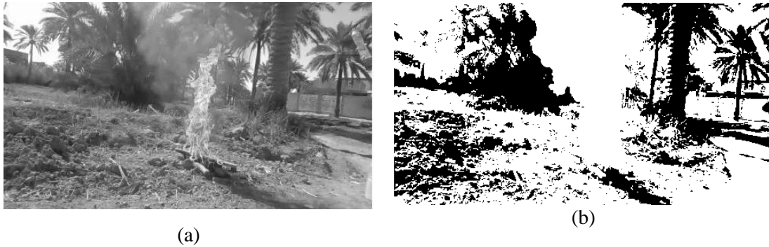
Figure 2.8 Kapur thresholding (a.) original image (b.) result of Kapur method.
