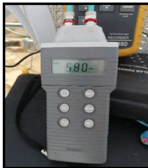
Figure 4-15: Digital Pressure Meter.
