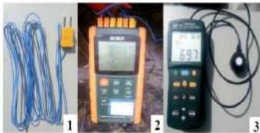
Figure 3. Instruments for measuring: 1-thermocouples, 2-temperature meter, 3-solar power meter
