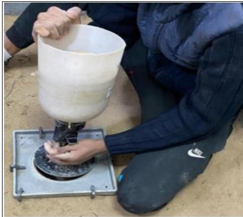
Figure (3.17): Sand Replacement Method
