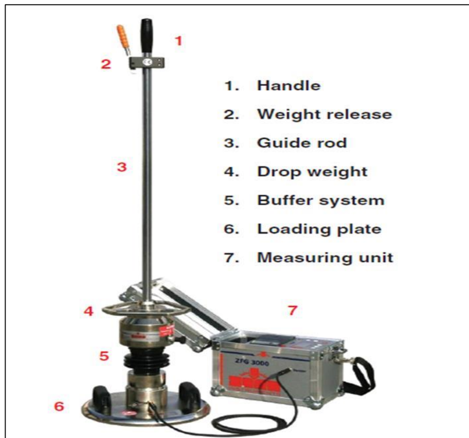
Figure (3.15): LWD Tests Device (Shaban et al., 2016).
