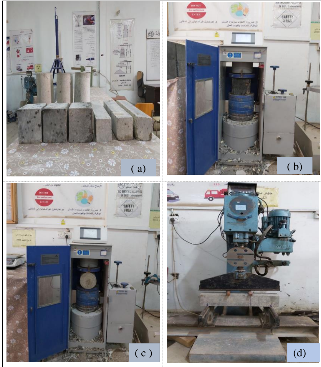
Figure 3-8: Mechanical properties tests : (a) numbers and shapes of specimens, (b) compressive strength, (c) splitting tensile strength, and (d) Modulus of Rupture.
