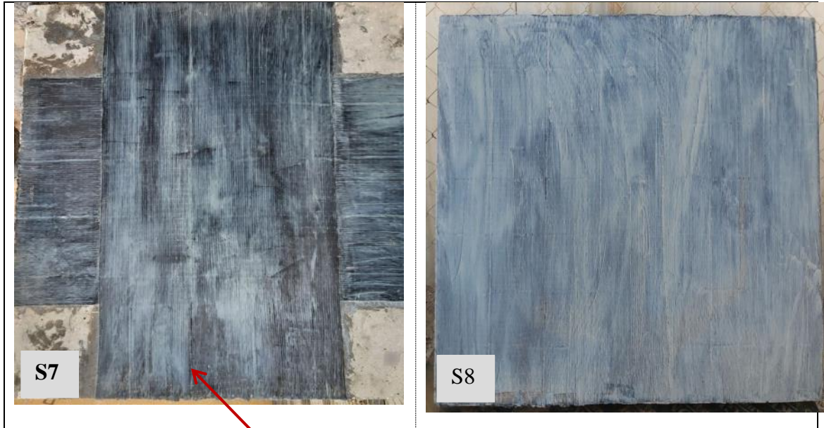
Figure 4-6: Compression zone after repeated loading at slabs S7 and S8.
