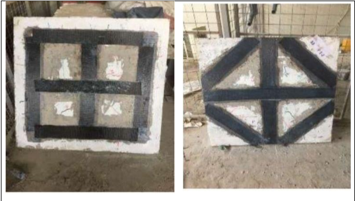
Figure 2-7: Two distribution method of the CFRP sheets adopted from Mutlaq et al. (2020).
