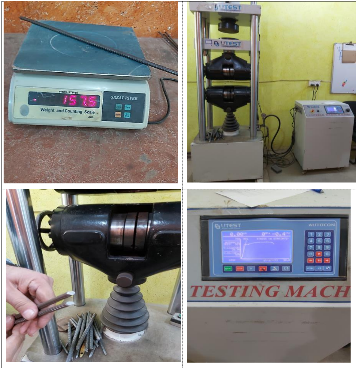
Figure 3-1: Steel bars testing at the laboratory of the University of Kerbala.
