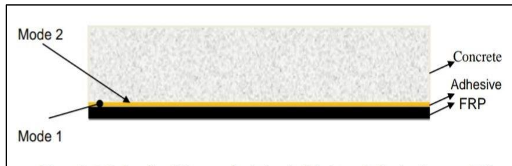
Figure 1-6: Debonding failure modes induced of the loss of adhesion between FRP and concrete substrate (Daud, 2015).
