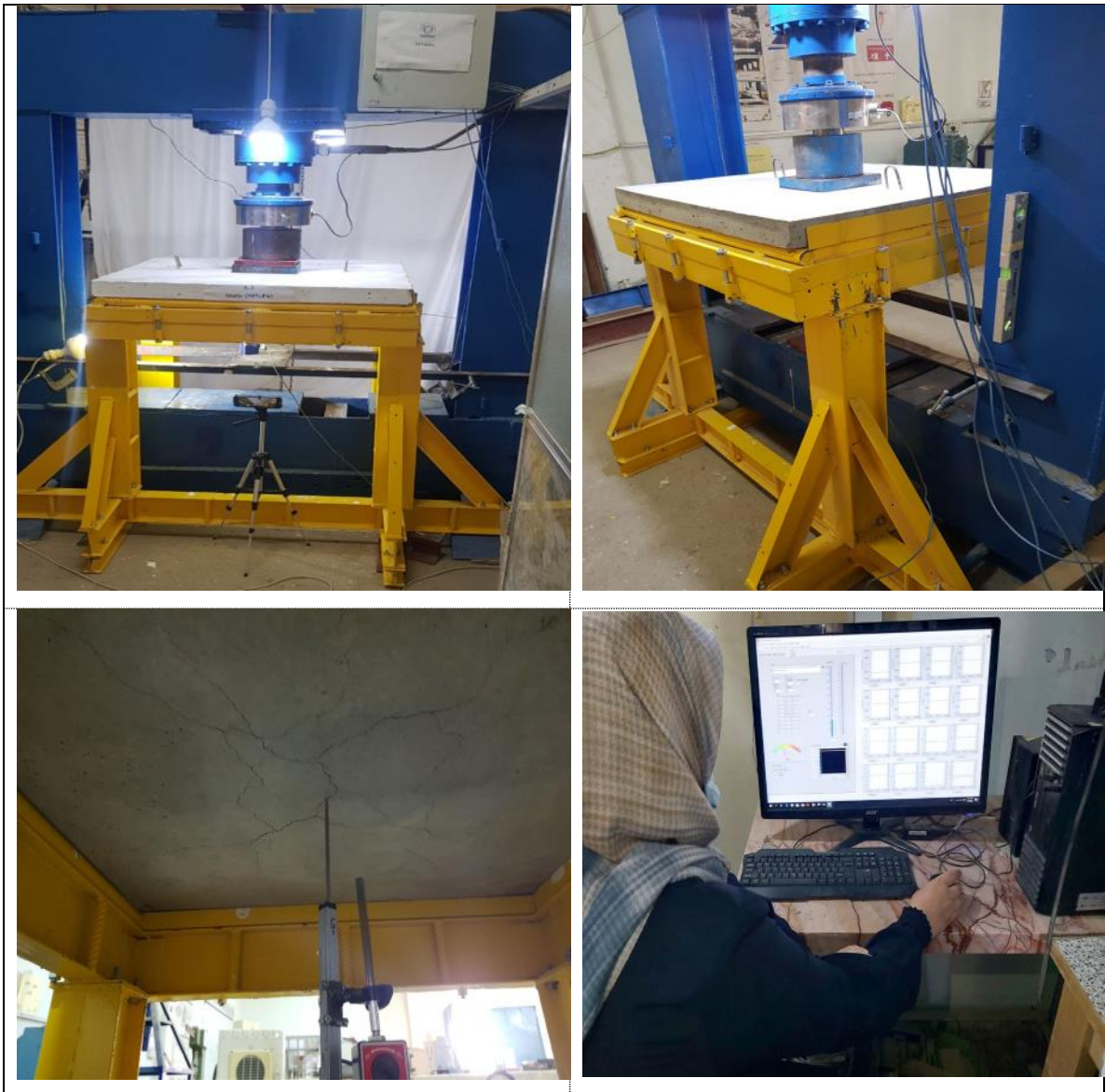
Figure 3-9: Multiple images represent the test stages of the slab, the steel frame, the LVDT, and the control computer.
