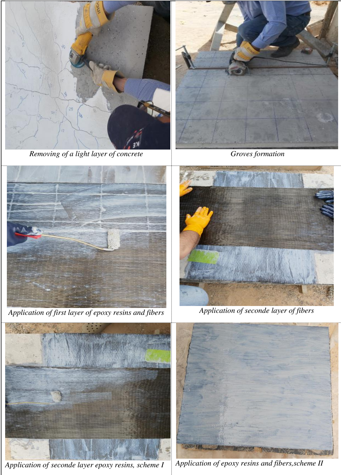
Figure 3-13: Application of CFRP sheets at the tensile face of tested slabs.
