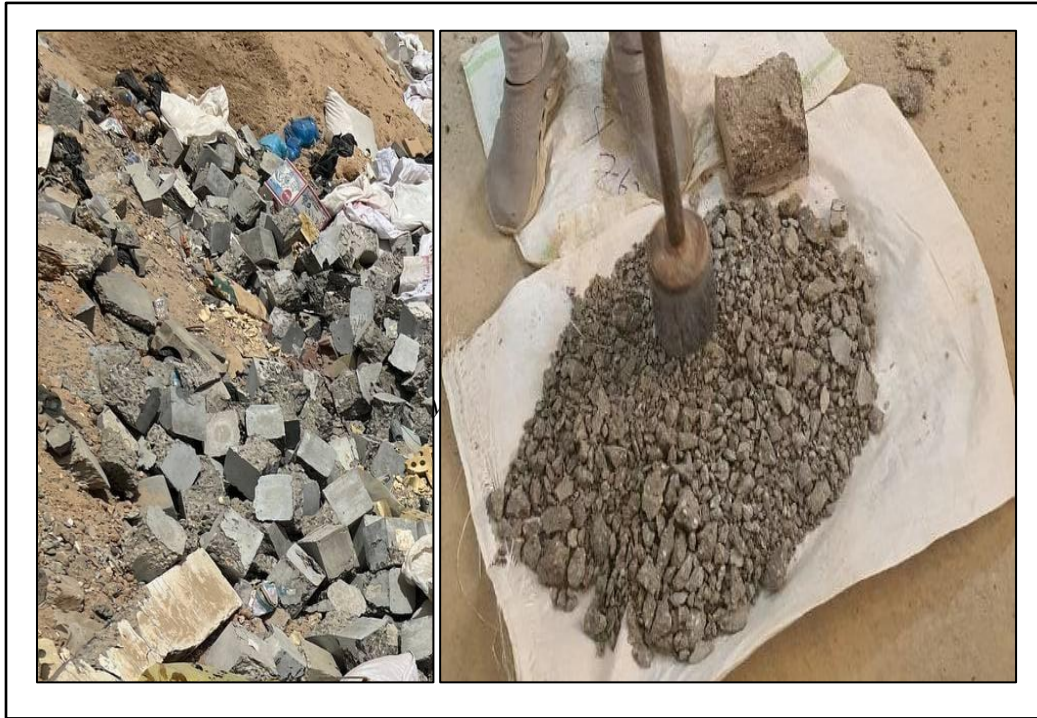
Figure 3-9: The Assembly and Crushing Of R.C.A.
