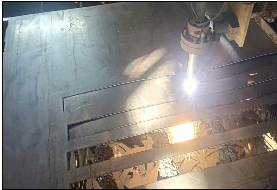
Figure 3-5: Cutting Parts for Flange and Web Plates by CNC machain
