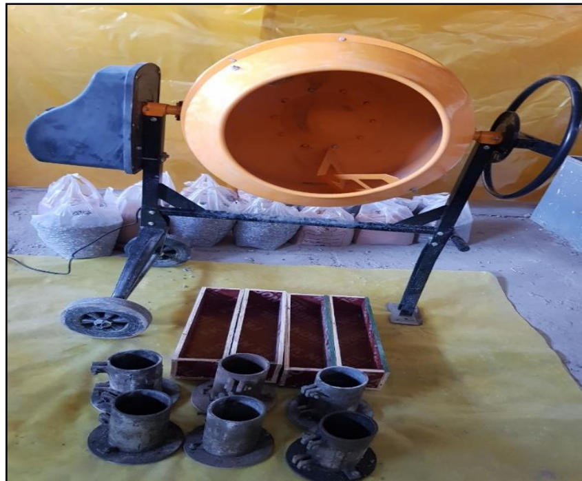
Figure 3-13: Rotating Machine Used for The Production of (NC).
