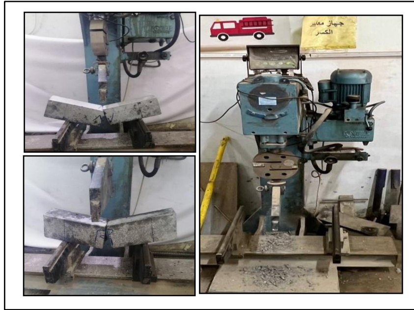
Figure 3-17: Modulus of Rapture (Test Sample and Machine).
