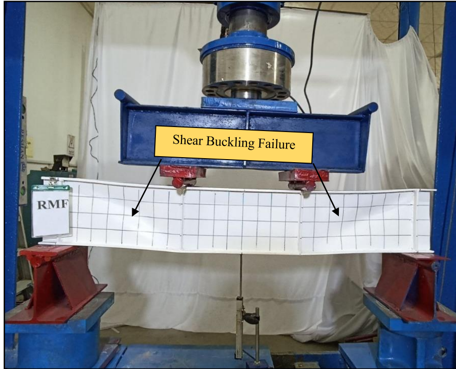
Figure 4-19: Specimen RMF During the Laboratory Examination.
