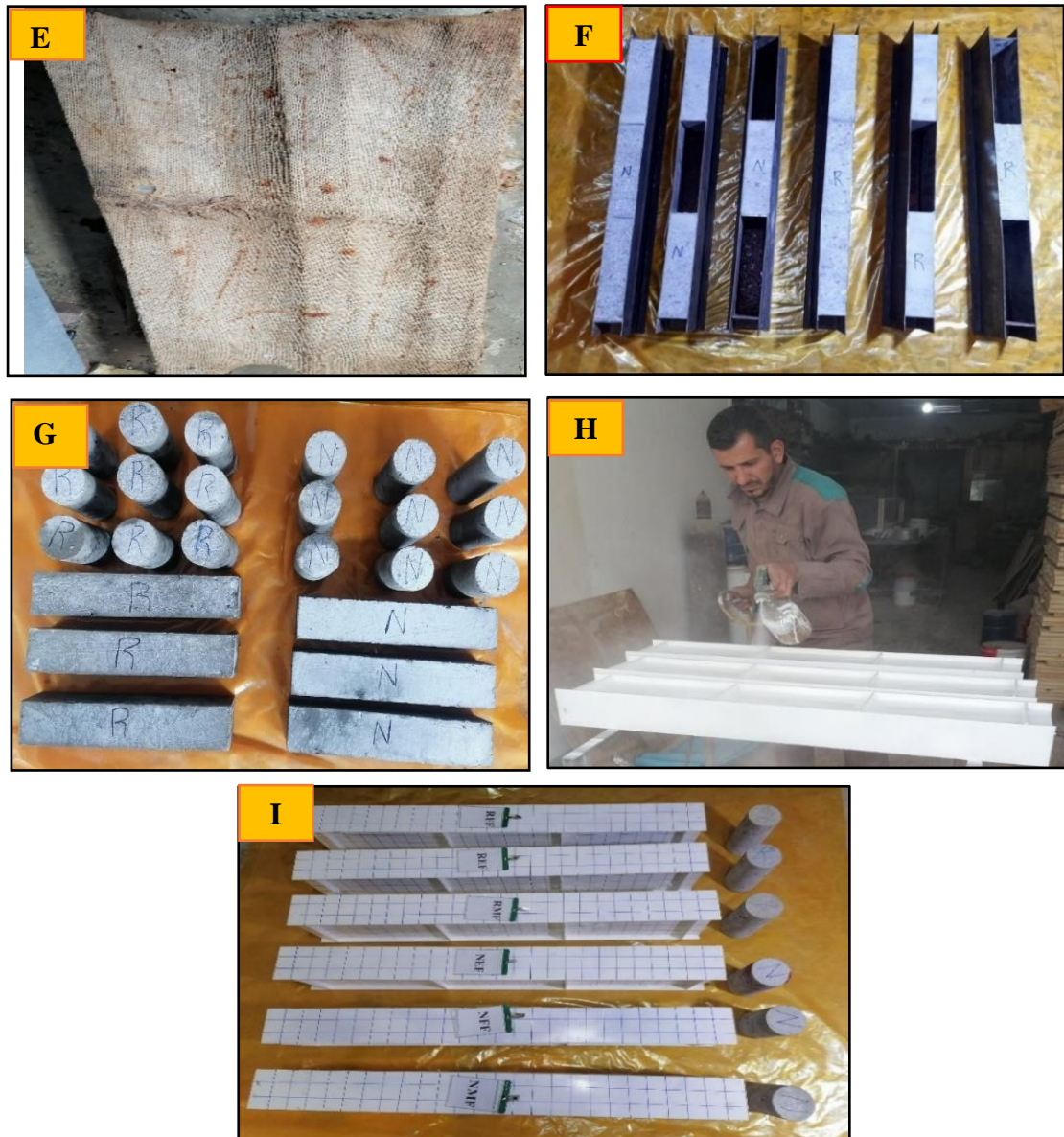
Figure 3-14: Stages In The Production of Test Specimens (A, B) Preparation And Mixing Of Materials; (C, D)- Casting And Vibration Of Concrete;(E) Curing Of Concrete;(F-I) Painting And Layout Of Samples.
