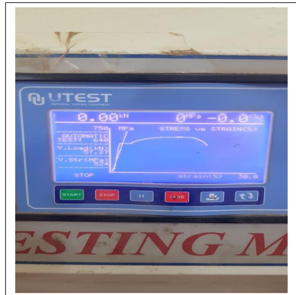
Figure 3.2: Steel Bar Tensile Machine
