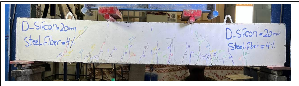
Figure 4.13: Cracking Pattern of Specimen D20-4F.
