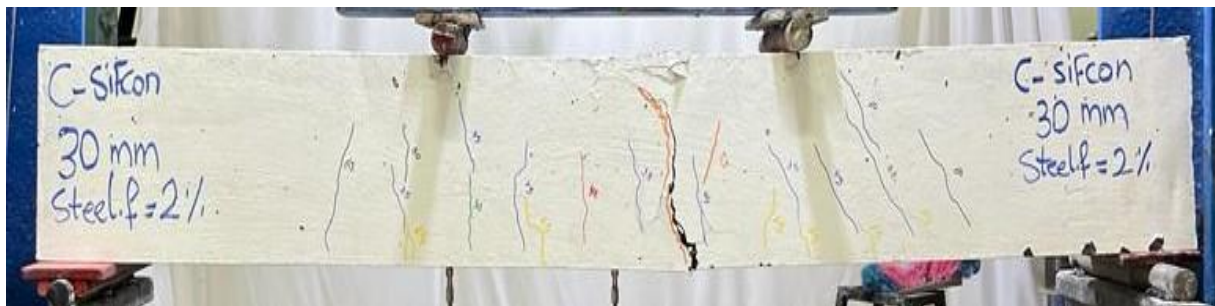
Figure 4.9: Cracking Pattern of Specimen C30-2.
