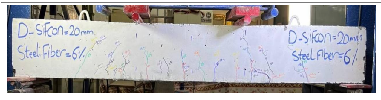
Figure 4.14: Cracking Pattern of Specimen D20-6F.
