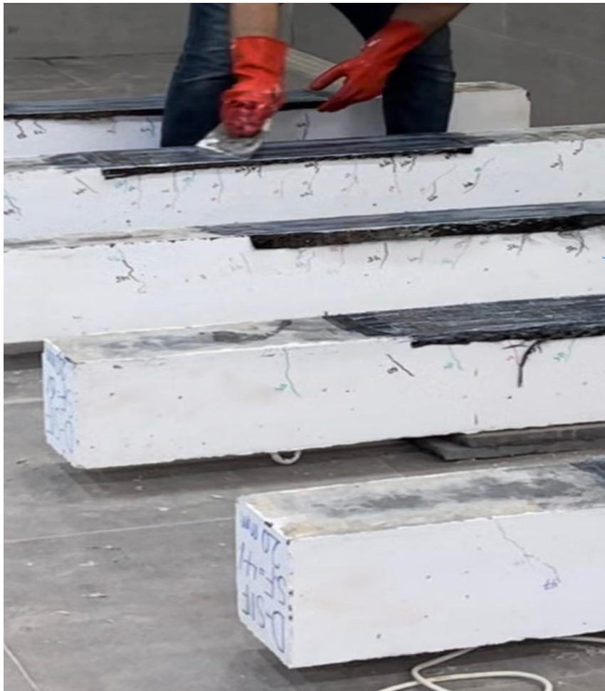
Figure 3.15 External Strengthening with CFRP sheets of Tested Beams
