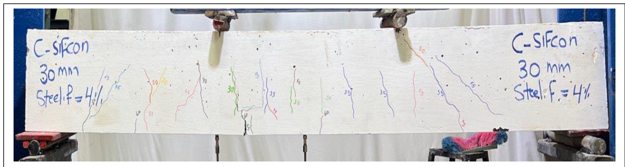
Figure 4.10: Cracking Pattern of Specimen C30-4.
