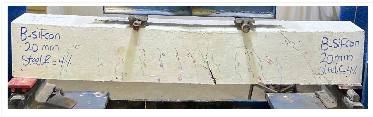
Figure 4.7: Cracking Pattern of Specimen B20-4.
