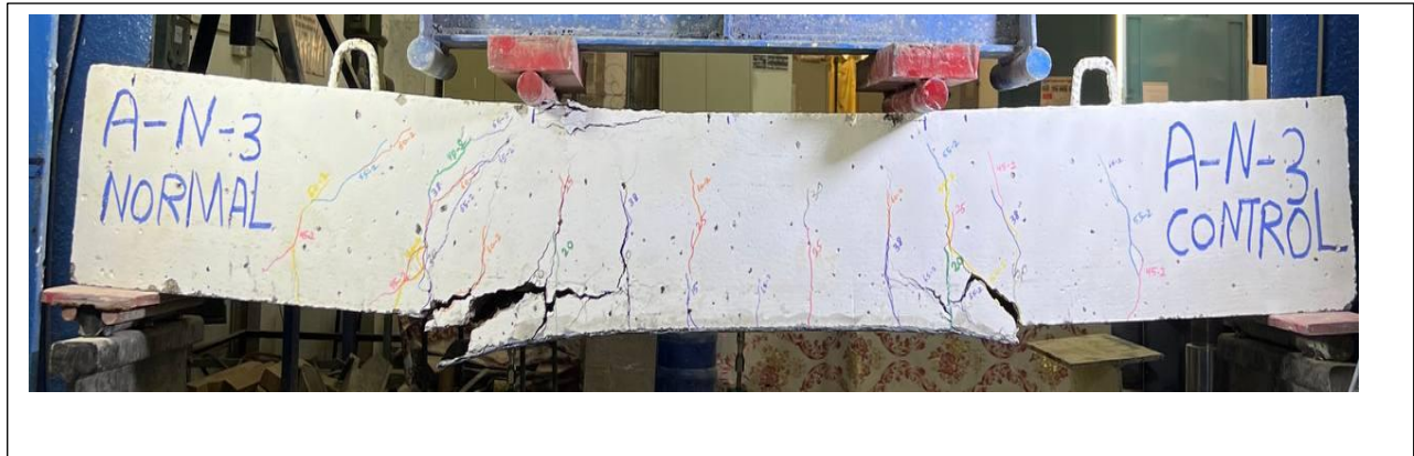
Figure 4.5: Cracking Pattern of Specimen A-NF.
