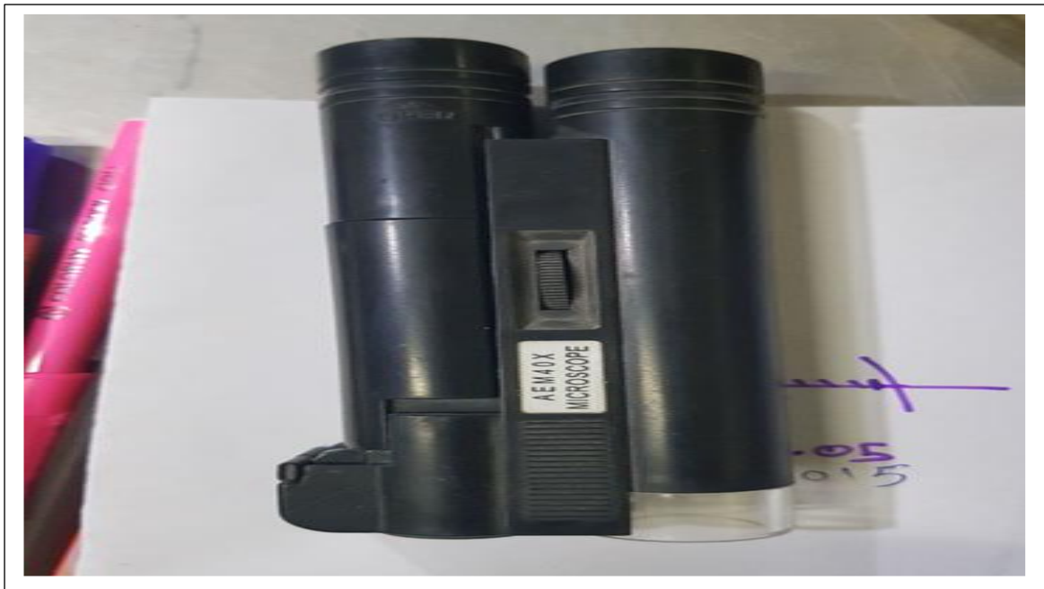
Figure 3.17: Crack Meter Microscopic Device.
