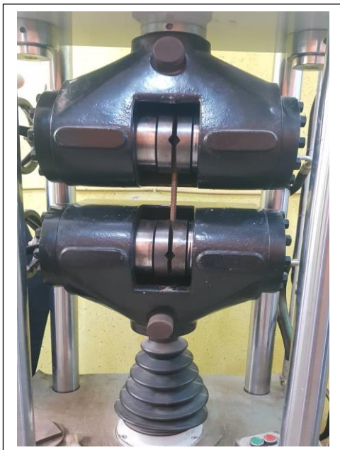
Figure 3.2: Steel Bar Tensile Machine
