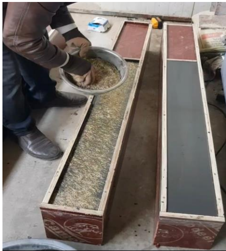
Figure 3.5 Wooden prismatic specimens' moulds
