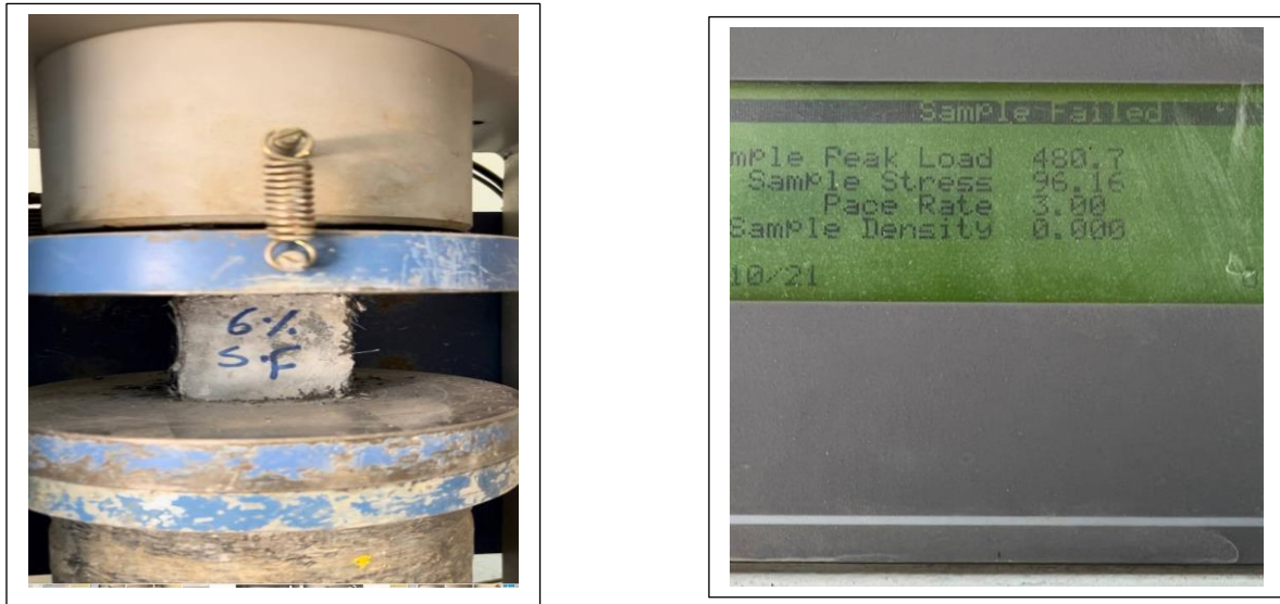
Figure 3.8: Concrete compressive Test Machine.
