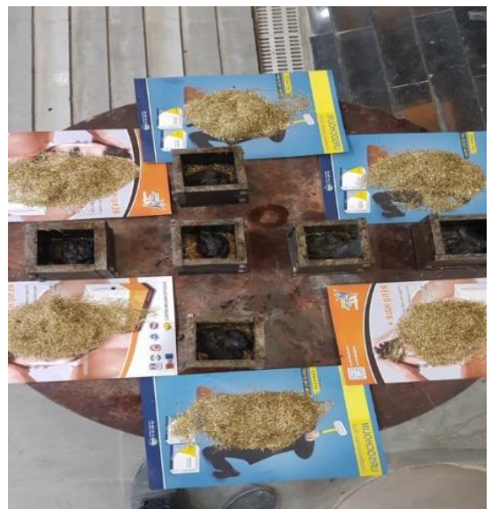
Figure 3.5 Wooden prismatic specimens' moulds
