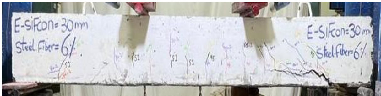
Figure 4.17: Cracking Pattern of Specimen E30-6F.
