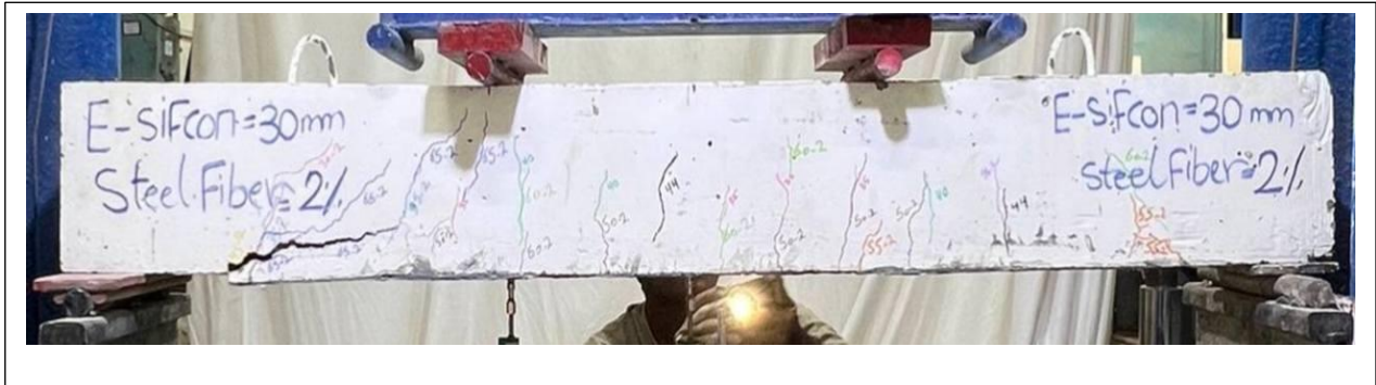
Figure 4.15: Cracking Pattern of Specimen E30-2F.
