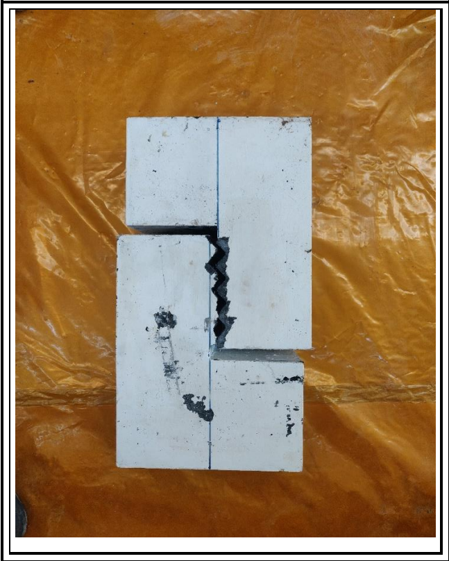
Figure 4- 9.Failure mode TRG 25 specimen.
