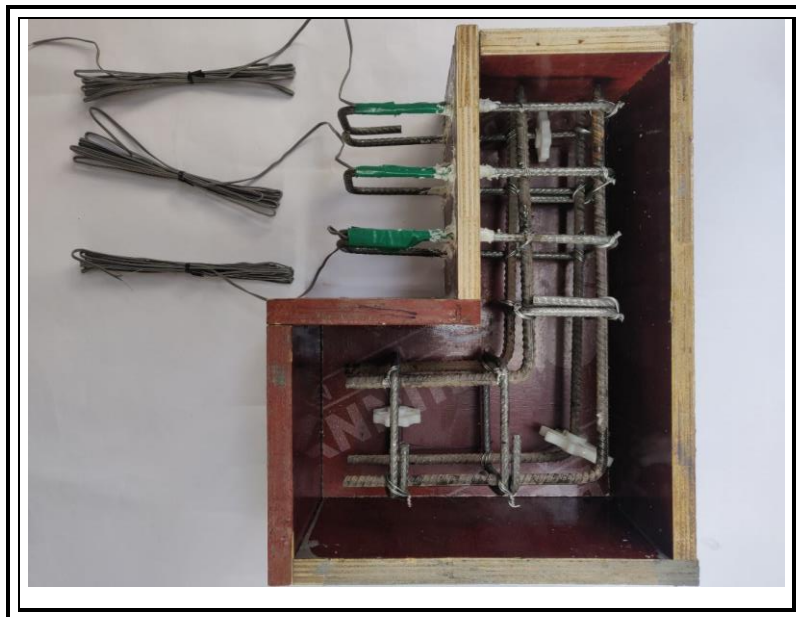
Figure 3- 6. Plywood form work.
