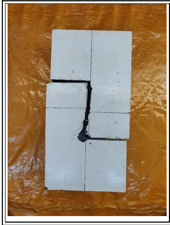
Figure 4- 3. Failure mode for CS.
