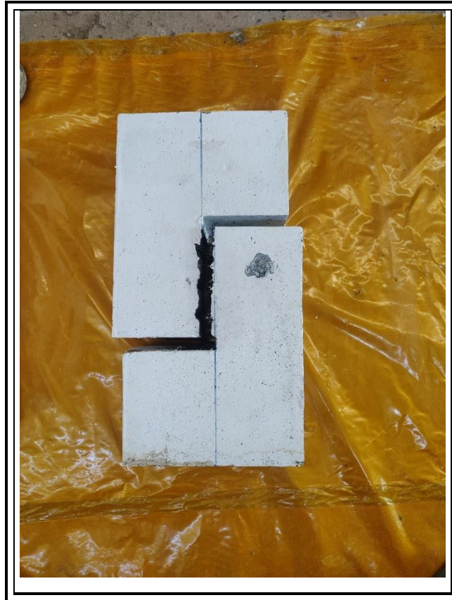
Figure 4- 7. Failure mode CG specimen.
