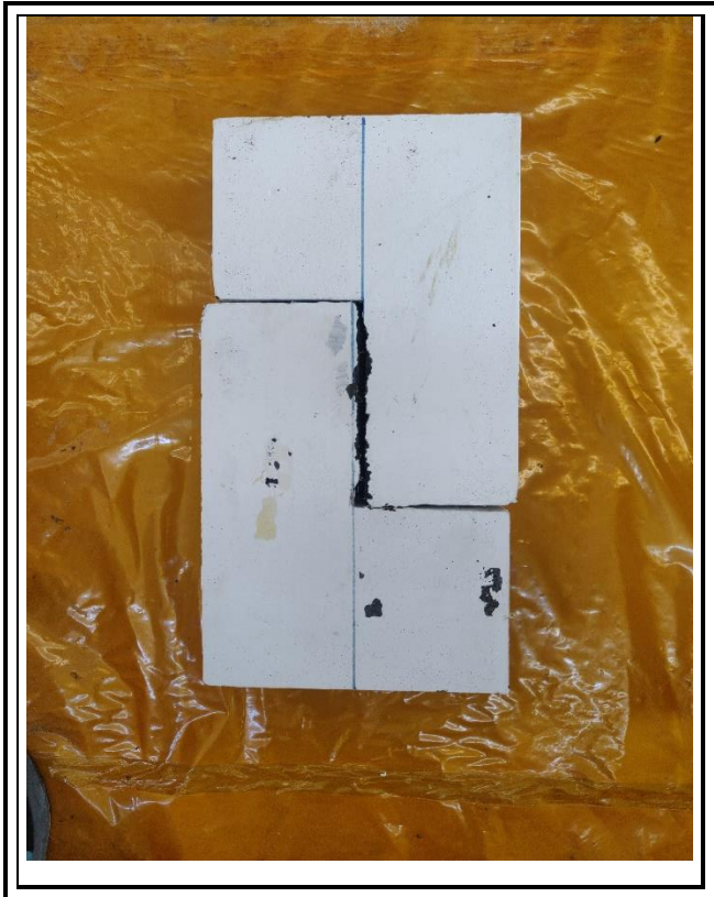
Figure 4- 17.Failure mode for EXF specimen.
