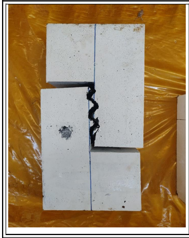
Figure 4- 11.Failure mode TRG 35 specimen.
