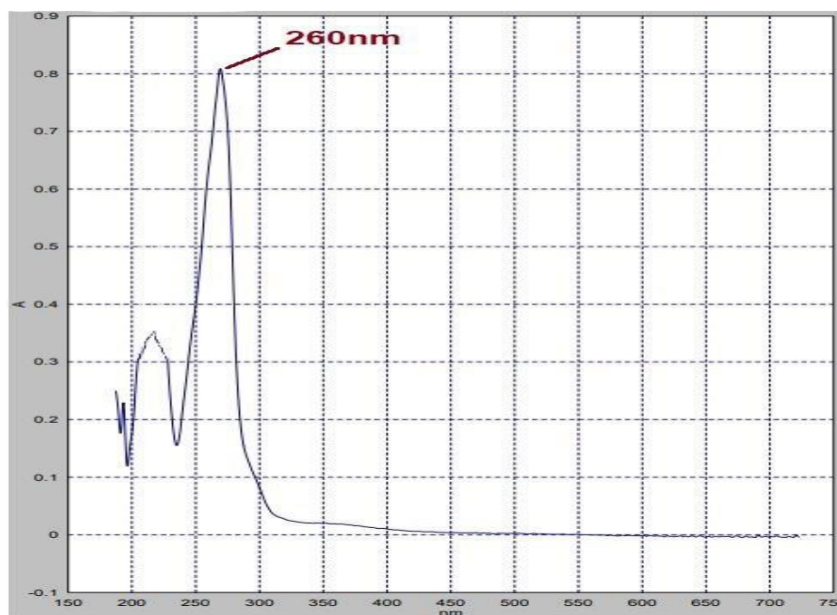
Figure 3.6: photo-spectrometry of extracted RNA by Nano drop , the trace represents the absorbance spectrum of one sample at 200-700 nm
