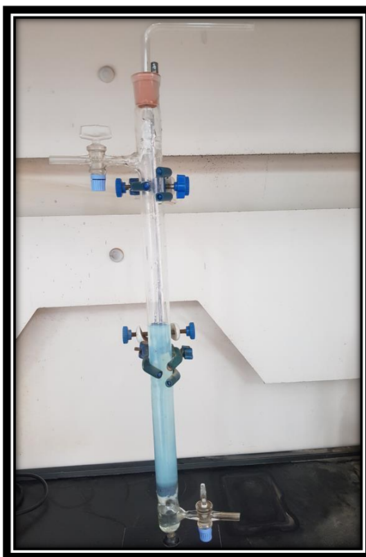
Picture (2.8): Separation column
