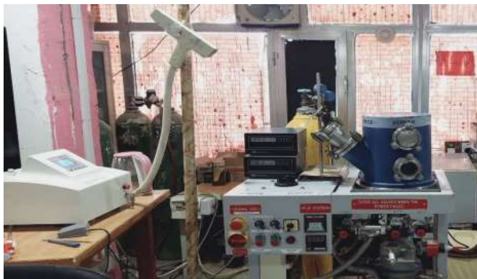
Figure (3.6): Pulsed laser deposition system.
