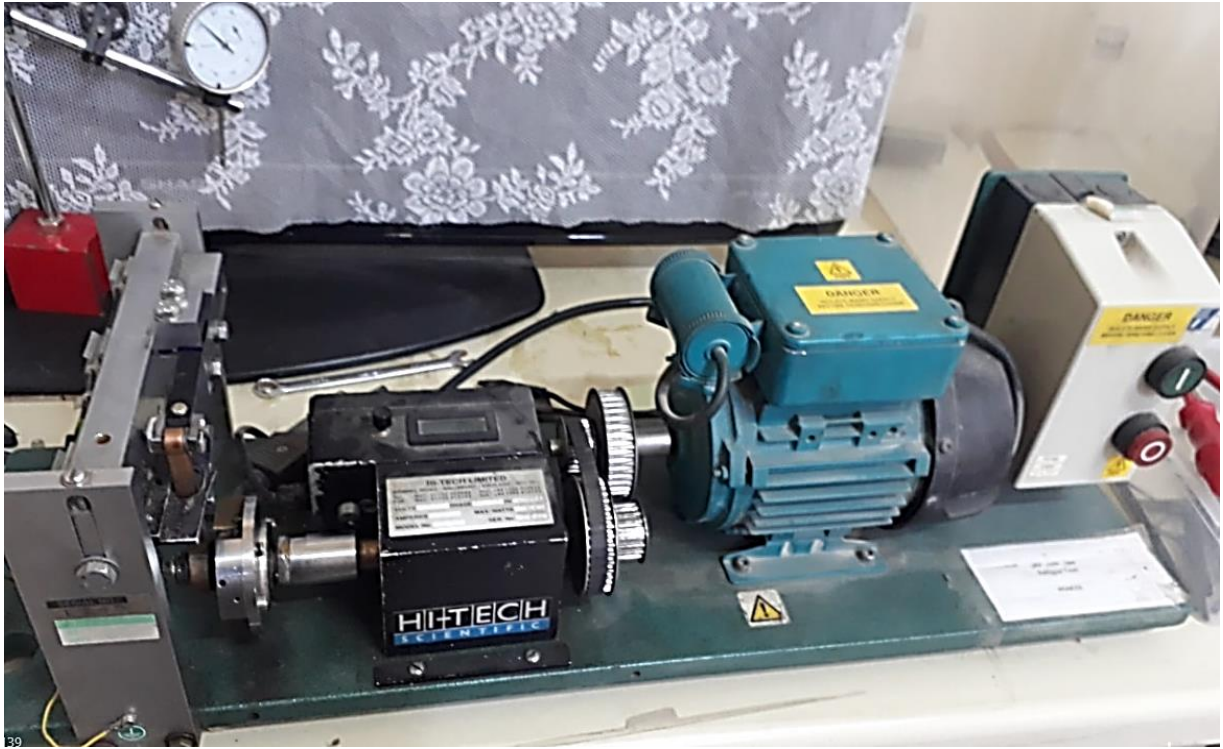
Figure 4.13 the testing machine (HSM20) of fatigue.
