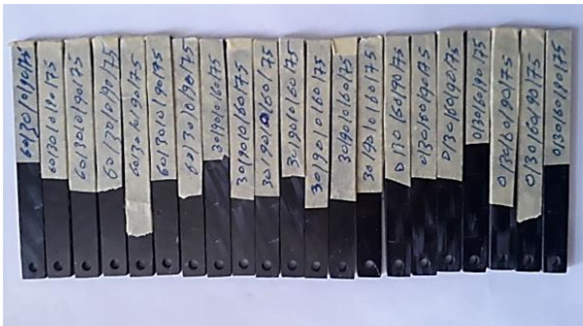
Figure 4.12 Sample dimensions of fatigue test.
