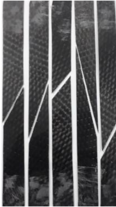
Figure 5.6 the fracture in the lamina (carbon/epoxy) with different fibers Orientation.
