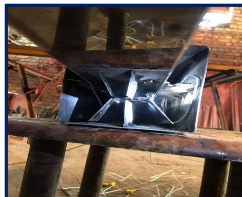
Figure 4.4: Channels manufacturing steps with installing the fins.
