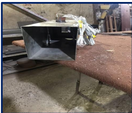
Figure 4.4: Channels manufacturing steps with installing the fins.
