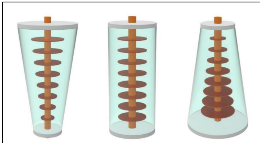
Figure 2.8: Latent heat thermal energy storage (LHTES) unit: (a) ascending conical; (b) cylinder; and(c) descending conical.
