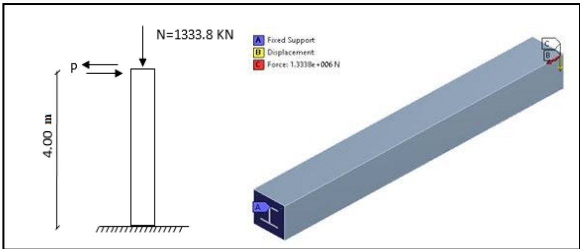
Figure 2-8 Composite Columns Boundary Conditions
