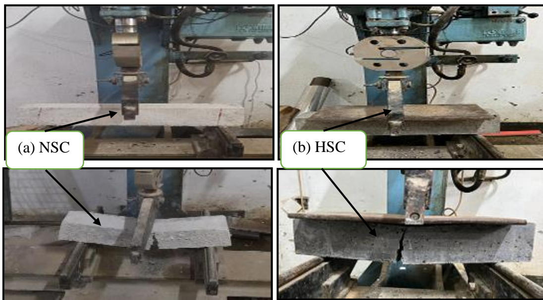
Plate 4-3 Failure Mode of Flexural Strength of Different Types of Concrete (a) NSC sampels (b) HSC sampels .
