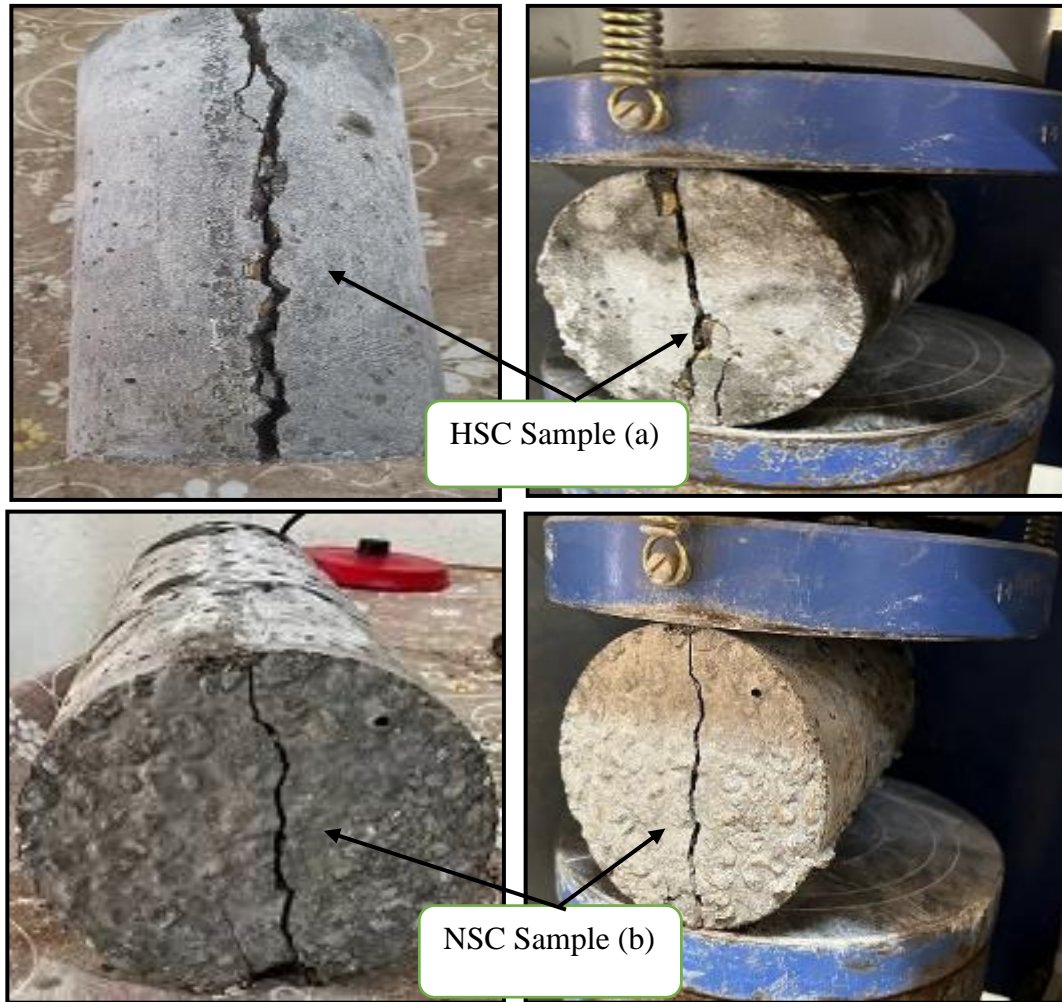
Plate 4-2 Failure Mode of Different Types of Concrete in Splitting Test (a) HSC (b) NSC
