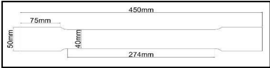
Figure 3-4 descriptions of dimension coupon as per ASTM-A370
