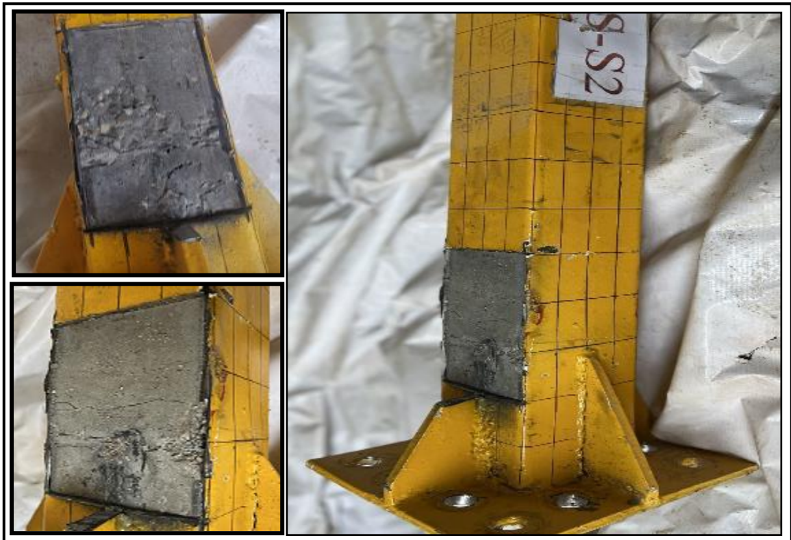
Plate 4-16 Cracks in Concrete after Failure
