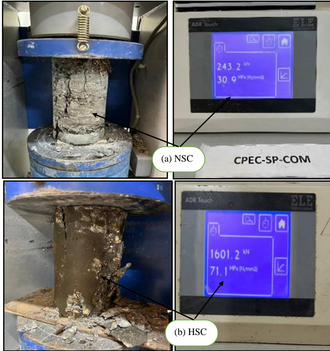
Plate 4-1 Failure Mode of Samples (a) NSC samples (b) HSC samples.
