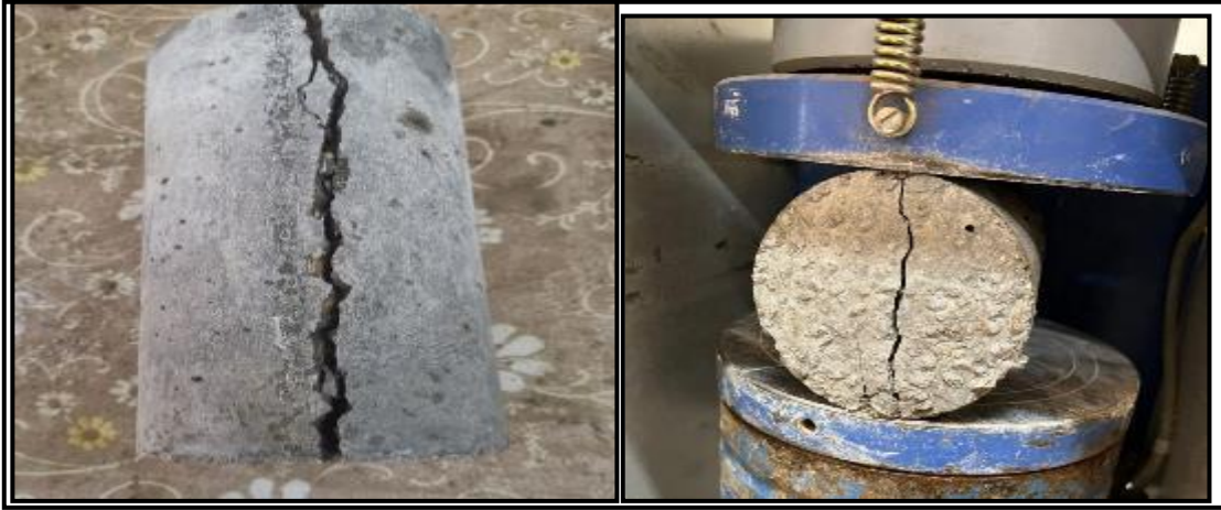
Plate 3-21 Splitting Tensile Test
