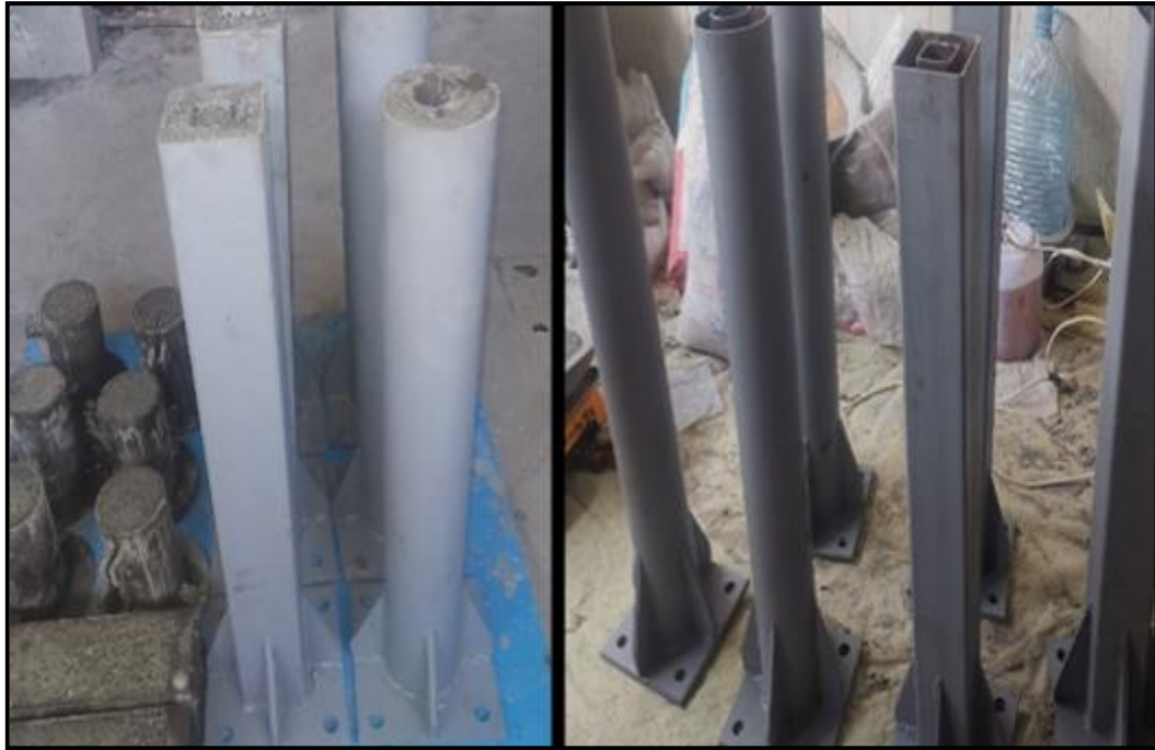
Plate 3-24 Preparing and Casting Specimens
