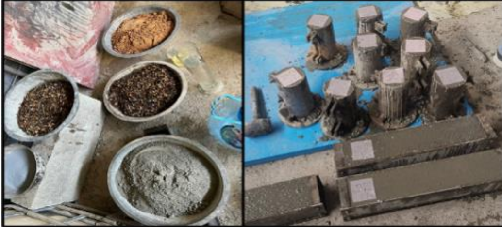
Plate 3-18 High Strength Concrete Mixture
