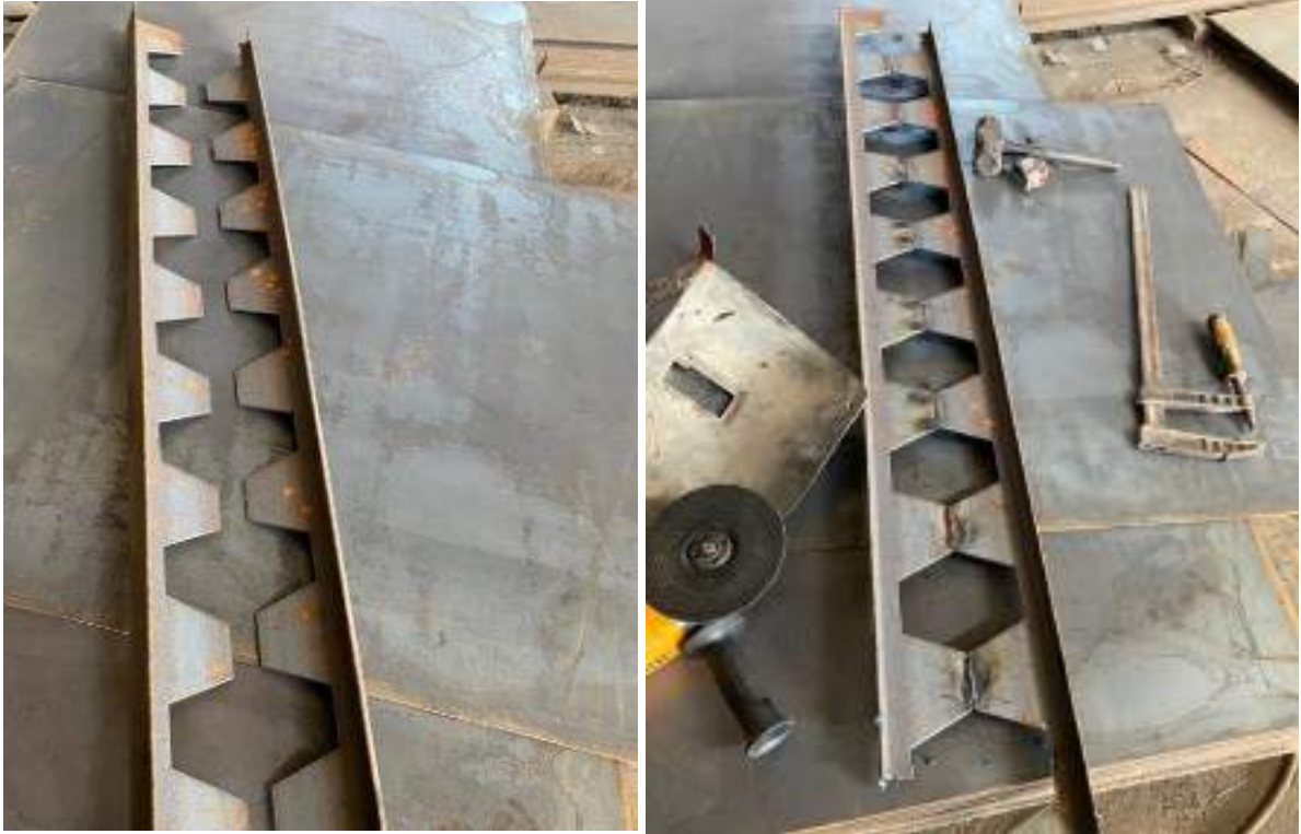
Plate 3-2: Assembling Technique of the Tee Sections.
