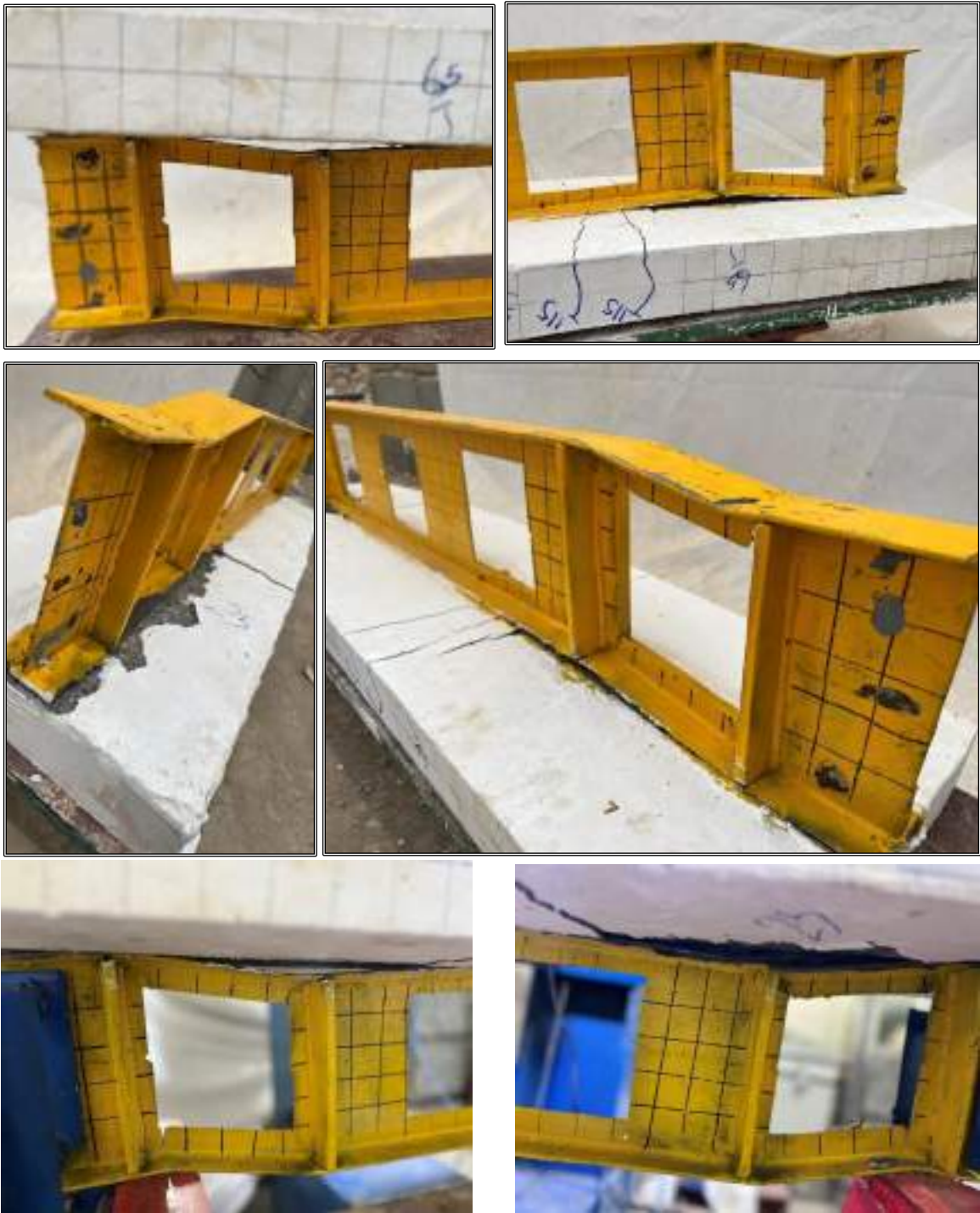
Plate 4-28: Beam CB-S9R2 at Failure.
