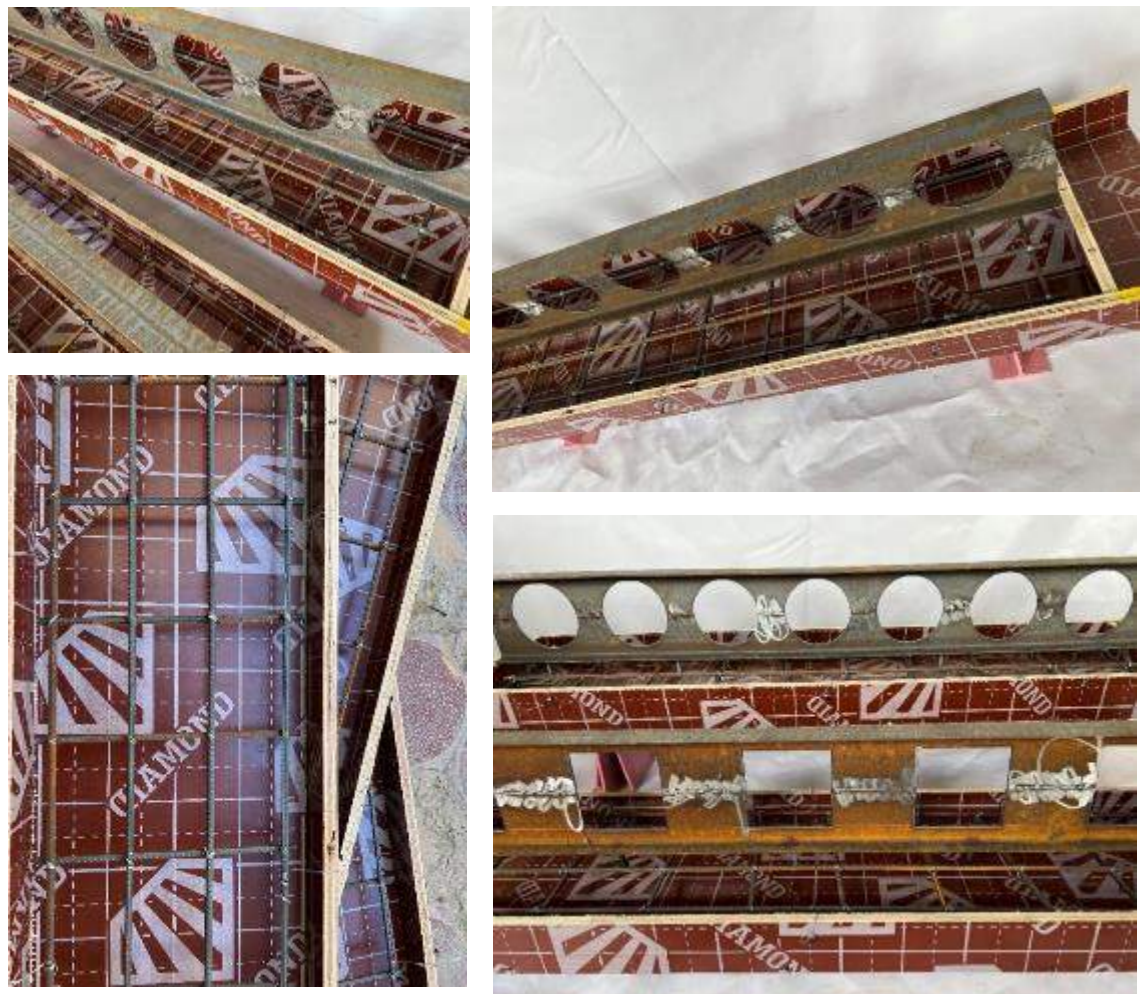
Plate 3-14: The Plywood Molds Used in Casting HSC Concrete Slab.
