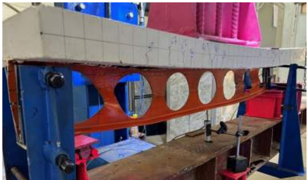
Plate 4-16: Beam CB-C4R1 at Failure.
