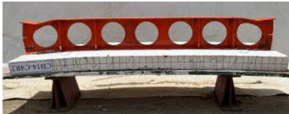
Plate 4-32: Beam CB-C4R2 at Failure.
