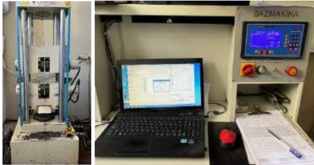
a- Mechanical Parts b- Digital Parts Plate 3-11: Tensile Steel Testing Machine.
