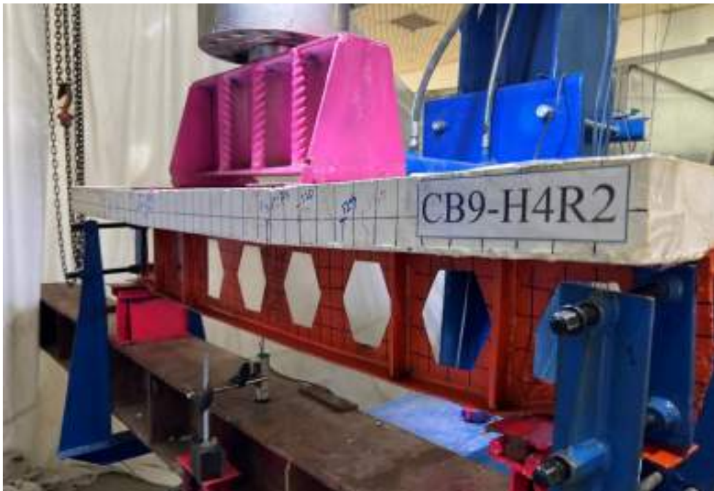
Plate 4-30: Beam CB-H4R2 at Failure.
