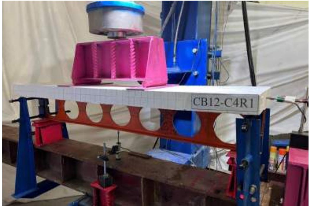
Plate 4-17 : Shape of Beam CB-C4R1 Before Testing.
