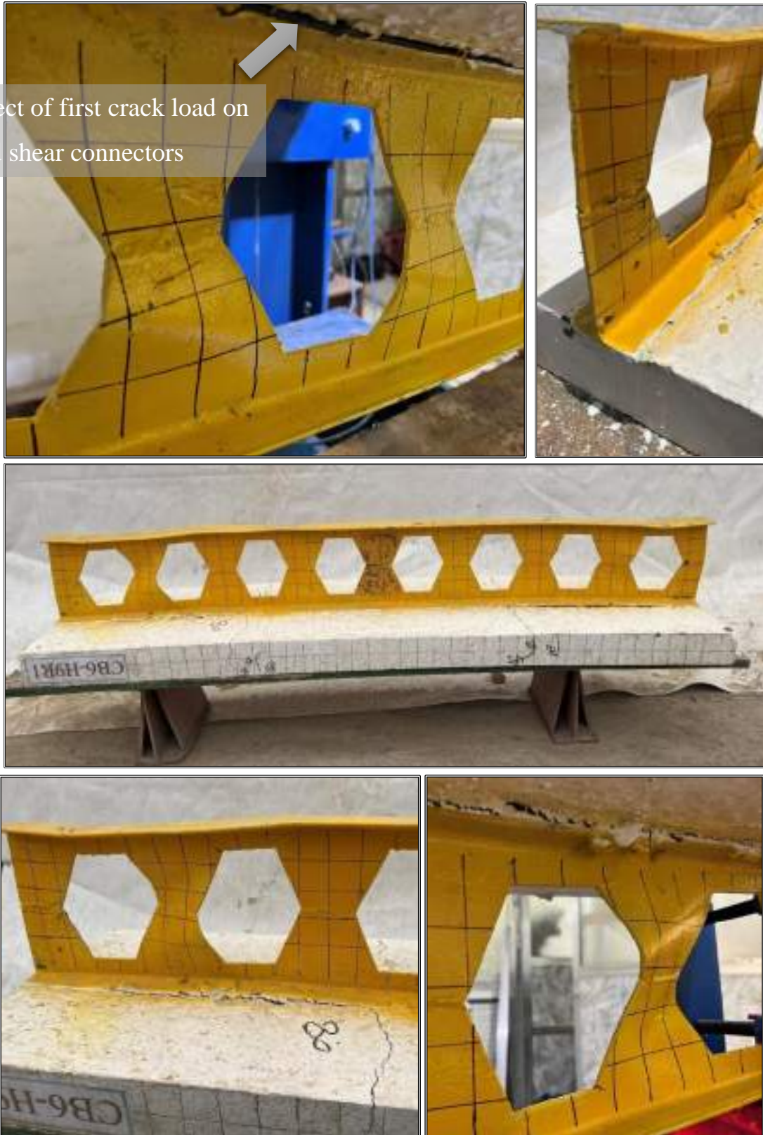
Plate 4-7: Failure of Beam CB-H9R1 After Testing (Web Post Buckling)
