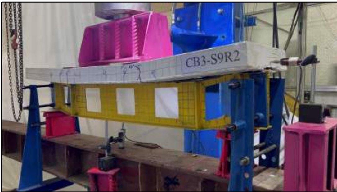
Plate 4-27: Beam CB-S9R2 at Failure.
