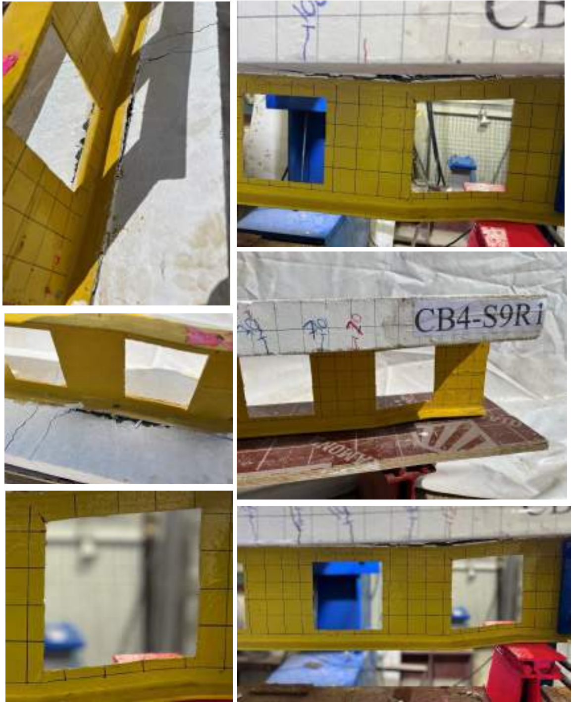
Plate 4-13: Failure of Beam CB-S9R1 After Testing (Buckling and yielding).
