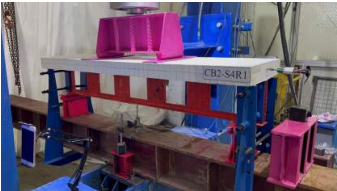
Plate 4-19: Beam CB-S4R1 at Failure.
