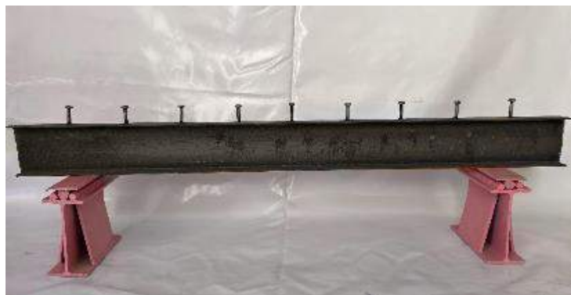
Plate 3-3: Distribution of Shear Connectors of CB-9S
