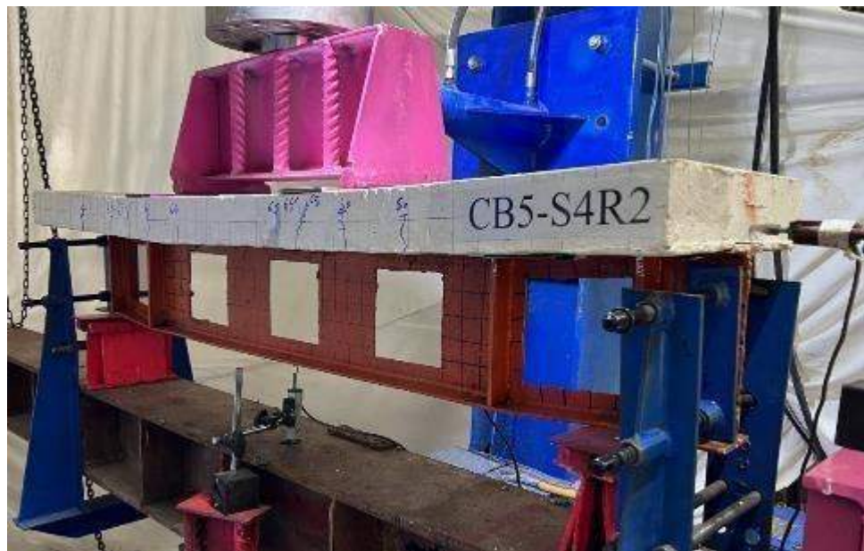
Plate 4-35: Beam CB-S4R2 at Failure.
