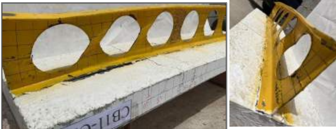
Plate 4-10: Effect of First Crack Load on Stud Shear Connectors.
