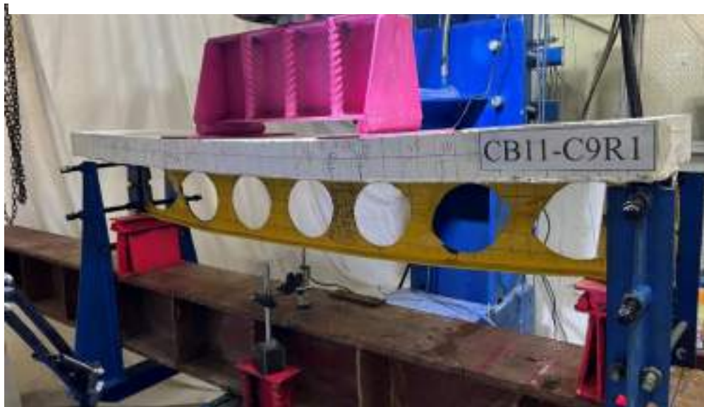
Plate 4-9: Beam CB-C9R1 at Failure.
