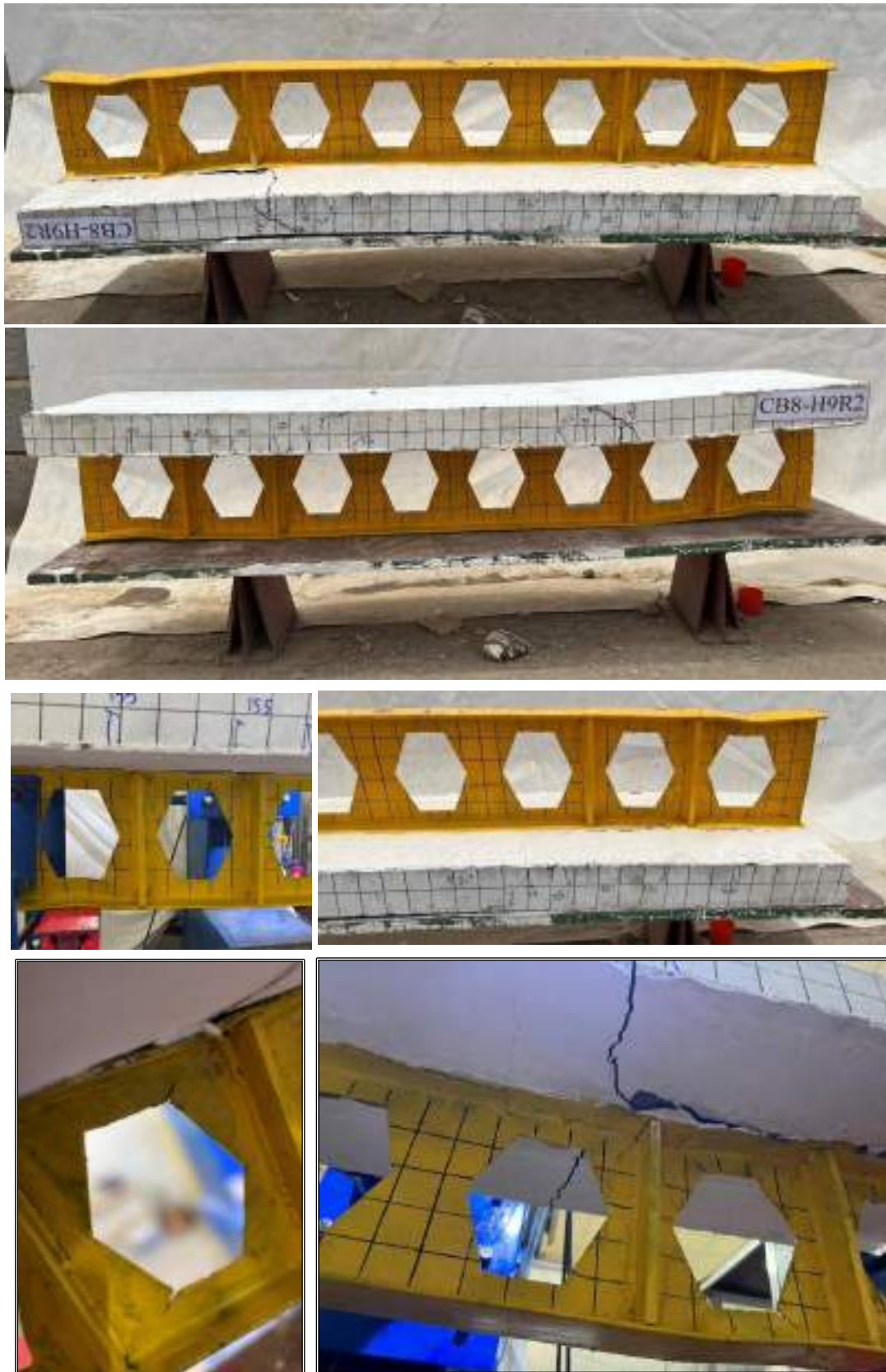
Plate 4-23: Beam CB-H9R2 at Failure.
