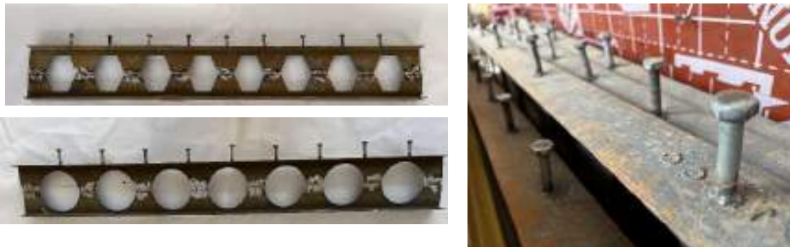
Plate 3-13: Illustration depicting stud shear connectors.
