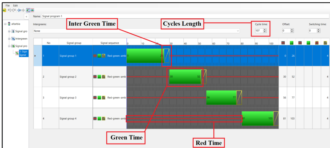
Figure 3-27 Screenshots Illustrating Fourth Stages Modeling Traffic Signal Timing (Insert The Cycles Length Time and Make Connection Between All Approach)
