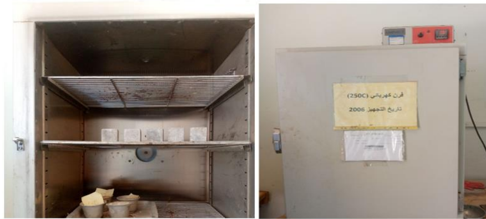
Figure 3-12:Oven drying of hardened density of grout specimen
