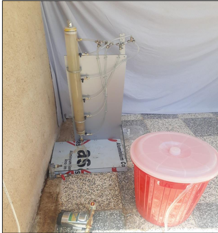
Figure 3.4 Column experiment system
