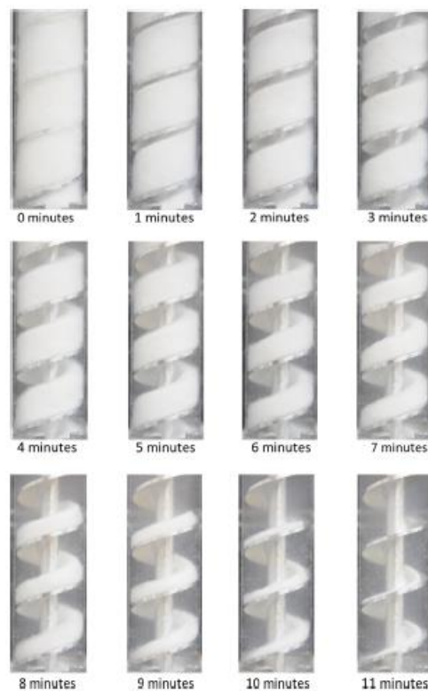
Fig. (2.13). The process of melting (charging) in a helical-fin laboratory prototype
