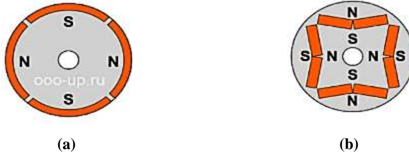
Fig.2.4: PMSM Types (a) SPMSM, (b) IPMSM [28].
