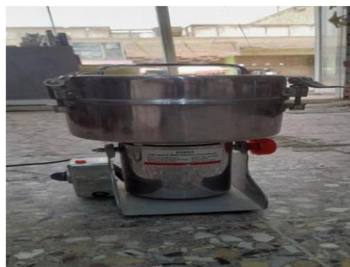
**Figure 3.4** Electronic mill
