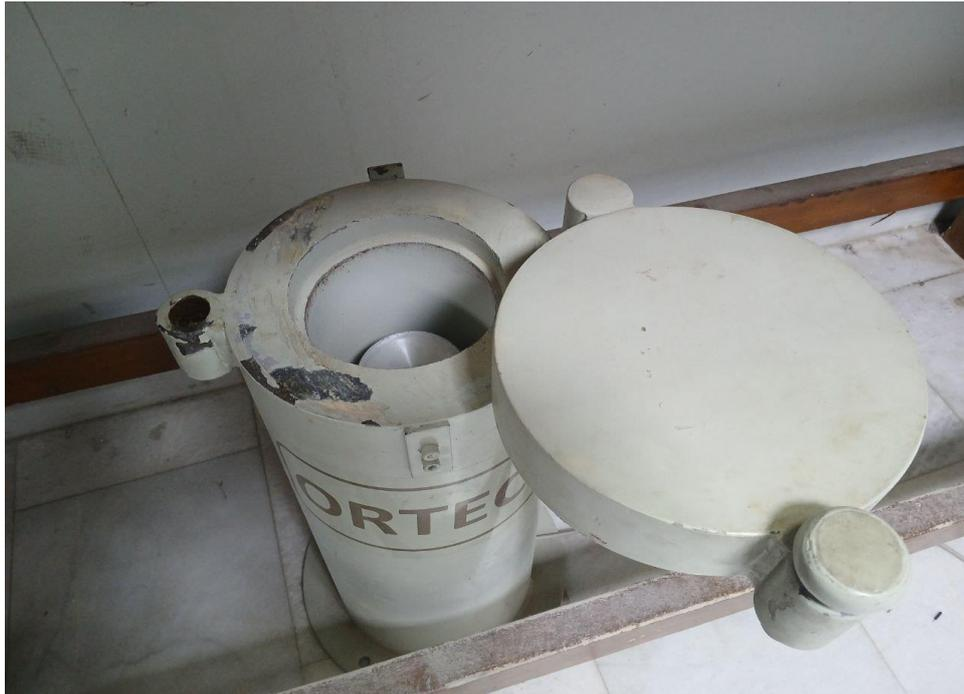
**Figure 2.8** Shield chamber and detector location inside the shield.
