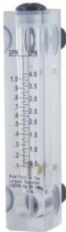
Figure (4-6): Flow meter image.
