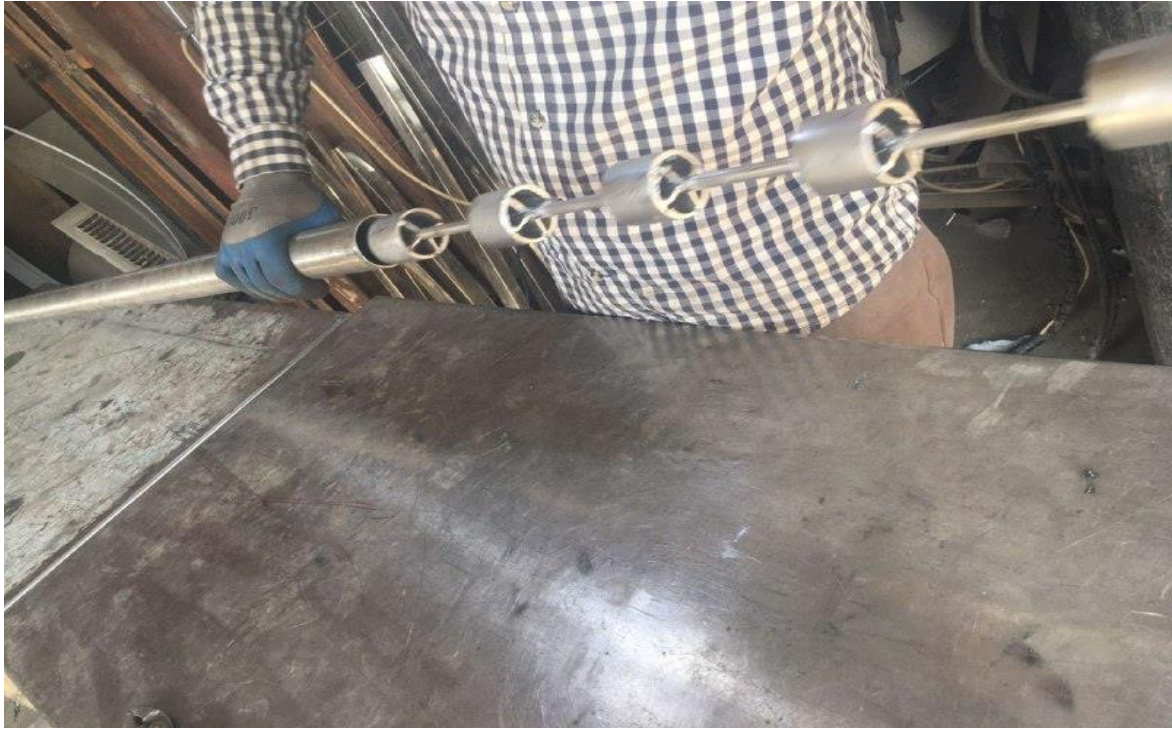
Figure (4-4): Cylindrical turbulators inside the PTR.
