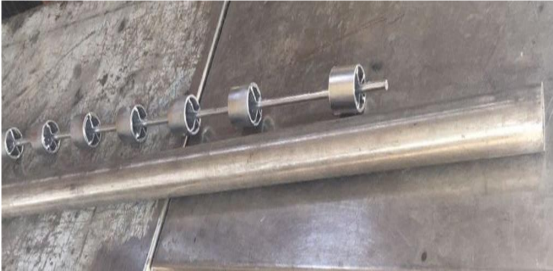
Figure (4-3): Photograph of the PTR and cylindrical turbulators.
