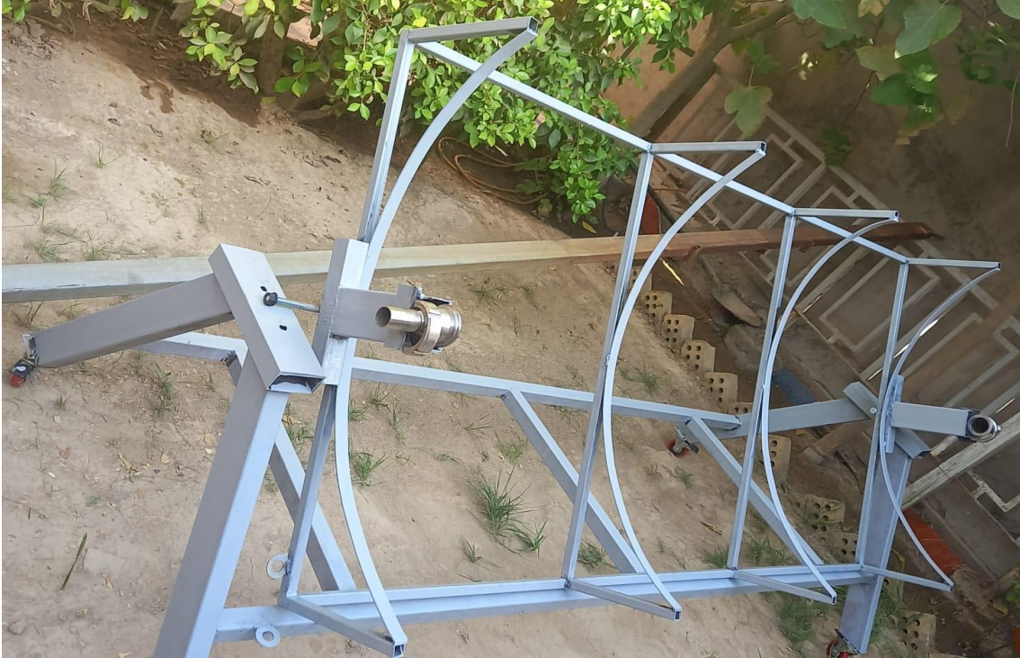
Figure (4-1): The support structure of the PTC.
