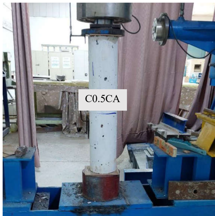
Corroded concrete column containing glass powder (G8)
