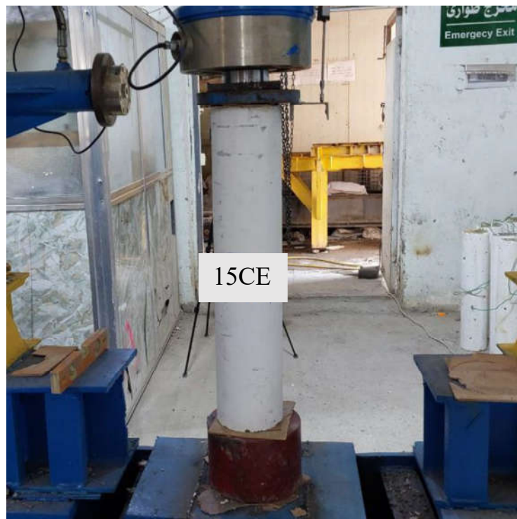
Non-corroded concrete column containing ceramic powder (G1)
