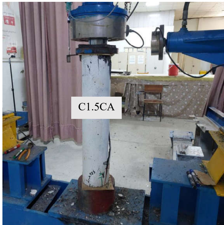
Corroded concrete column containing carbon black (G9)
