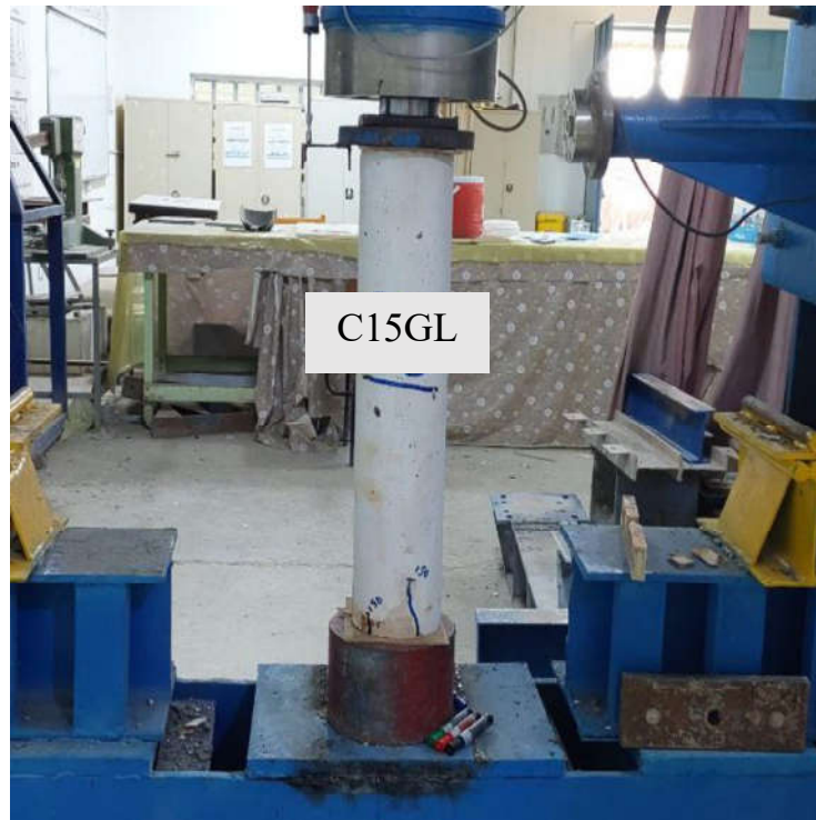
Corroded concrete column containing glass powder (G8)
