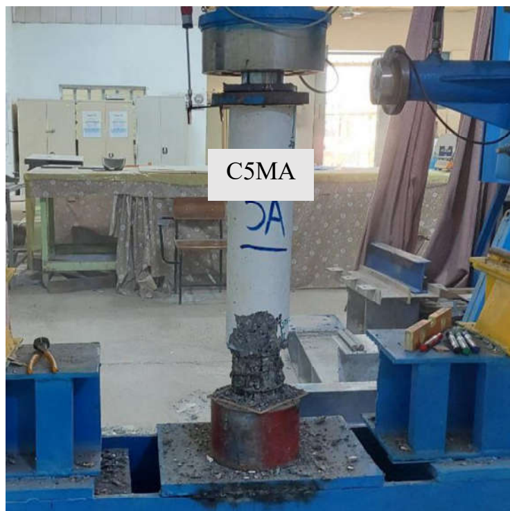
Corroded concrete column containing ceramic powder (G6)
