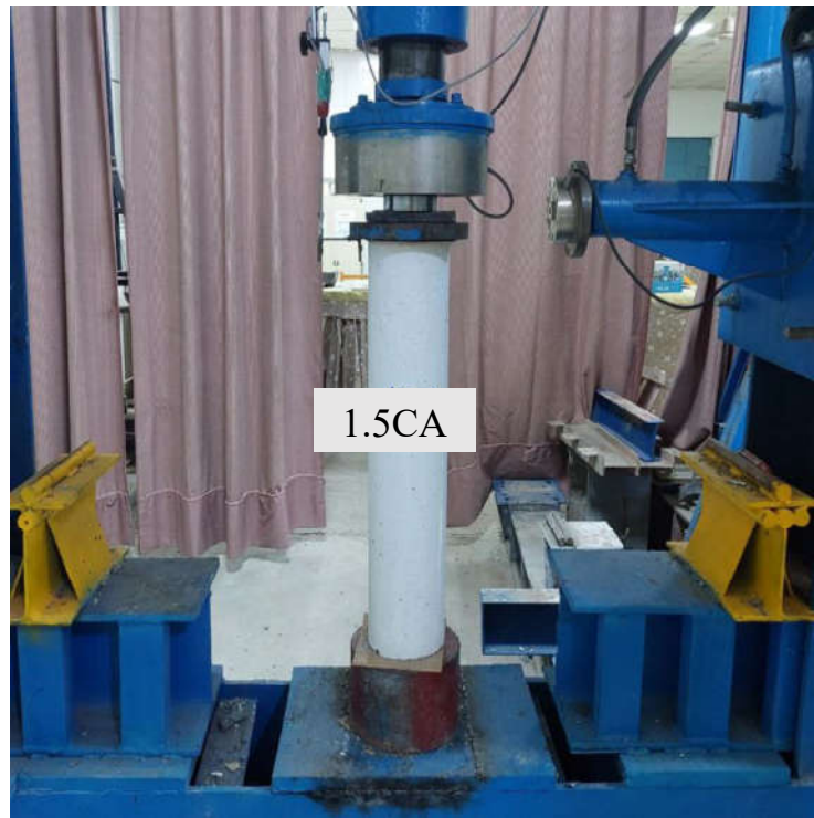
Non-corroded concrete column containing carbon black (G4)
