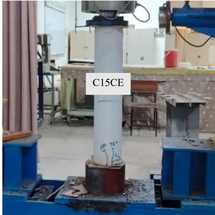
Corroded concrete column containing ceramic powder (G6)
