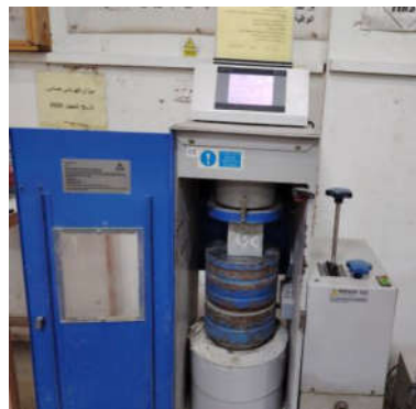
Figure 3-14. Compressive strength test.
