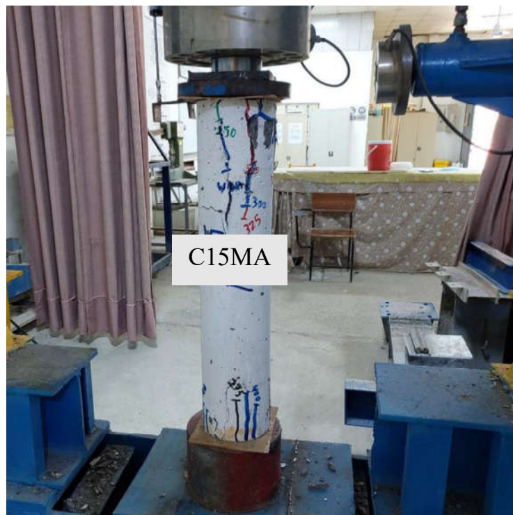
Corroded concrete column containing marble powder (G7)
