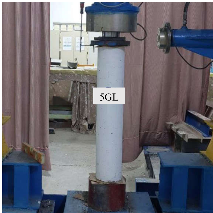
Non-corroded concrete column containing marble powder (G2)
