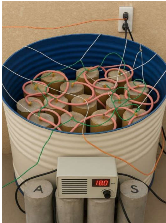
Figure 3-21. The mechanism of accelerating corrosion using electric current for the studied columns.
