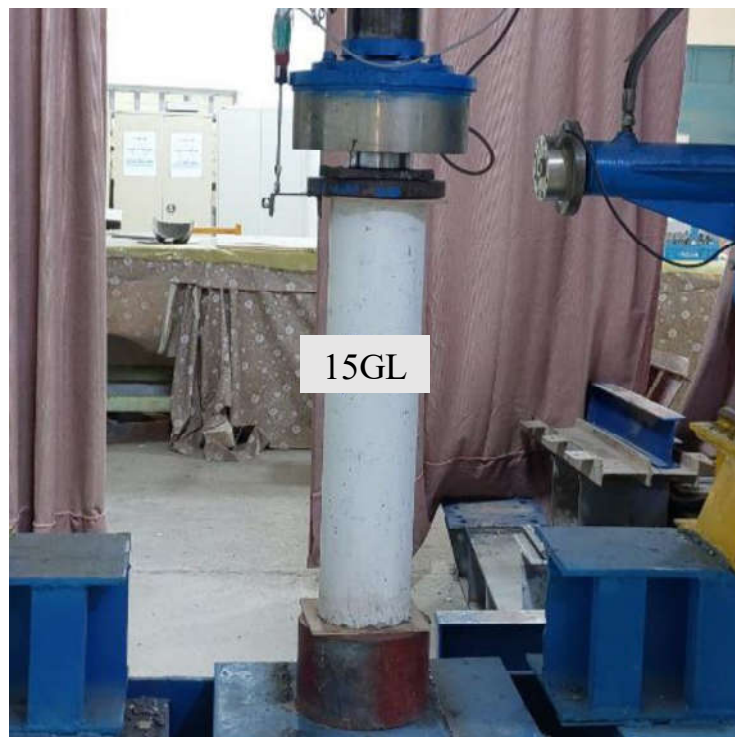
Non-corroded concrete column containing glass powder (G3)
