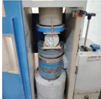
Figure 3-15. Splitting tensile strength test.
