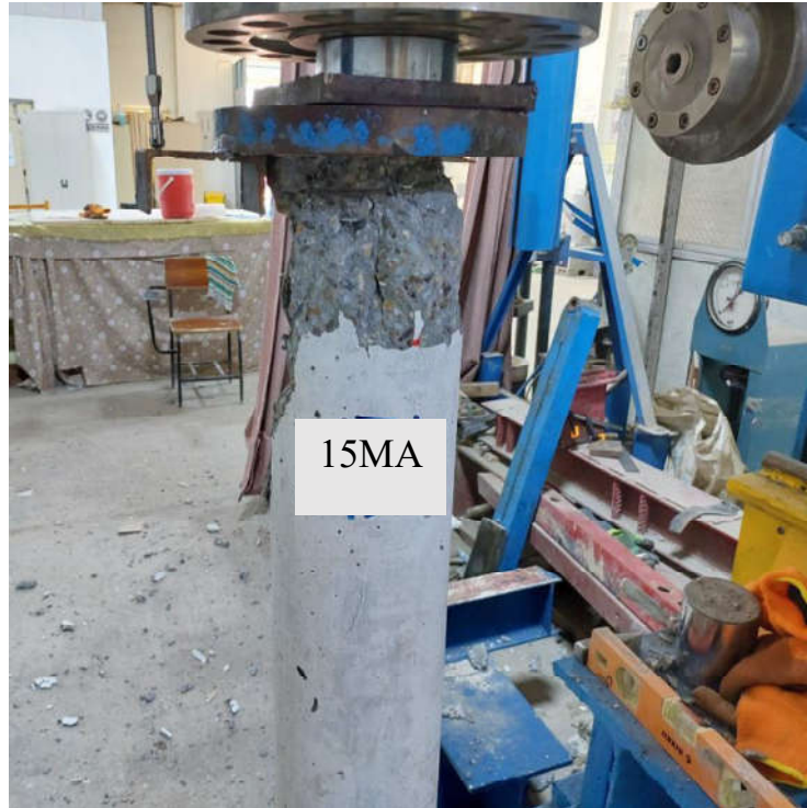
Non-corroded concrete column containing marble powder (G2)
