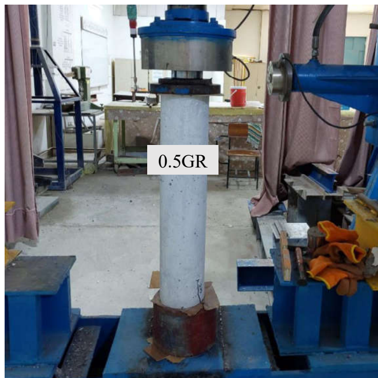
Non-corroded concrete column containing carbon black (G4)
