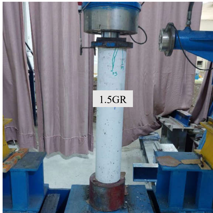
Non-corroded concrete column containing graphite powder (G5)
