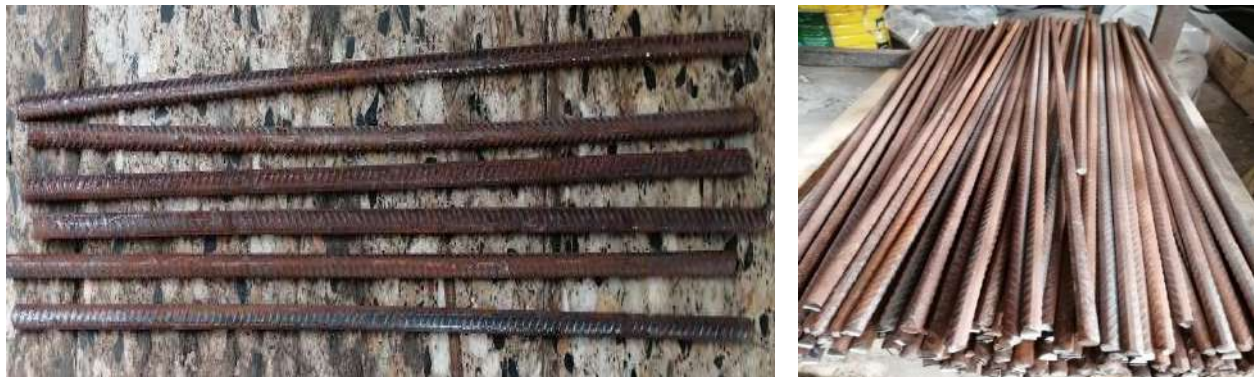
Figure (3.8): Steel Bar Reinforcement.
