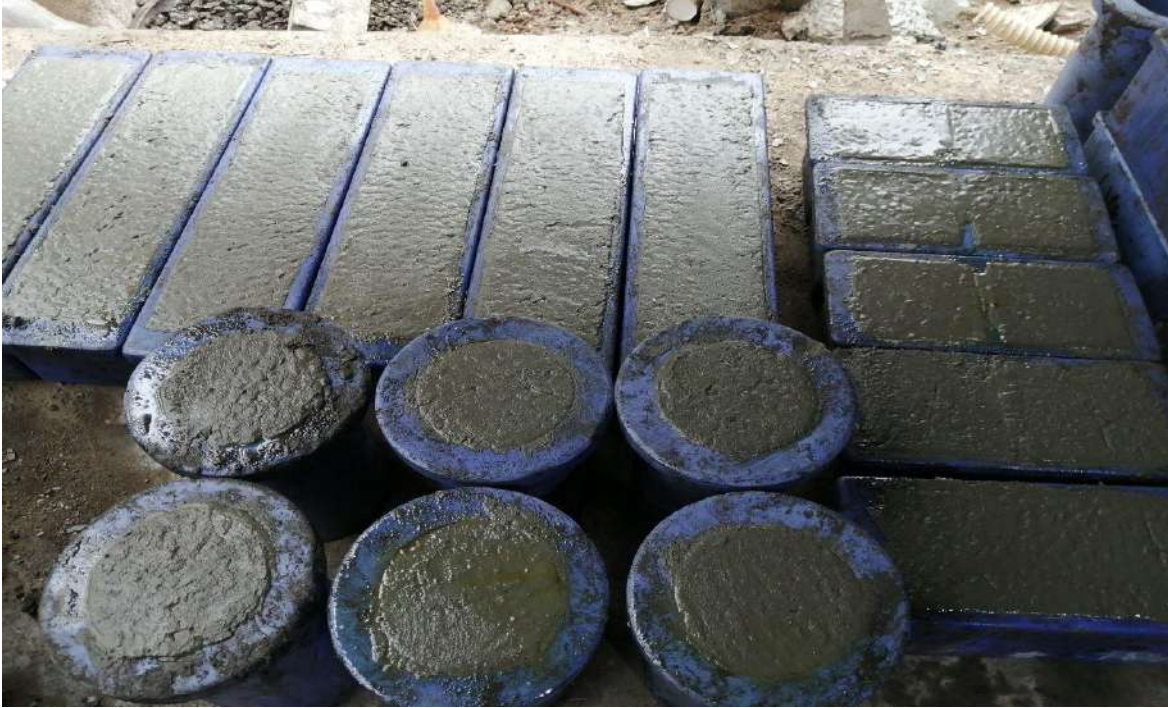
Figure (3.18): Casting of the cube, cylinder, and prism for concrete tests.
