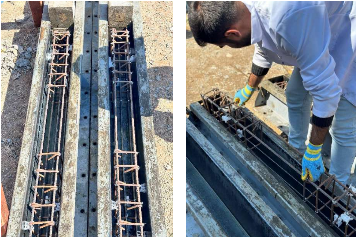
Figure (3.14): Beam specimens, steel moulds, and reinforcement bars.
