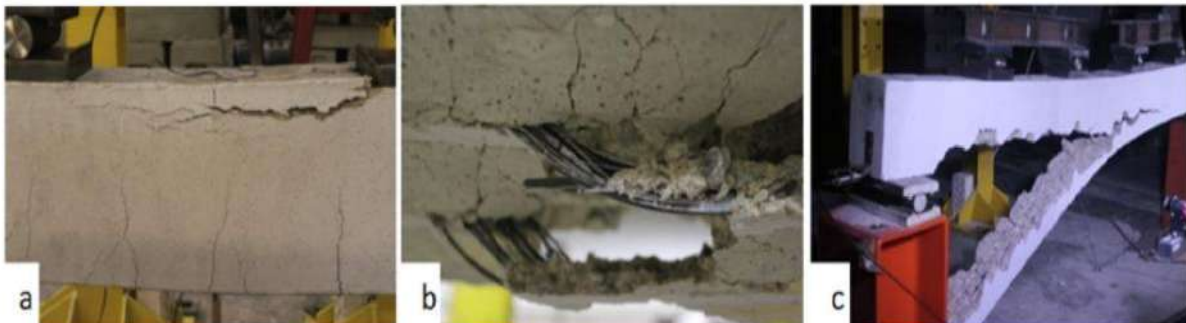
Figure (2.14): Failure modes: (a) Concrete crushing, (b) NSM CFRP rupture, (c) Concrete cover separation (Barris et al., 2020).
