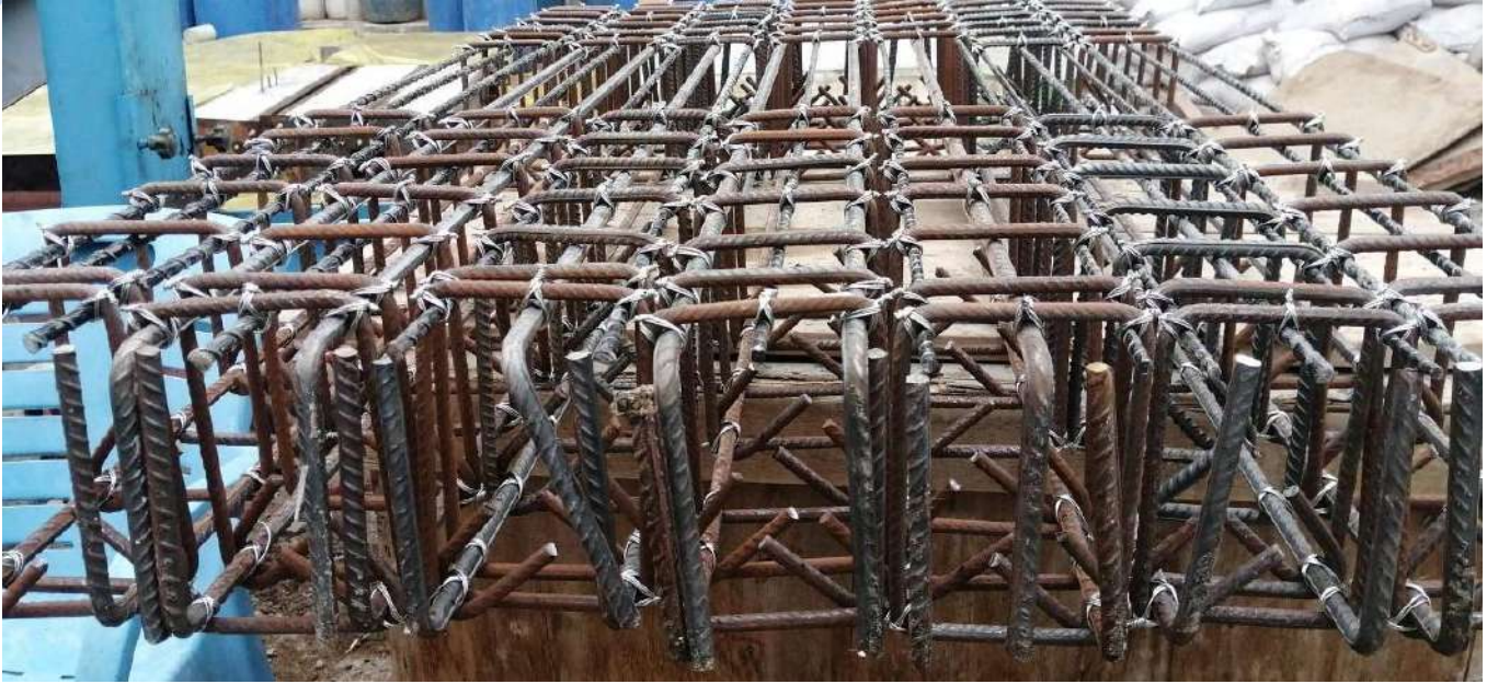
Figure (3.6): Detail of hybrid reinforcement of specimens.
