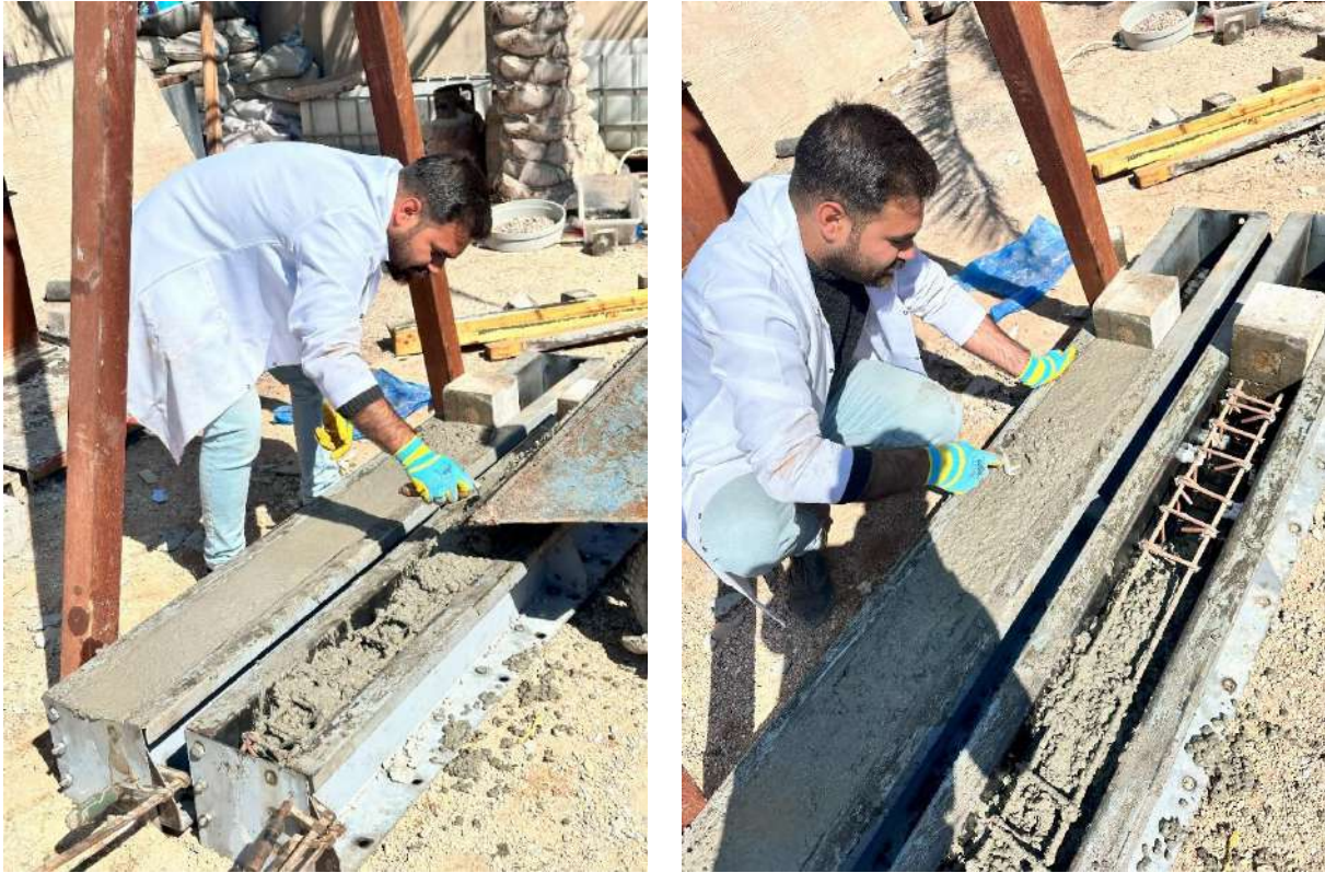
Figure (3.16): Casting the Specimens.
