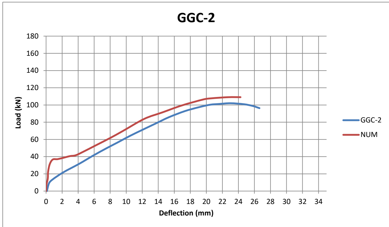
Figure (5.26): Numerical and experimental load-deflection curves for (GGC-2) model.
