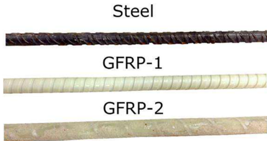
Figure (2.13): Bar types used for internal reinforcement (Barris et al., 2020)
