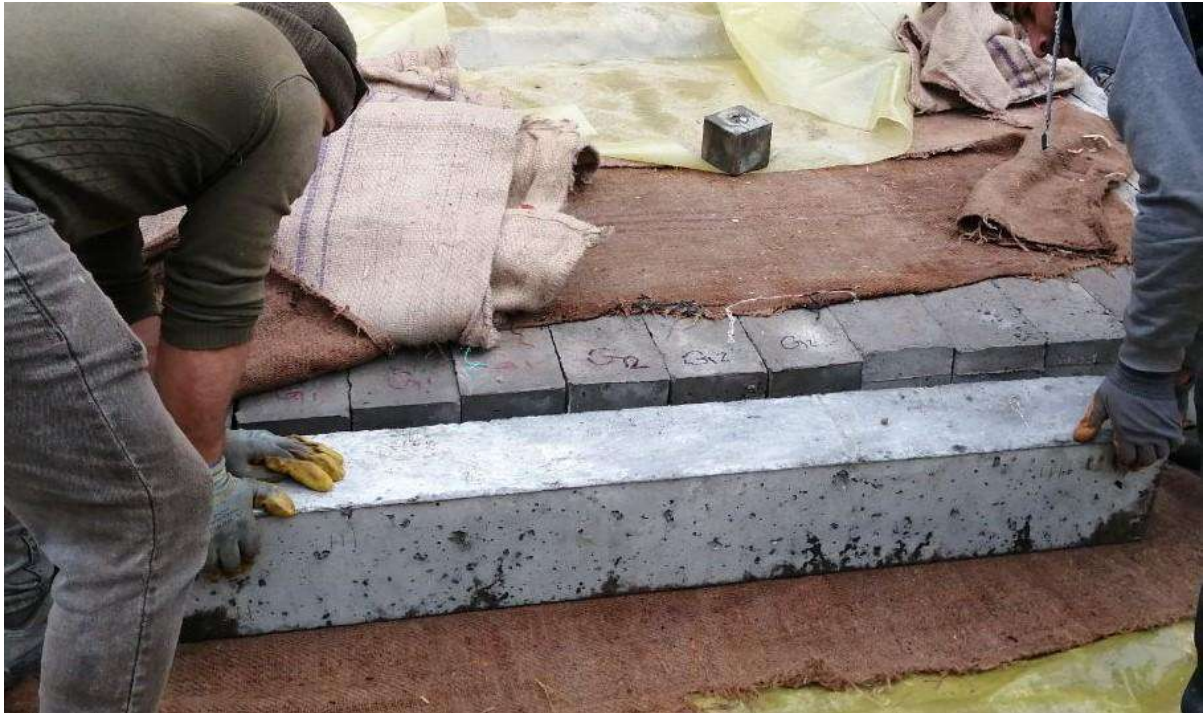
Figure (3.19): Curing of the specimens.
