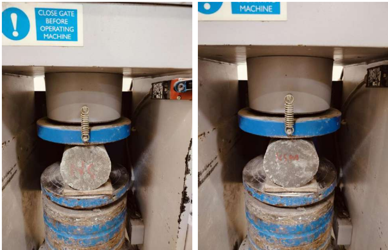
Figure (3.22): Splitting Tensile Strength Test.
