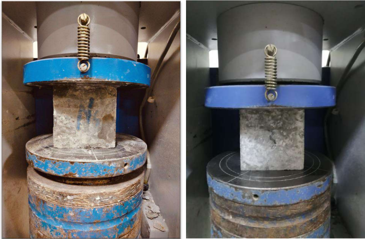
Figure (3.21): Compressive strength tests of Cube.
