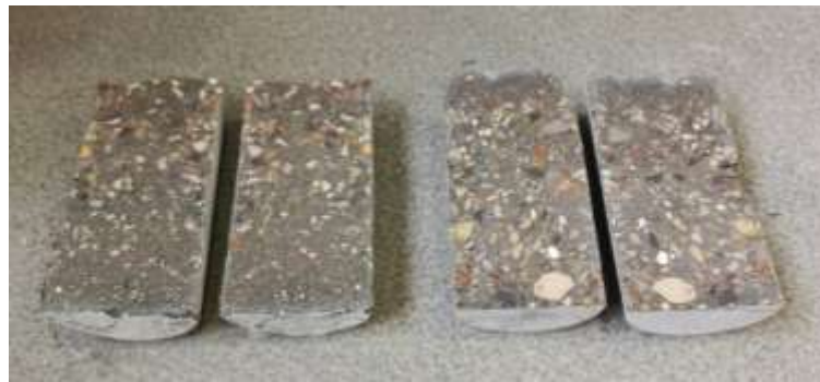
Plate 4-1: Failure patterns due to the splitting tensile strength test .
