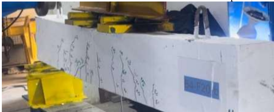
Plate 4-6: Failure mode for B4-F20-b under repeated load
