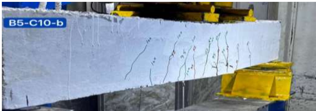
Plate 4-7: Failure mode for B5-C10-b under repeated load
