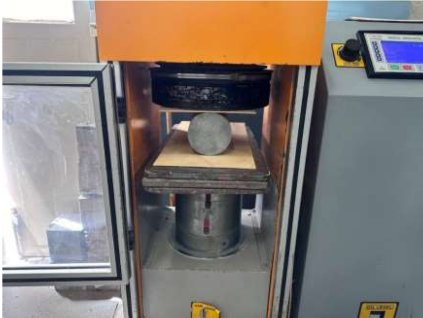
Plate 3-13: Tensile strength splitting test
