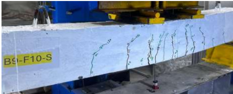
Plate 4-11: Failure mode for B9-F10-S under repeated load.
