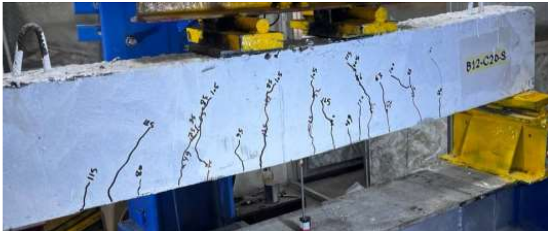
Plate 4-14: Failure mode for B12-C20-S under repeated load
