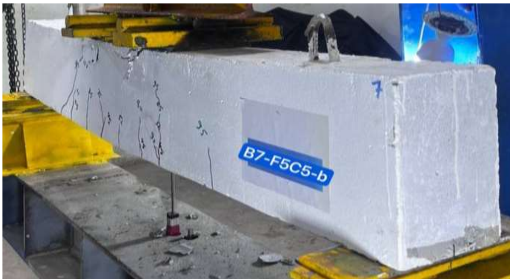
Plate 4-9: Failure mode for B7-F5C5-b under repeated load
