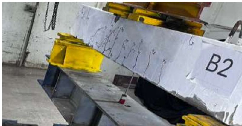
Plate 4-4: Failure mode for B2 under repeated load
