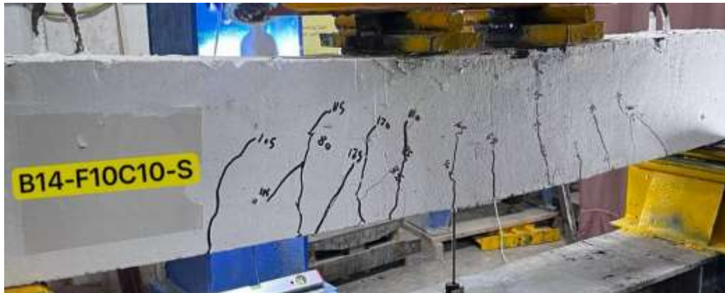
Plate 4-16: Failure mode for B14-F10C10-S under repeated load
