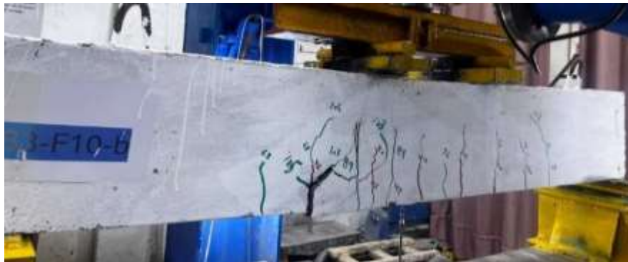
Plate 4-5: Failure mode for B3-F10-b under repeated load
