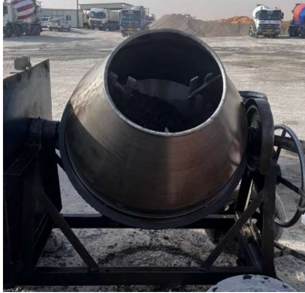
Plate 3-7: Laboratory concrete mixer.
