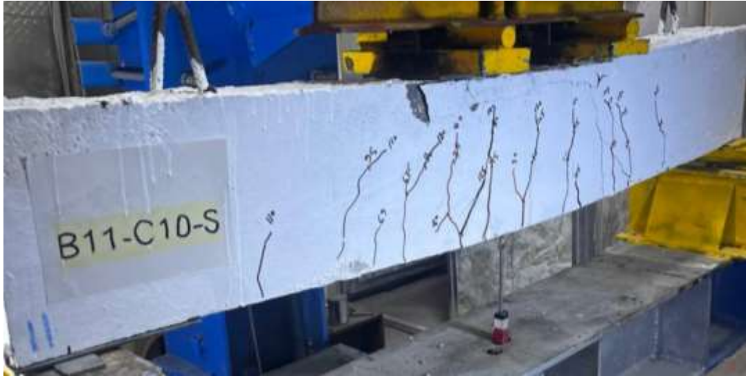
Plate 4-13: Failure mode for B11-C10-S under repeated load
