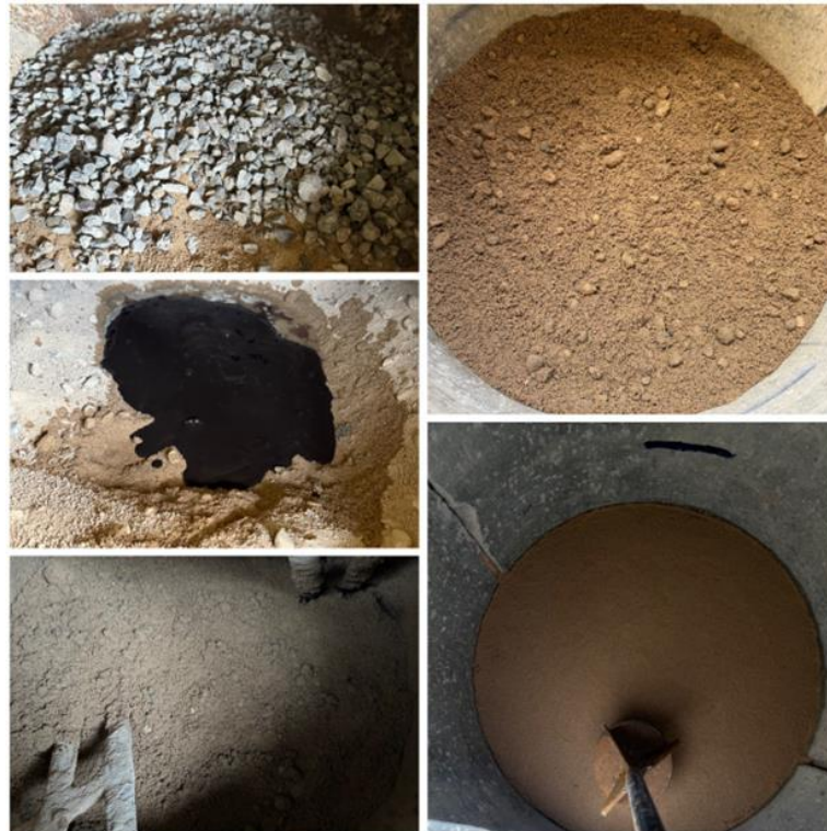
Figure (3-8): Steps to Prepare a Sample of Soil.
