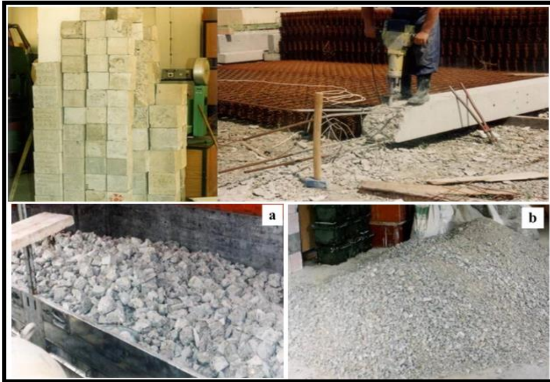
Figure (2-4): RCA material after (a) primary and (b) secondary crushing(Radonjanin, 2010).
