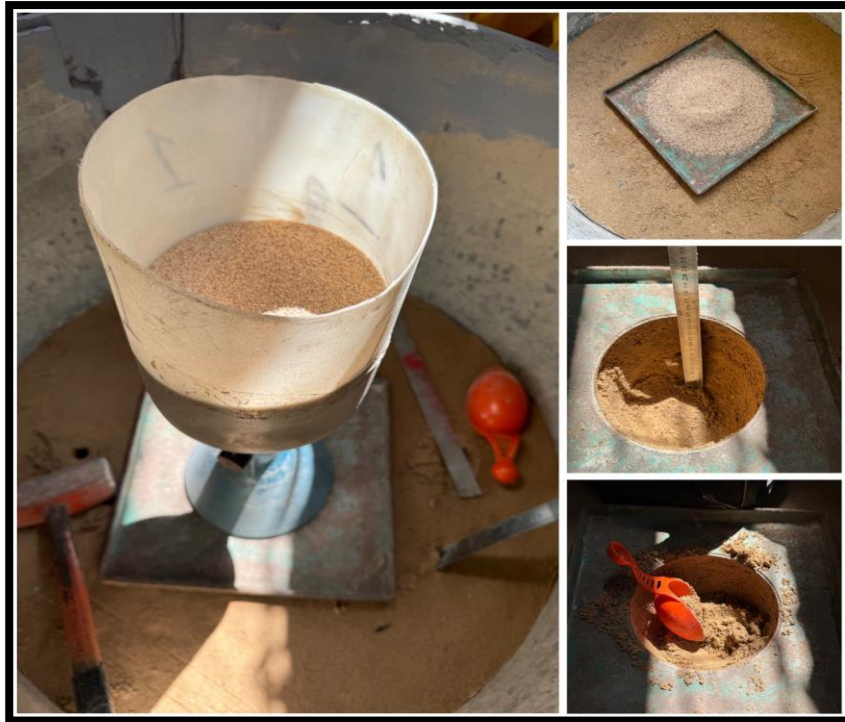
Figure (3-11): Sand Replacement Test.
