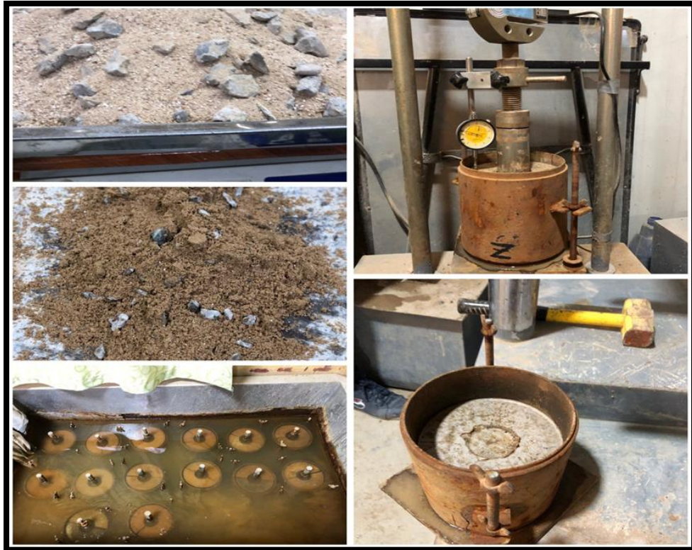
Figure (3-7): Preparation of Test Specimens of the Treated Soil Mixtures for CBR Test.
