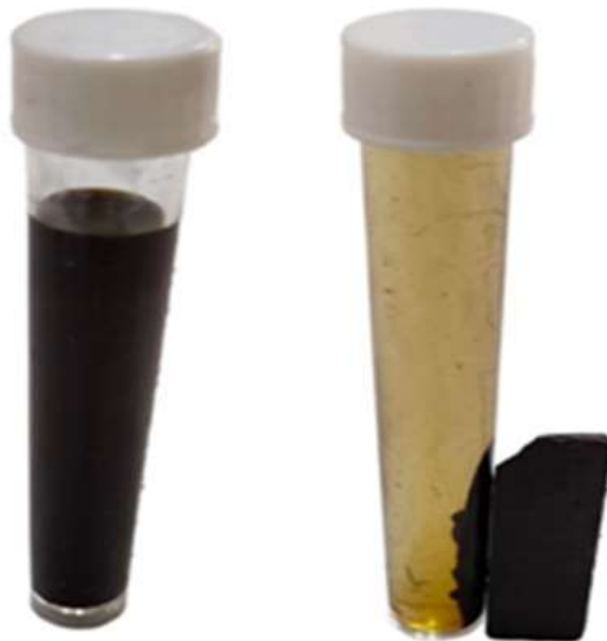
Figure (2.11): Photograph of a magnet attracting of Fe 3 O 4 in water
