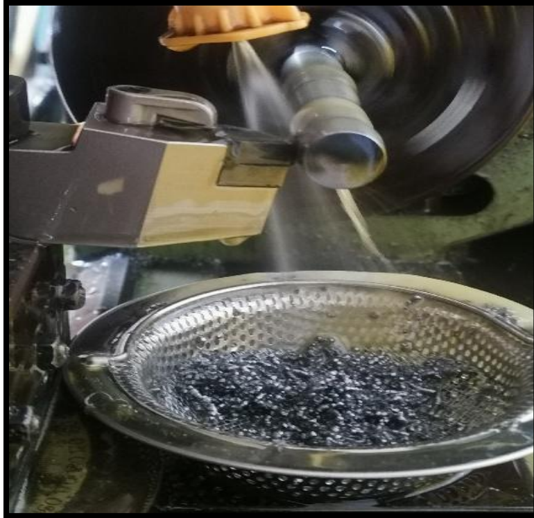
Figure 4.19: The Oil jet lubrication with angle 15°.
