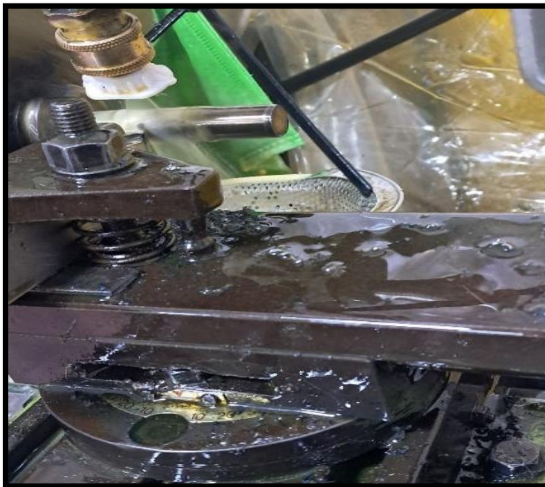
Figure 4.19: The Oil jet lubrication with angle 15°.
