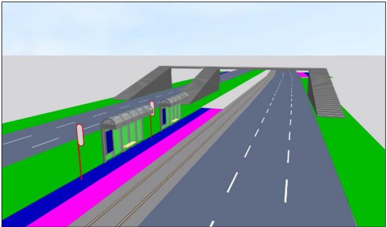
Figure (6.15.a): Simulated tram stops and isolated lane alignment at central median.
